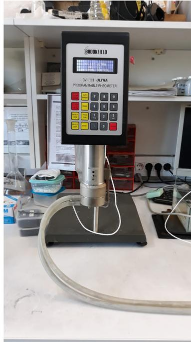
Figure 2.3. Viscosity measuring device
