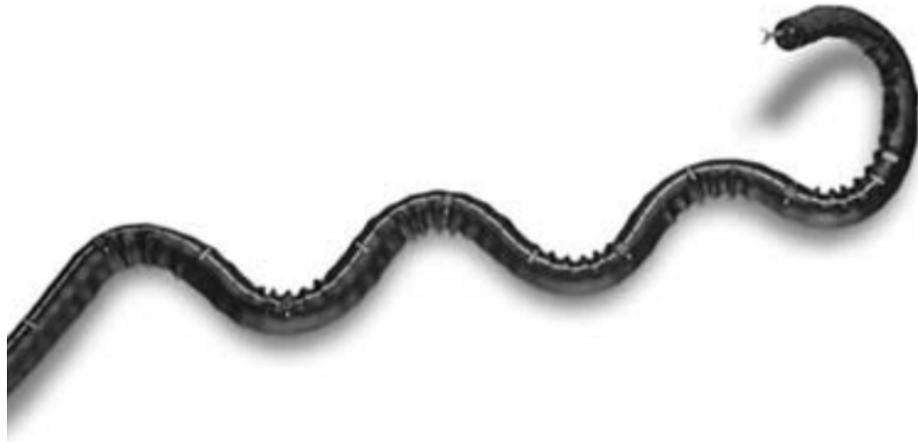
Figure 2.8. Independently actuated segments of the NeoGuide Endoscopic System through its colonoscope shaft. Reprinted from [66].
