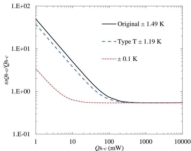
Figure 5.9. Effect of temperature measurement uncertainty on  $\omega_{Q_{h-c}}/Q_{h-c}$ .
