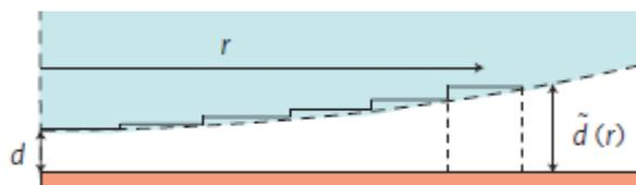
Figure 2.15 Visualization of Derganjuin Approximation (Rousseau *et al.*, 2009)
