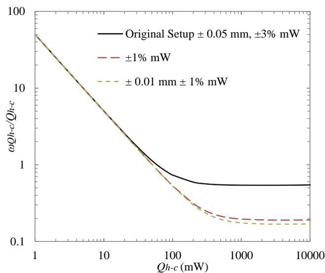
Figure 5.10. Effect of dimensional accuracy and flux measurement accuracy on  $\omega_{Q_{h-c}}/Q_{h-c}$ .
