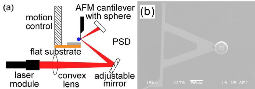
Figure 2.11. Experimental Setup (Narayanaswamy *et al.*, 2008).
