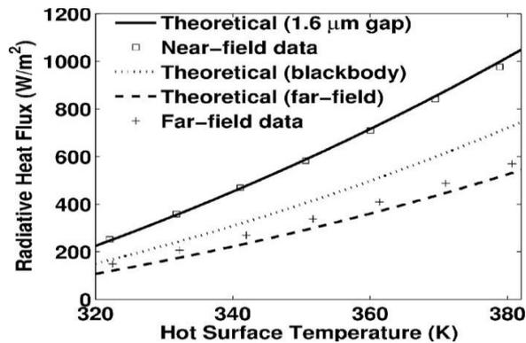
Figure 2.10. Experimental Results (Hu *et al.*, 2008).
