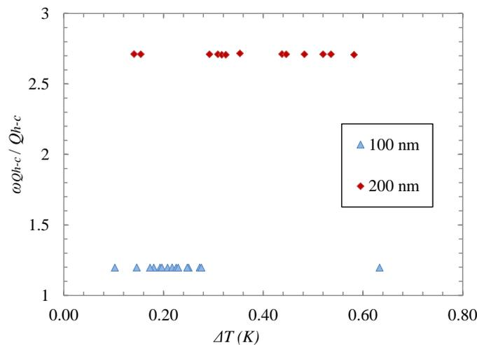
Figure 5.7. Relative uncertainty  $\omega_{Q_{h-c}} / Q_{h-c}$  vs.  $\Delta T$ .
