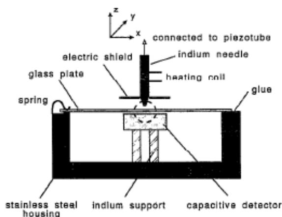
Figure 2.4. Experimental setup (Xu *et al.*, 1994).
