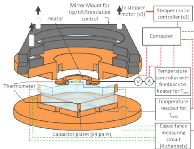
Figure 2.17. Experimental setup (Ottens *et al.*, 2011).
