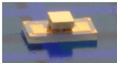
Figure 3.21. Nextreme UPF4 Optocooler<sup>TM</sup> thermoelectric cooler (1.5x2.5 mm<sup>2</sup> footprint) (NextremeThermal Solutions, 2009).
