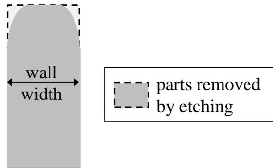
Figure 3.15. Effect of etching process on wall width.
