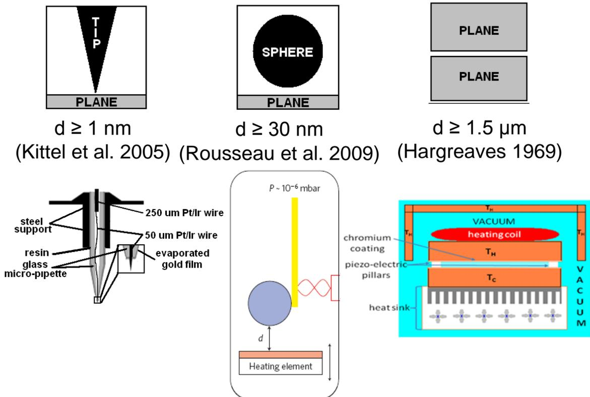
Figure 2.16. Minimum near-field measurement gaps at different geometries.
