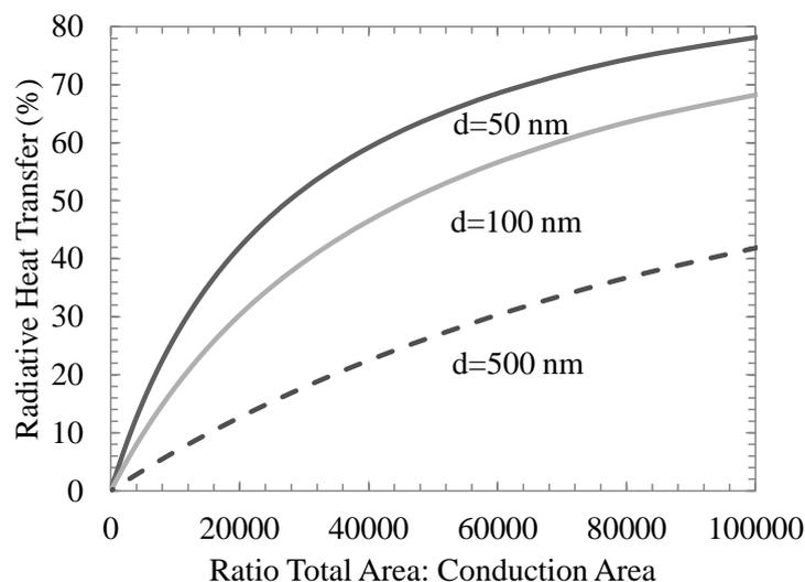
Figure 3.11. Radiative heat transfer percent vs. total area: conduction area.
