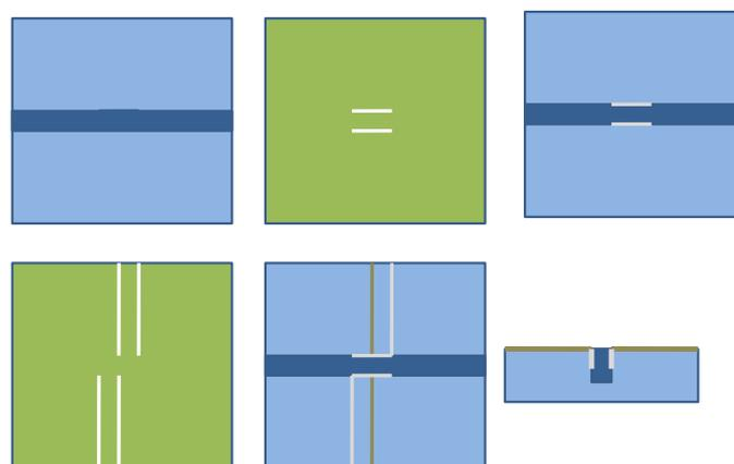
Figure 3.8. Mask and vapor deposition of thermo-couples.
