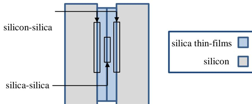
Figure 4.3. Sample interfaces with possible thermal contact resistance.
