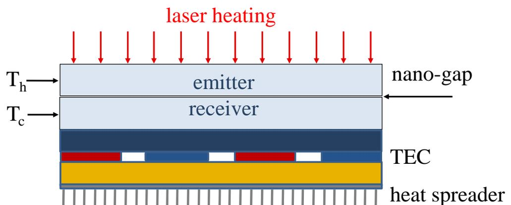
Figure 3.4. Option 1 sample and test setup design.
