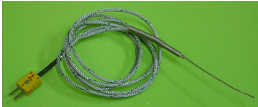
Figure 3.15. Ceramic insulated K type thermocouple
