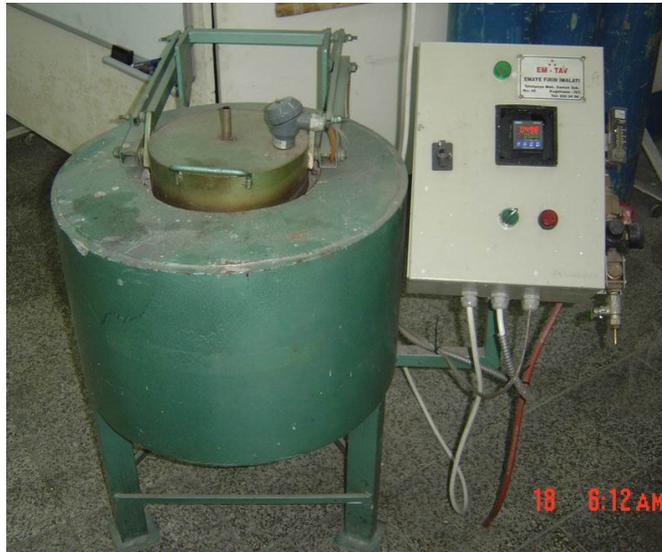
Figure 3.5. Annealing furnace
