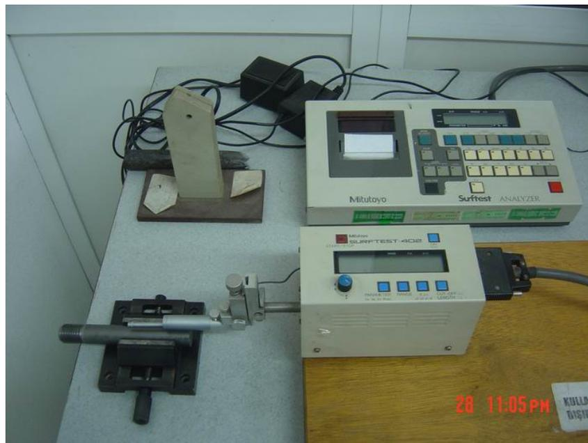
Figure 3.48. Surface roughness measurement machine in KOSGEB - Istanbul
