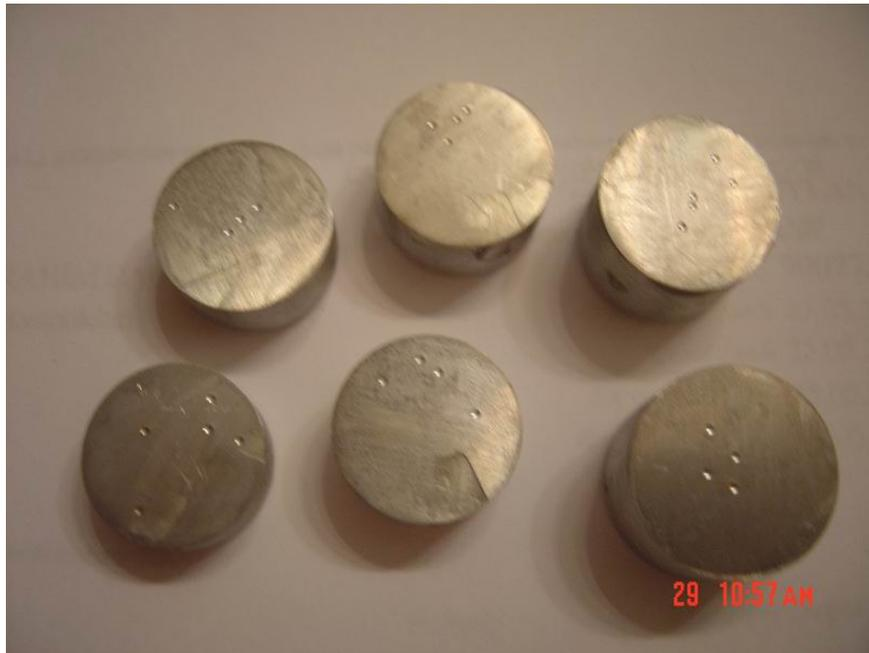
Figure 3.52. Samples were subjected to Brinell Hardness Test
