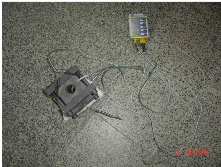
Figure 3.23. Connection of thermocouples to Curve-X and die
