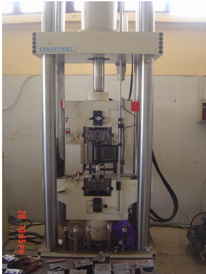
Figure 3.55. Tensile testing machine in KOSGEB - Istanbul
