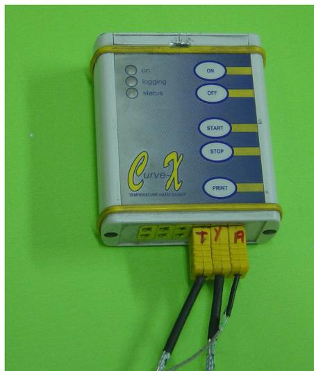
Figure 3.16. Curve-X Datalogger and thermocouple pin connection
