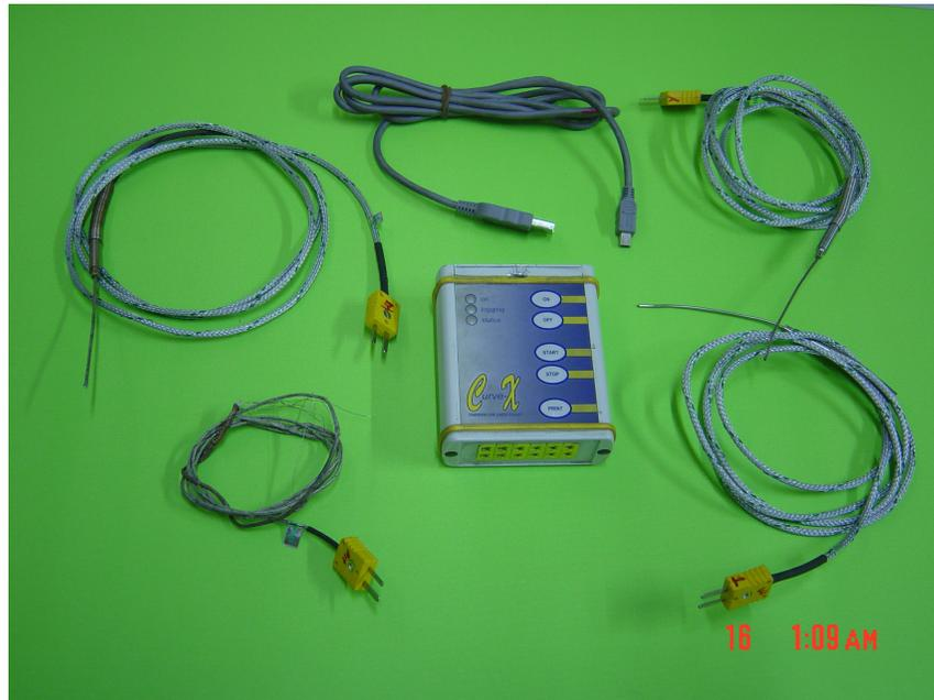
Figure 3.17. Temperature measurement set
