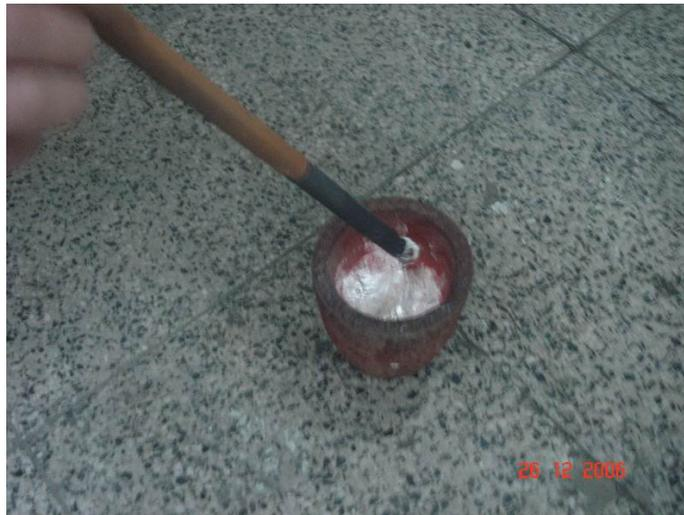
Figure 3.25. Stirring of molten metal in crucible
