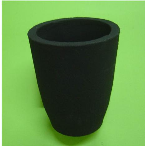
Figure 3.12. Clay graphite crucible
