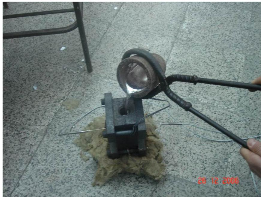
Figure 3.26. Pouring molten metal into the die
