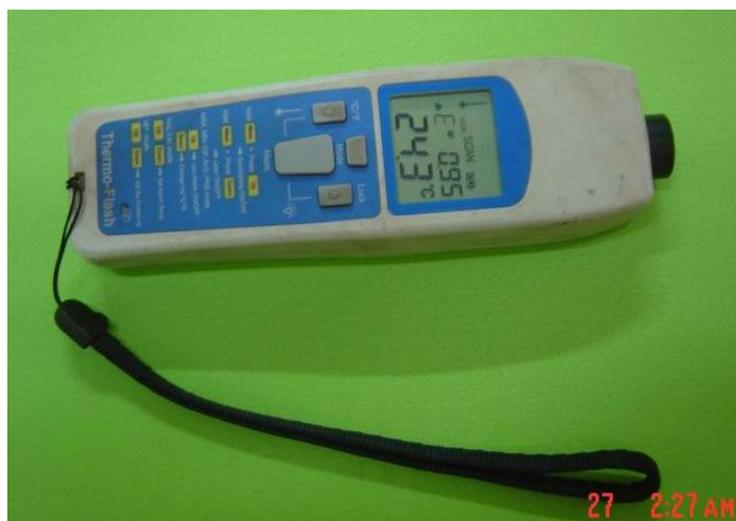
Figure 3.19. Infrared thermometer
