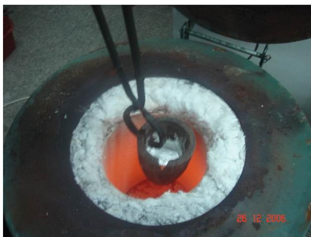
Figure 3.22. Taking out the crucible from melting furnace
