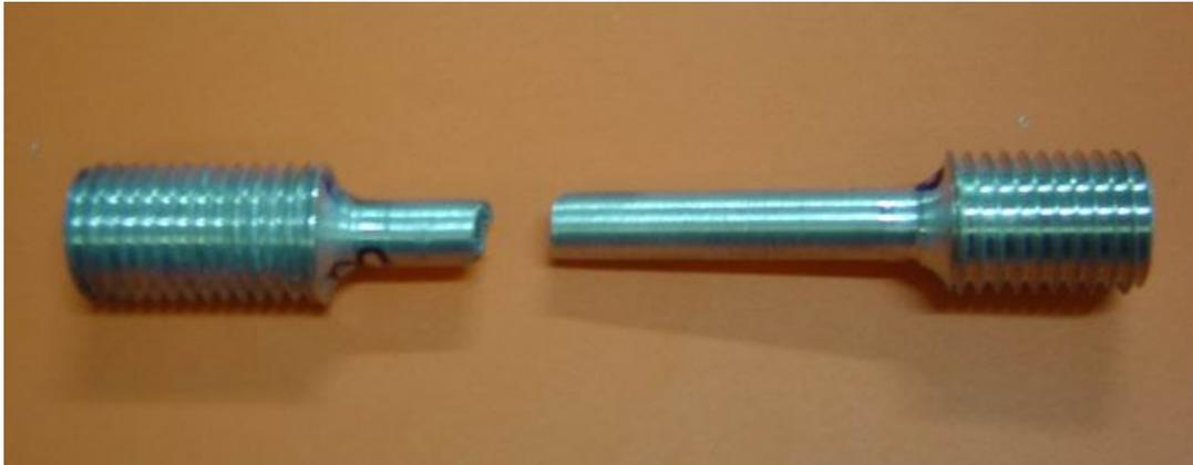
Figure 4.18. A broken specimen in tensile testing
