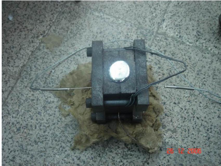
Figure 3.27. Molten ZA-27 alloy just poured
