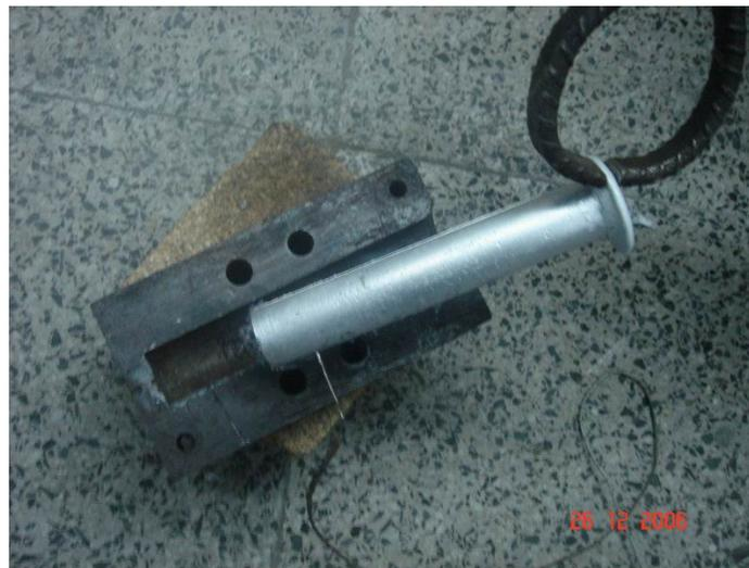
Figure 3.28. Specimen while taken out from the die
