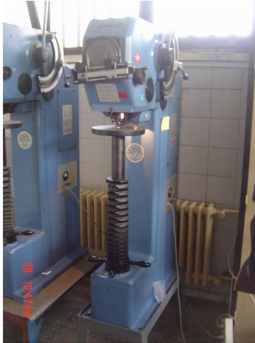
Figure 3.50. Brinell testing machine in KOSGEB - Istanbul
