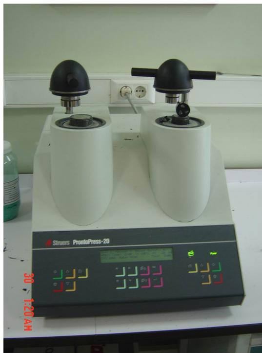
Figure 3.60. Bakelite mold preparation machine
