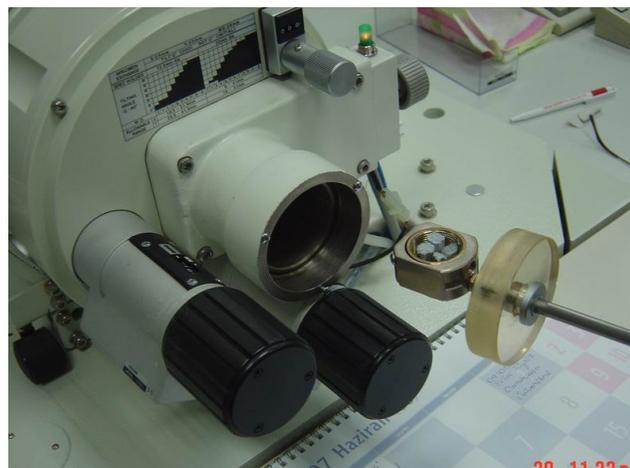
Figure 3.58. Inserting of adaptor in SEM
