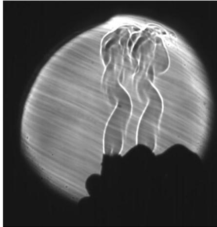
Figure 4.9. The double view of Schlieren image of the single lighter plume.
