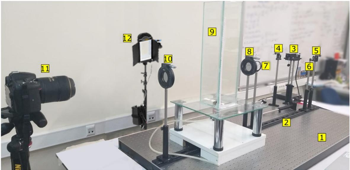
Figure 4.2. Optical setup. (1) Optical table, (2) Optical rail system, (3) Laser, (4-5) Kinematic frames and mirrors, (6) Plano-concave lens, (7) Plano-convex lens, (9) Liquid column, (8-10) Polarizers, (11) Camera, (12) Illuminator.
