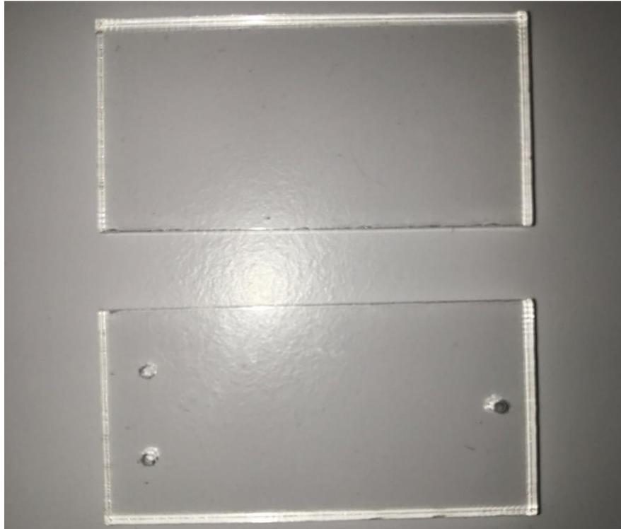
Figure 3.5. Laser cut PMMA sheets with the dimensions of 50 x 25 x 3 mm
