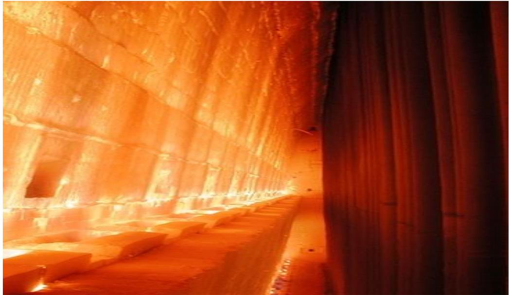
Figure 2.3. Inside of Terrace Wall <sup>TM</sup> steam reformer radiant box.
