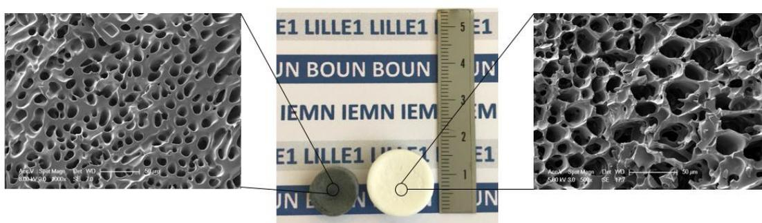
Figure 6.3. Hydrogel samples prepared using similar amount of monomers and SEM images of cryogels with (left) and without (right) embedded rGO.
