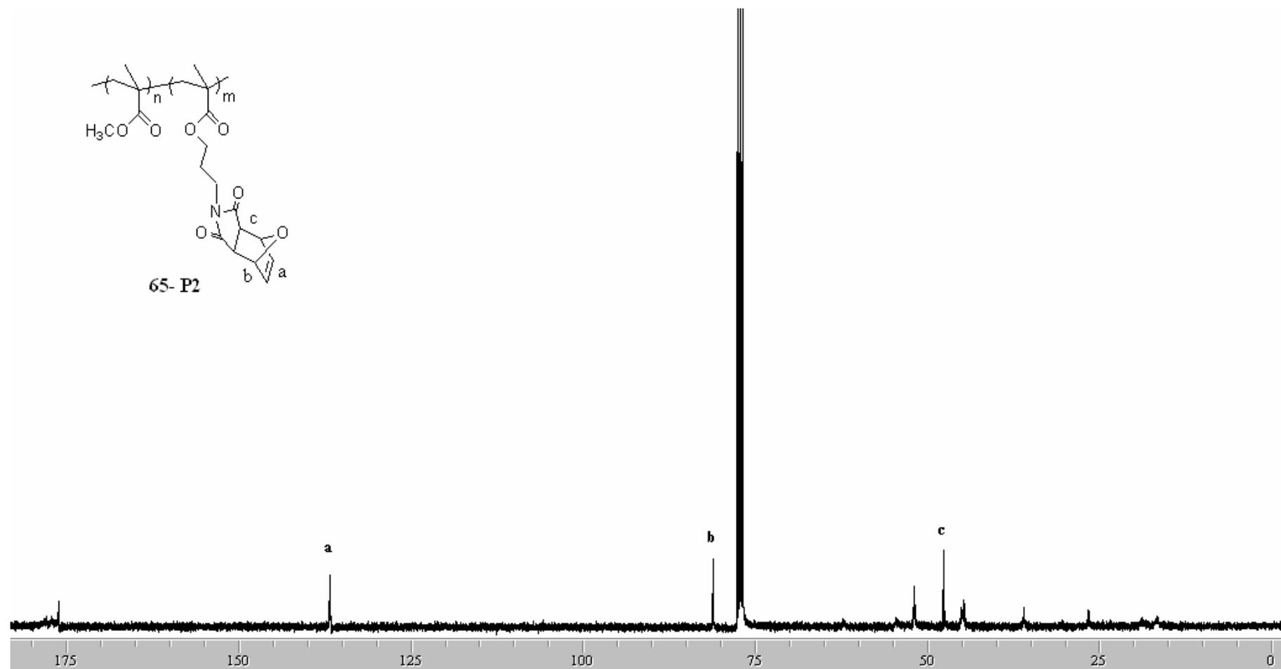
Figure A.7.  $^{13}\text{C}$  NMR spectrum of maleimide copolymer **P2**
