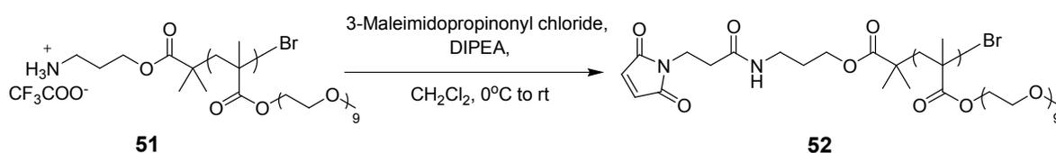
Figure 3.5. Post functionalization of 1° amine terminated polymer
