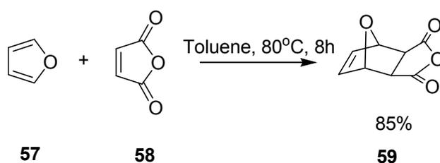
Figure 5.2. Synthesis of furan-maleic anhydride adduct
