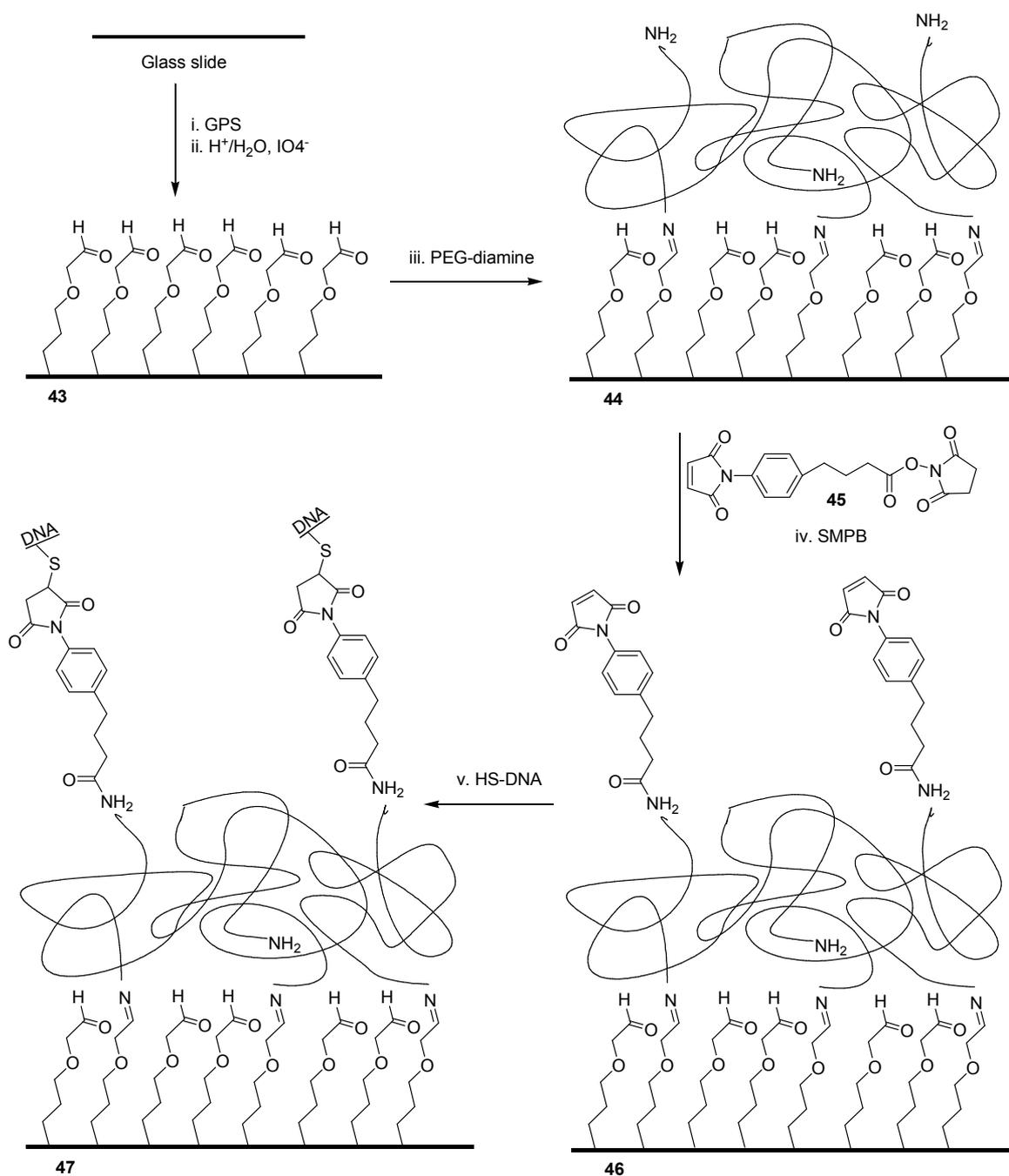
Figure 3.3. Schematic representation of the procedure for preparing PEG-grafted, maleimide terminated surfaces for the immobilization of thiolated DNA oligonucleotides
