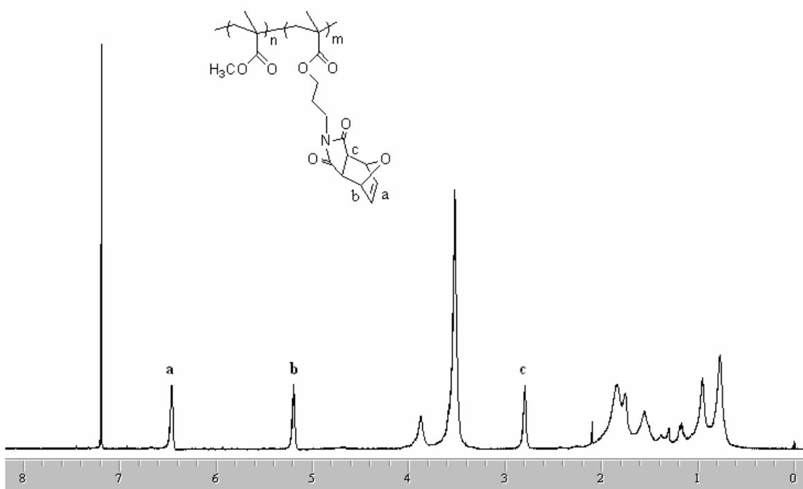
Figure 5.10. <sup>1</sup>H NMR spectrum of latent-maleimide polymer
