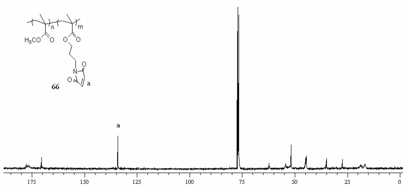
Figure A.11.  $^{13}\text{C}$  NMR spectrum of maleimide copolymer **P2** after retro Diels-Alder reaction (**P5**)
