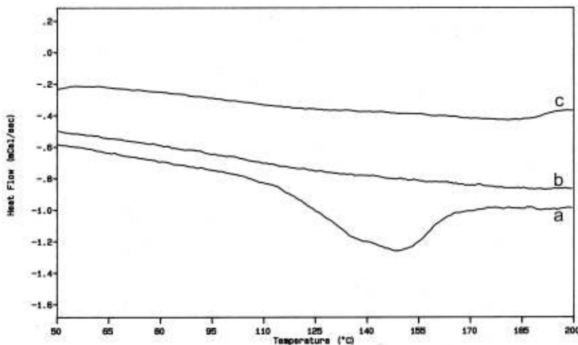
Figure 5.17. DSC thermogram of P2 (a: 1<sup>st</sup> heating, b: 2<sup>nd</sup> heating) and P5 (c)
