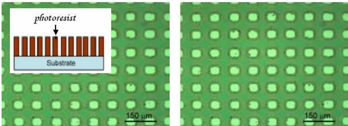
Picture 6.1. Microscopic view of the mold used for the preparation of PDMS stamp
