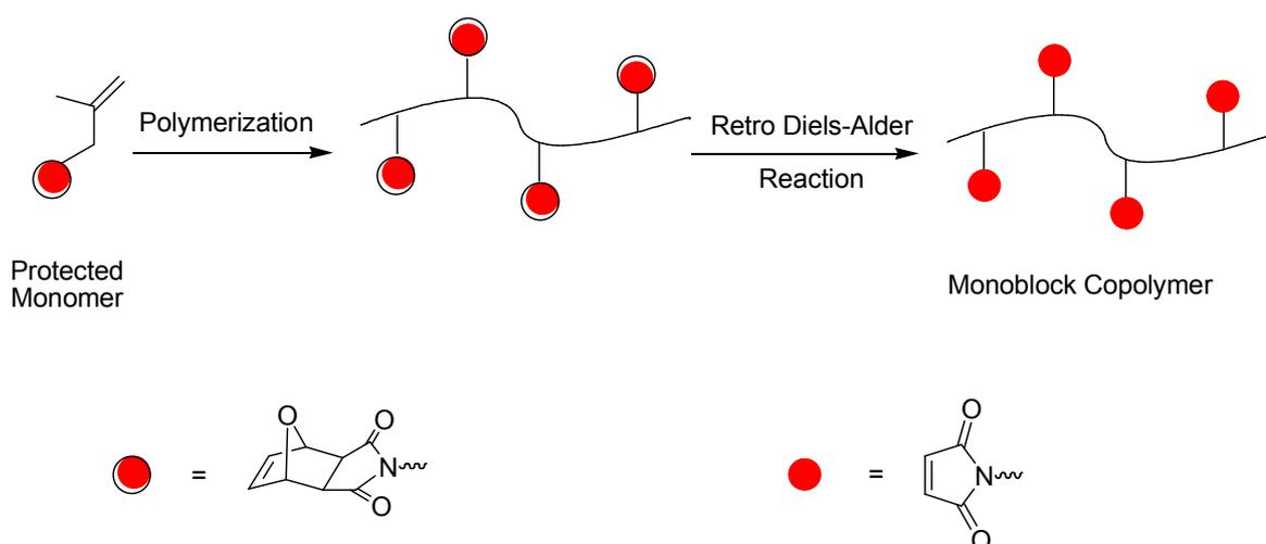
Figure 4.1. Illustration of polymer synthesis via DA / rDA sequence
