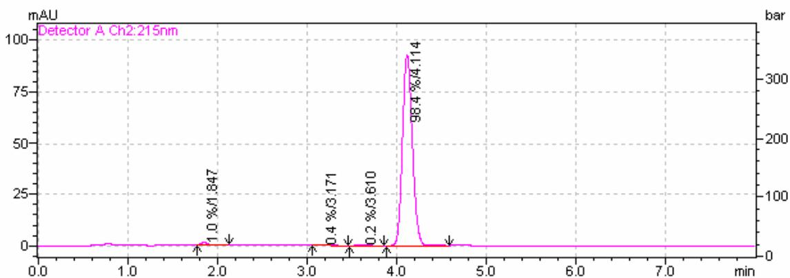
Figure 5.5. HPLC of latent-maleimide containing monomer **63**
