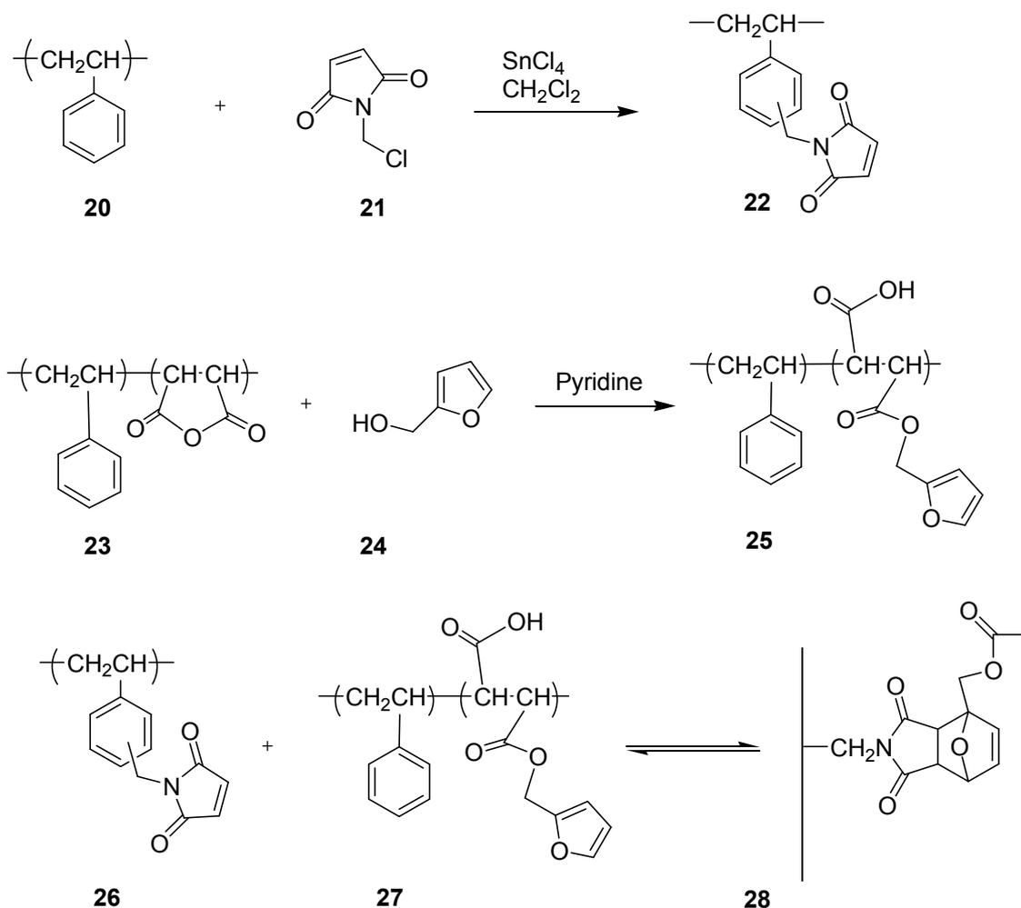
Figure 2.8. Modification of styrene polymers for crosslinking
