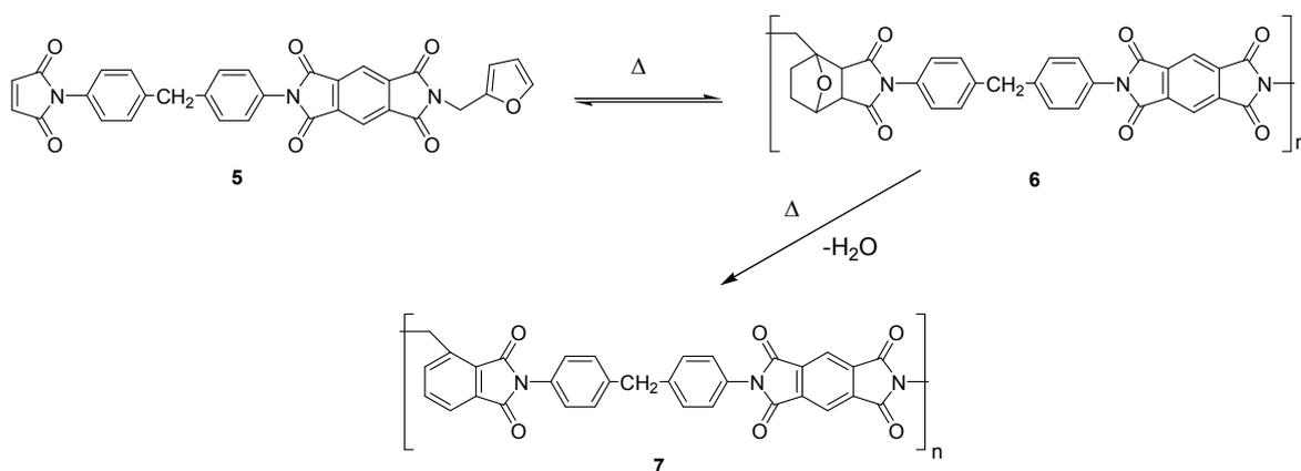
Figure 2.3. Diels-Alder polymerization of AB type of monomer
