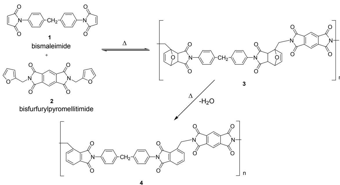
Figure 2.2. Diels-Alder polymerization of AA and BB type of monomers
