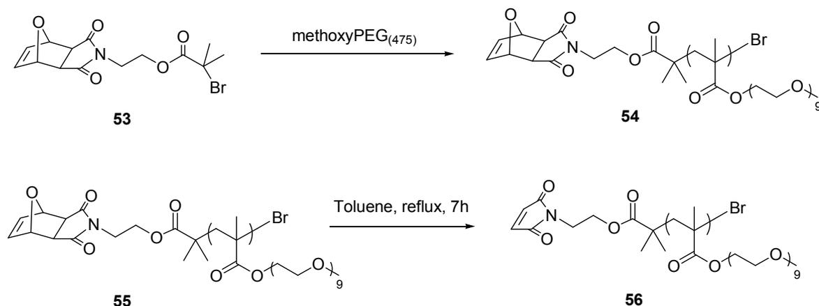
Figure 3.6. Synthesis of maleimide terminated polymer
