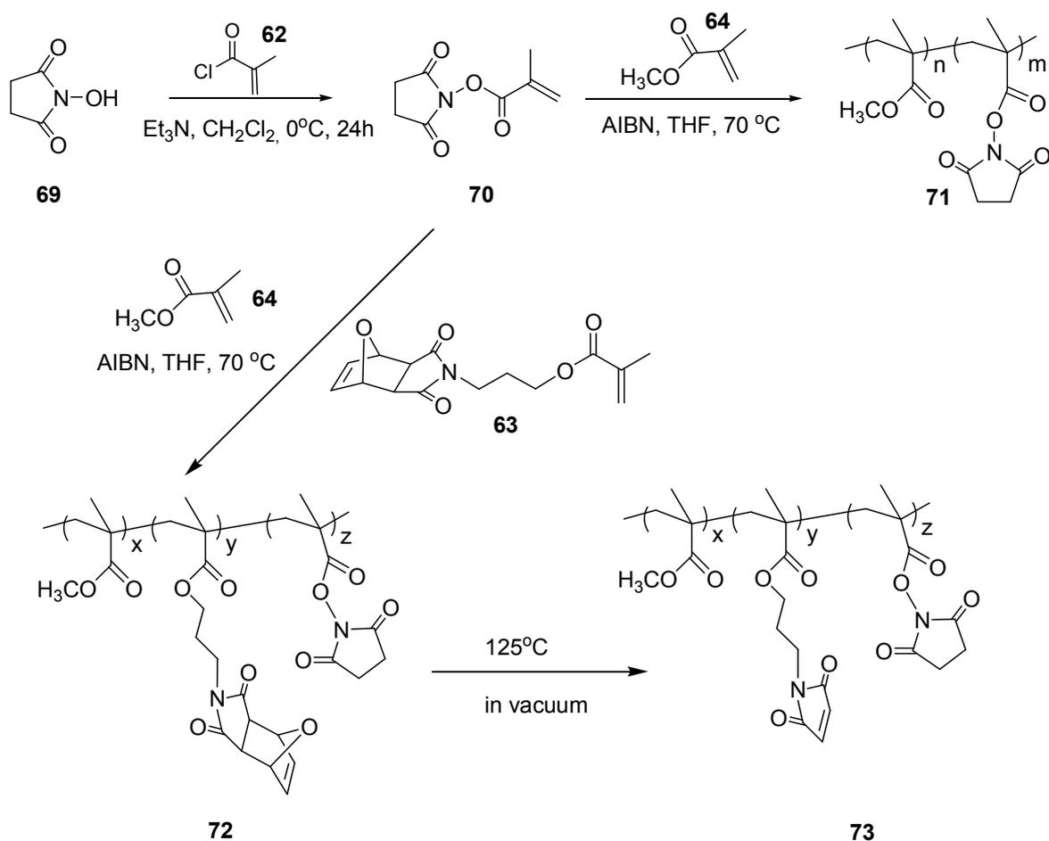
Figure 5.21. Synthesis of polymers bearing two reactive moieties
