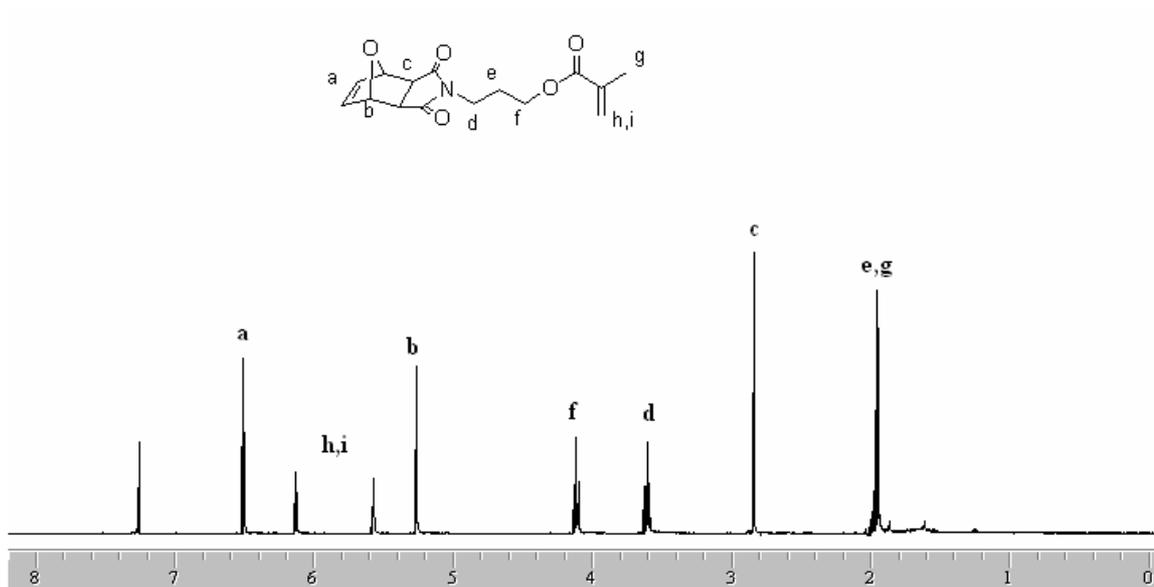
Figure 5.6  $^1\text{H}$  NMR spectrum of latent-maleimide containing monomer
