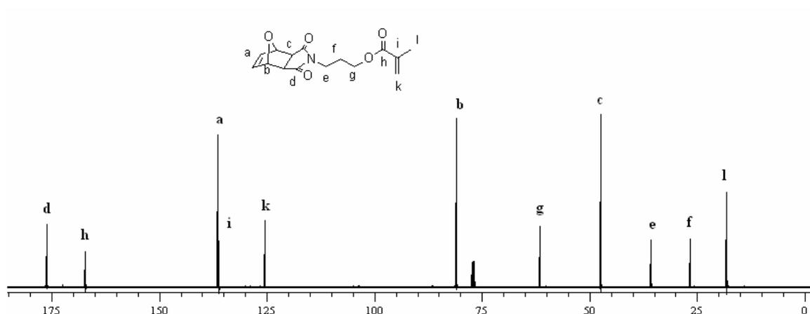
Figure 5.7.  $^{13}\text{C}$  NMR spectrum of latent-maleimide containing monomer
