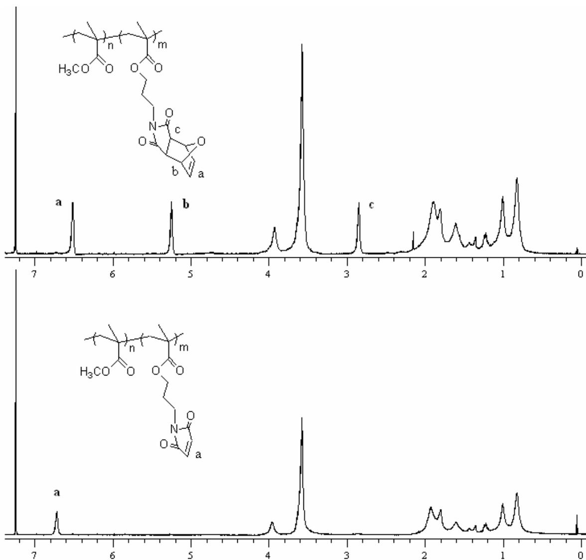
Figure 5.14  $^1\text{H}$  NMR spectra of polymer before and after rDA
