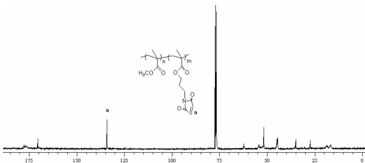
Figure 5.15.  $^{13}\text{C}$  NMR spectrum of reactive polymer
