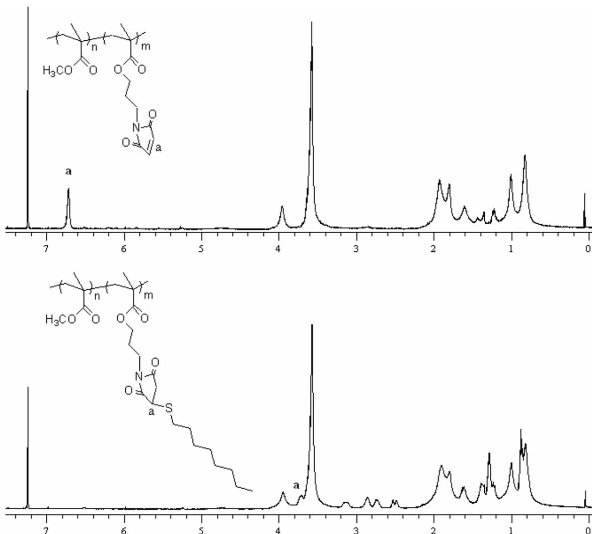
Figure 5.19.  $^1\text{H}$  NMR spectra of polymer before and after thiol addition
