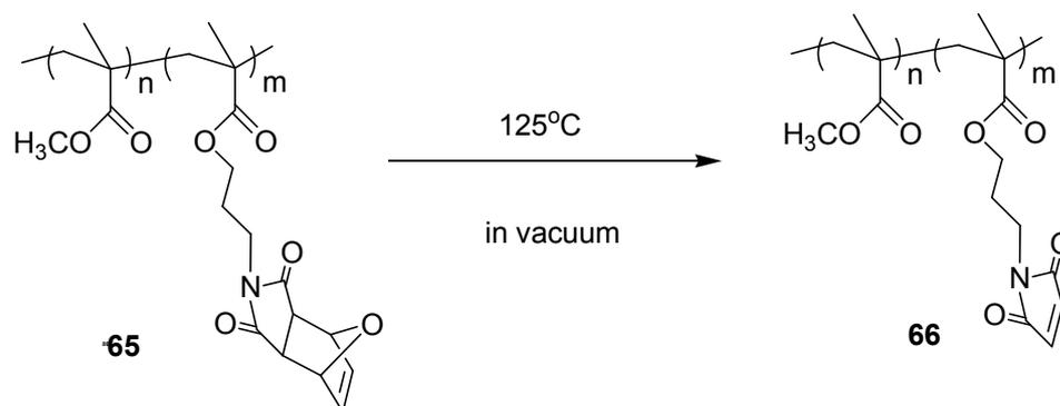
Figure 5.13. Synthesis of the reactive polymer
