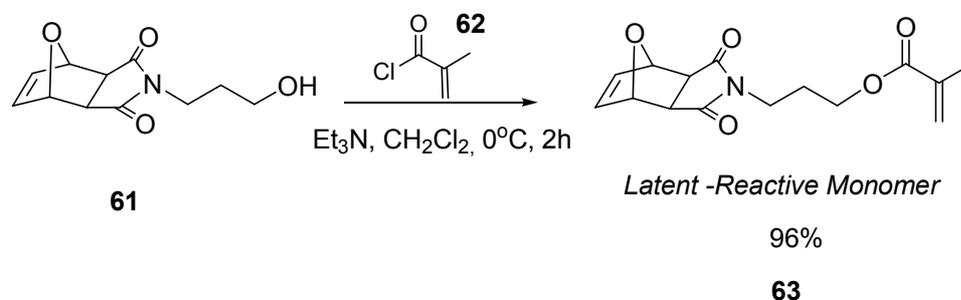
Figure 5.4. Synthesis of latent-maleimide containing monomer
