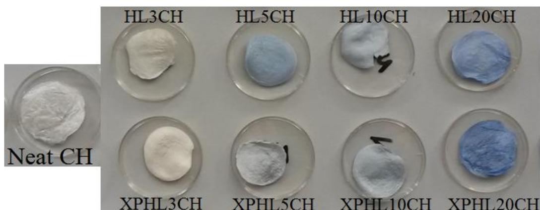
Figure 4.27. Photographs of hydrogels after desorption test of cationic dye adsorption.
