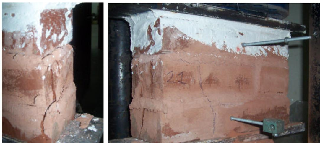
Figure 3.25. Failure of the masonry specimen
