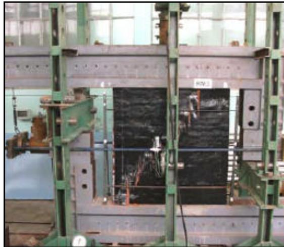
Figure 8. 5. The tested RM3 wall (vertical applied CFRP) [45]
