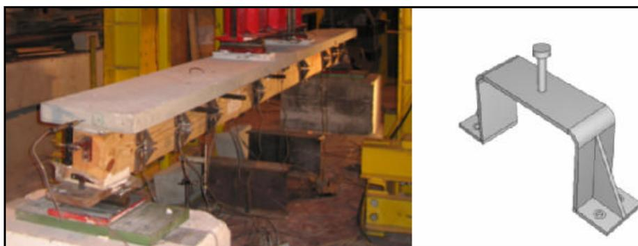
Figure 8. 26. Application of concrete over timber beams with steel connector [49]
