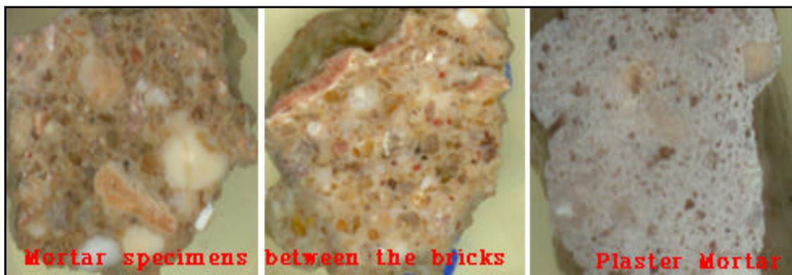
Figure 3.12. Mortar specimens, prepared for SEM and EDX analysis
