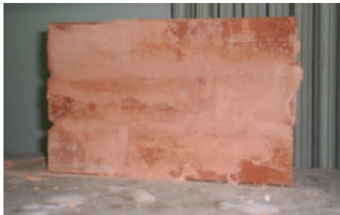
Figure 3.23. Compression test specimen with 1.8 cm mortar height and 6.5 cm brick height
