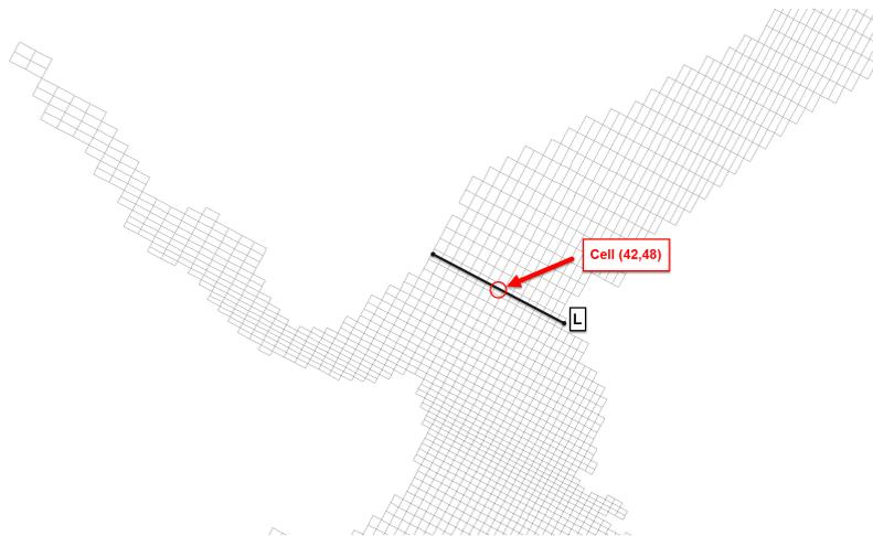
Figure 5.27. Sketch of cross-section used for calculation of the Reynolds No.
