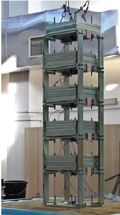
Figure 3.17. 1:10 Scaled 5-Story Building Model with St 42 Steel Column.
