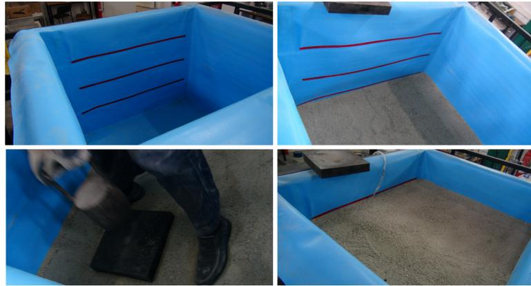
Figure 3.27. Soil Filling and Compaction.
