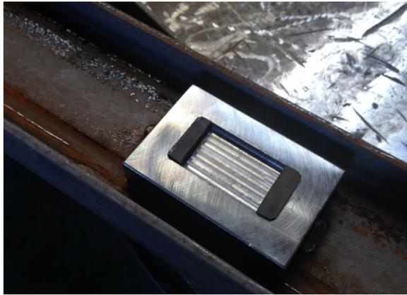
Figure 3.9. A View of Roller Bearing House with Rubber Strip Stopper.
