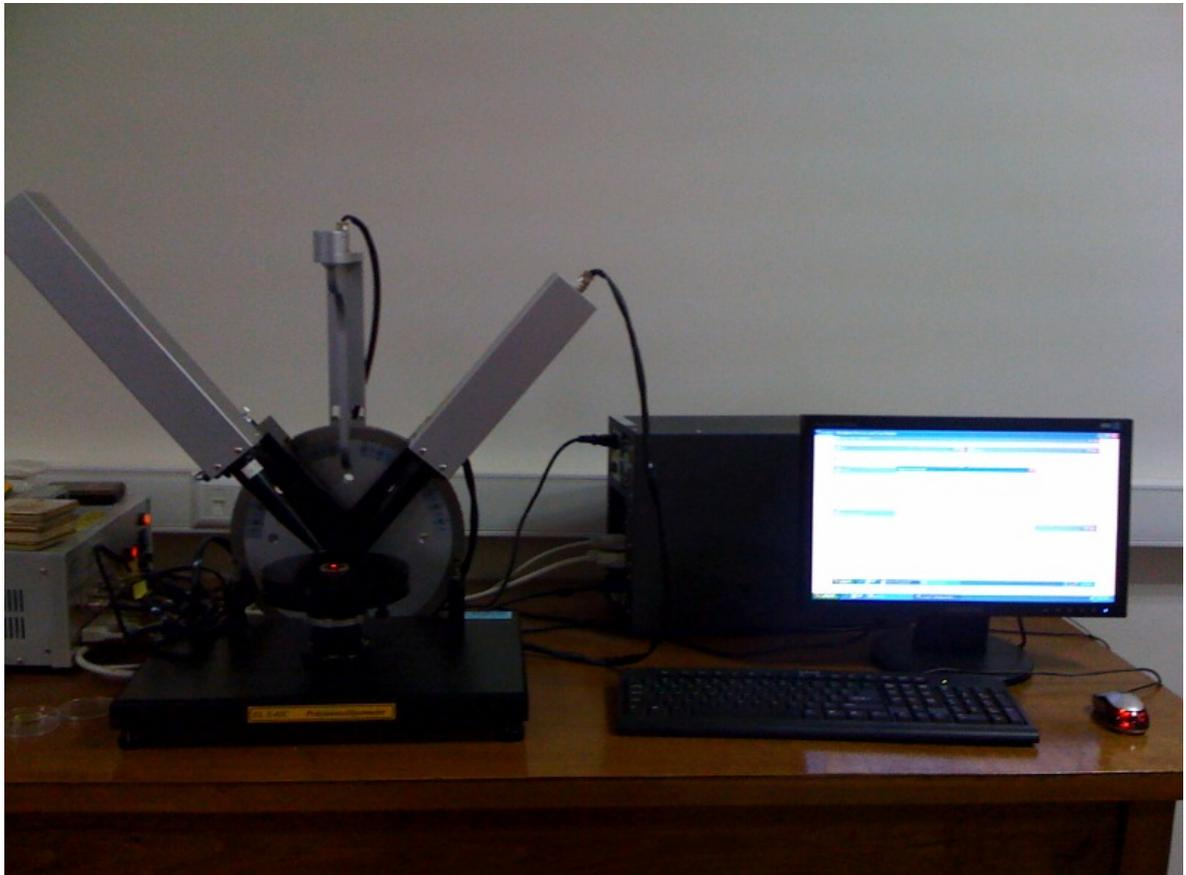
Figure 3.2. Picture of the ellipsometry used in our experiments
