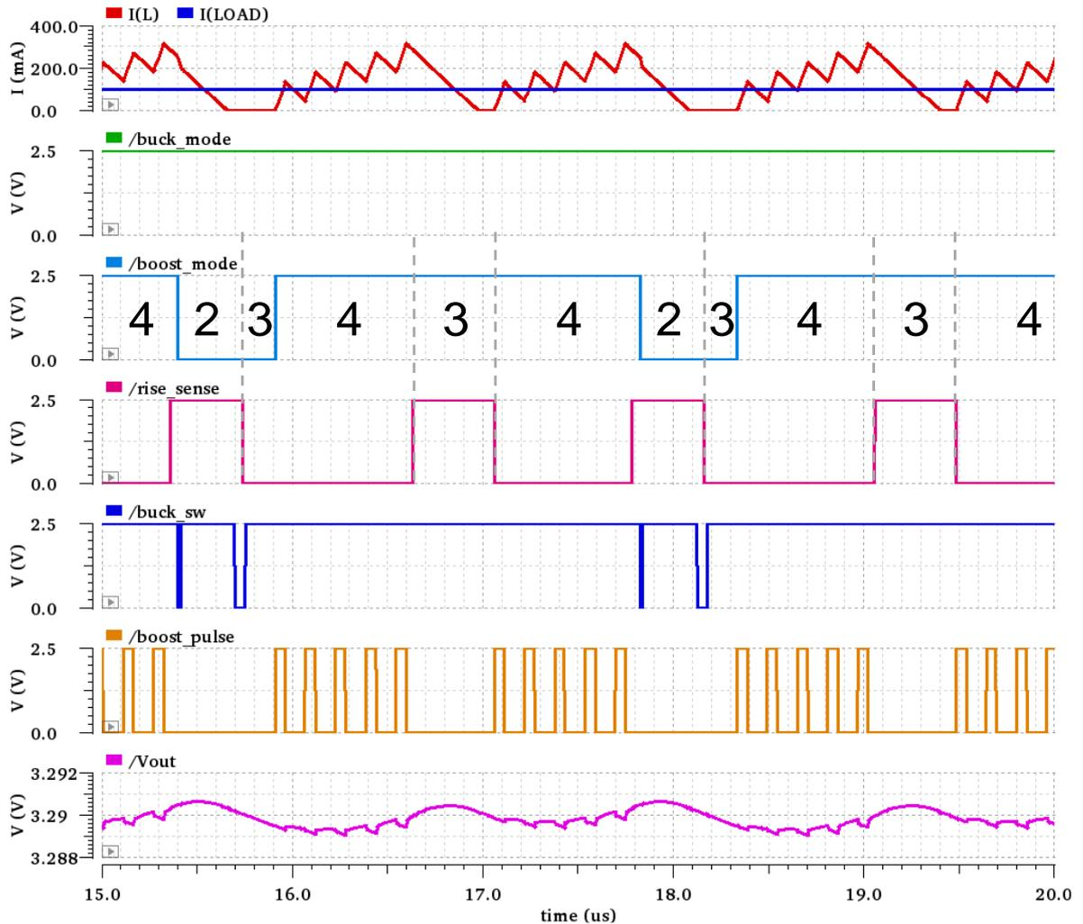
Figure 5.6. Simulation results for  $V_{IN}=2.5V$ ,  $V_{OUT}=3.3V$   $I_{LOAD}=100mA$ .
