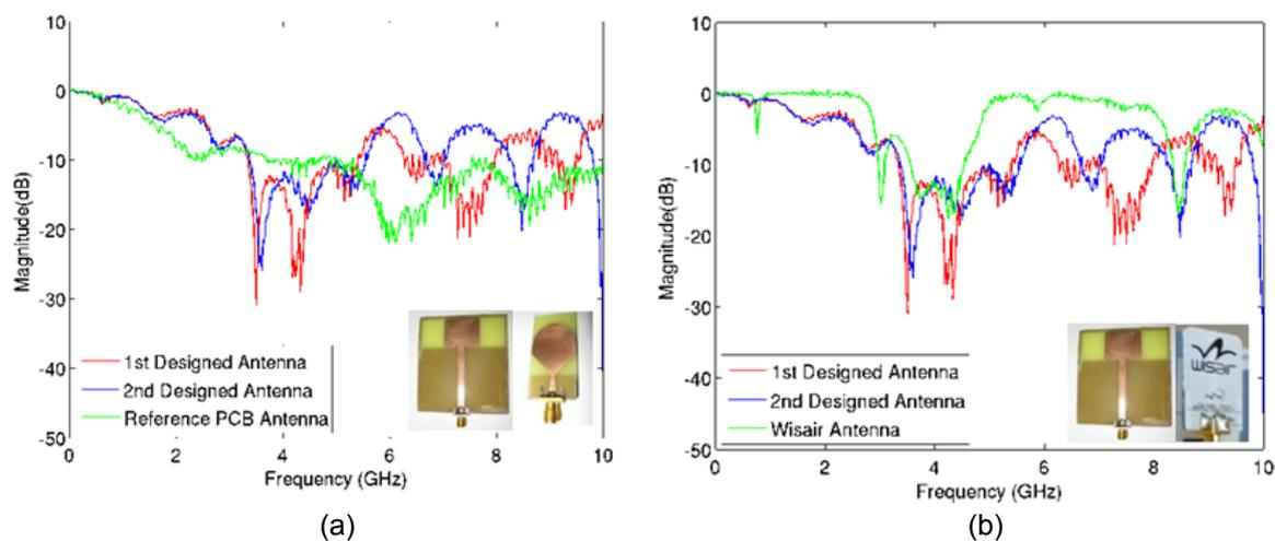
Figure 6.6. S11 comparisons (a) designed antenna vs. reference antenna (b) designed antenna vs. commercial antenna.
