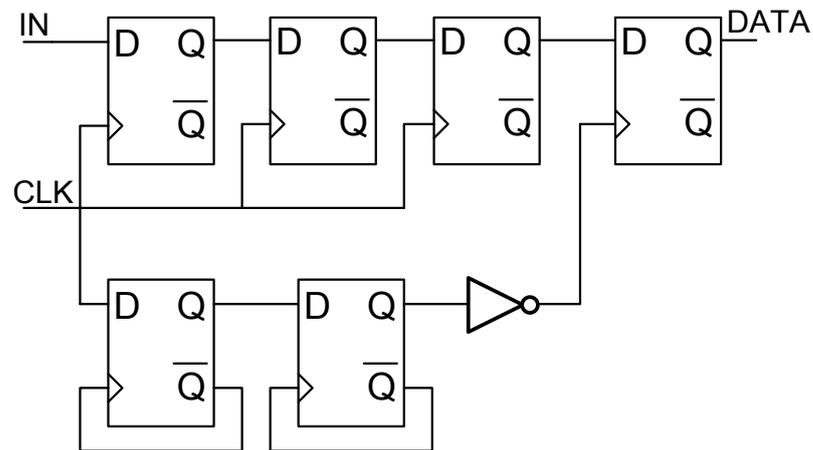
Figure 5.31. High frequency sampler and demodulator.
