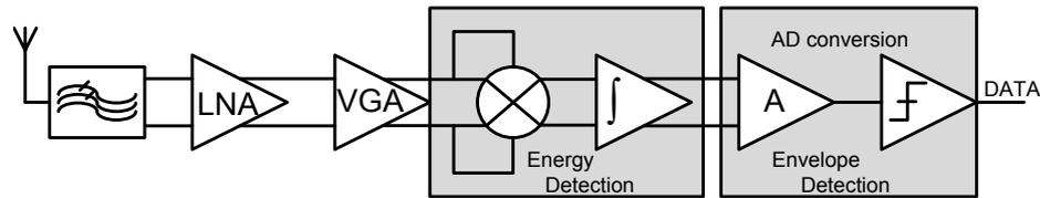
Figure 5.2. Non-coherent receiver block diagram.
