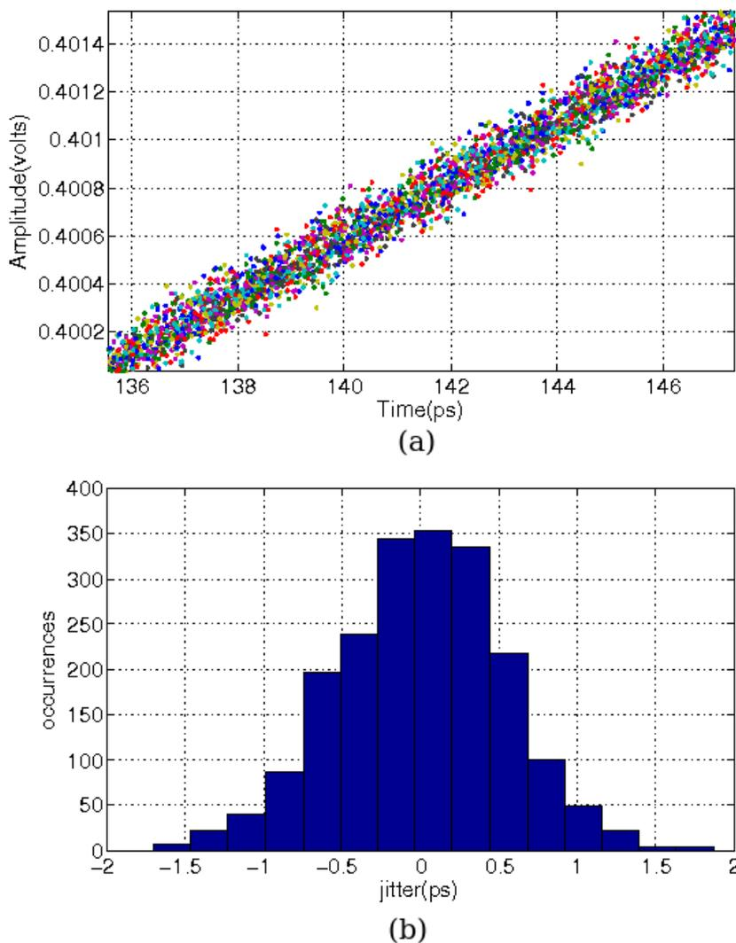
Figure 5.49. Jitter measurements (a) jitter plot, (b) jitter histogram.
