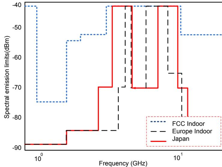
Figure 1.1. UWB Spectrum Limits.
