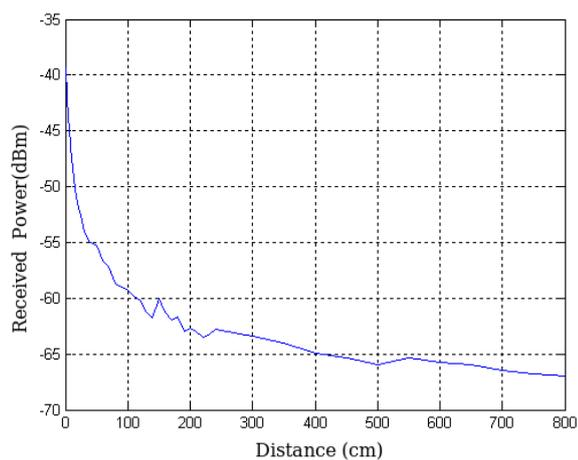
Figure 7.2. Output Power of Wisair Development Board.
