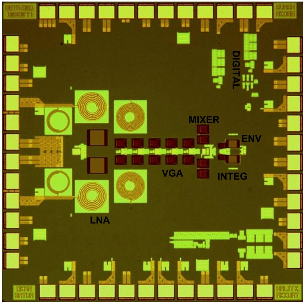
Figure 5.14. Receiver micrograph.
