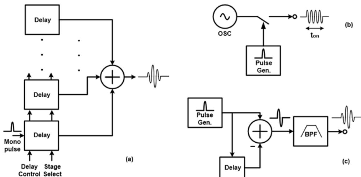
Figure 4.1. Transmitter architectures (a) Pulse combination, (b) Oscillator, and (c) Filtering methods.
