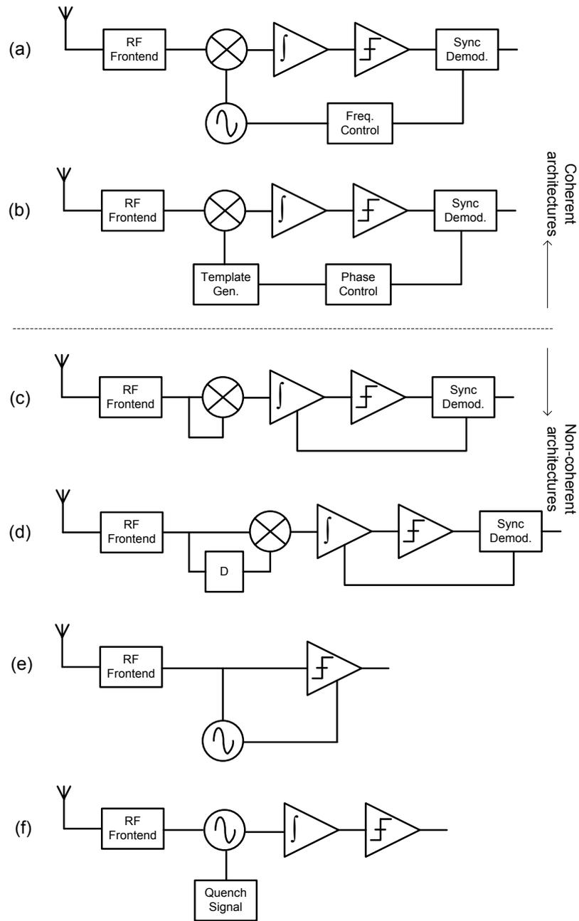
Figure 5.1. Receiver architectures for coherent and non-coherent IR-UWB; (a) Coherent clock synchronization, (b) Template pulse, (c) Energy detection, (d) Transmitted reference, (e) Injection locking, and (f) Super-regenerative.
