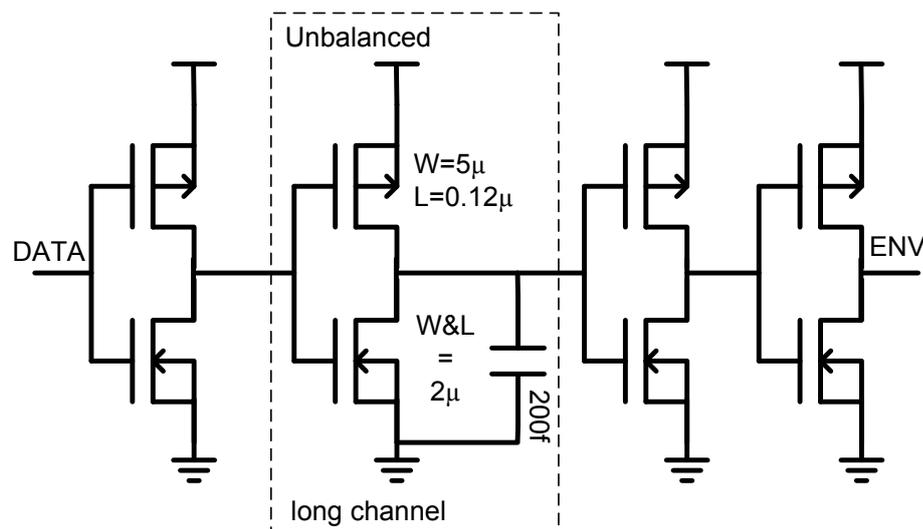
Figure 5.24. Digital envelope detector circuit.
