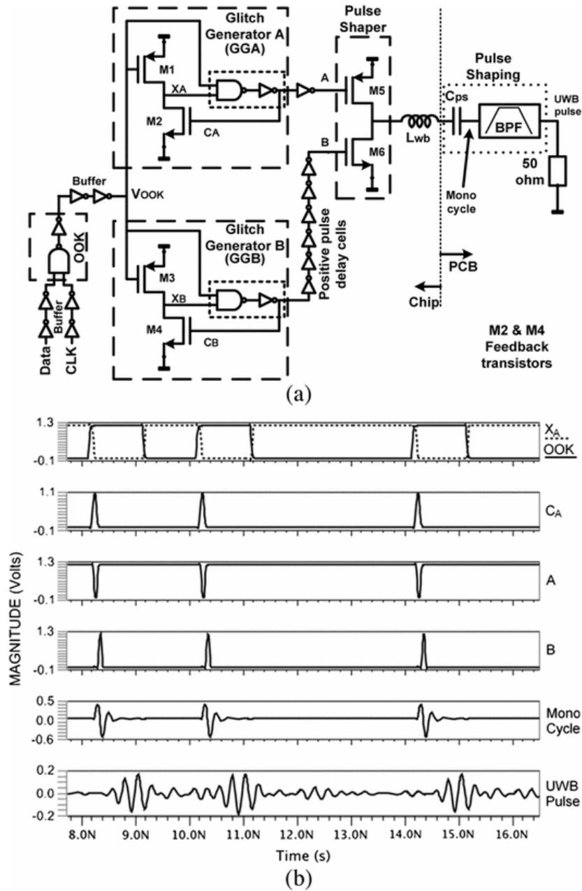
Figure 4.4. (a) Block diagram of the proposed transmitter and (b) post-layout transient simulation results of the internal and external nodes.
