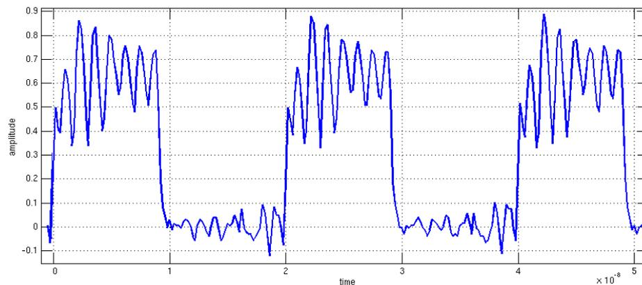
Figure 5.30. Self correlation demodulation result at 100 Mbps.
