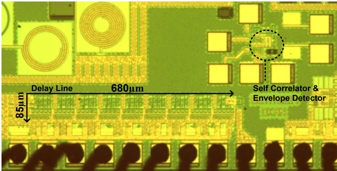
Figure 5.33. Micrograph of the implemented designs.
