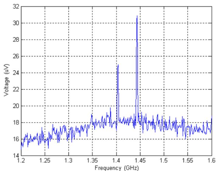
Figure 2.4. Indoor EMF measurement taken at a computer lab.
