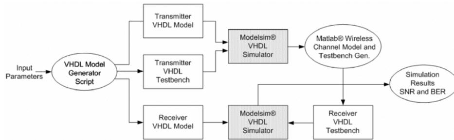
Figure 3.1. MATLAB - VHDL design flow.
