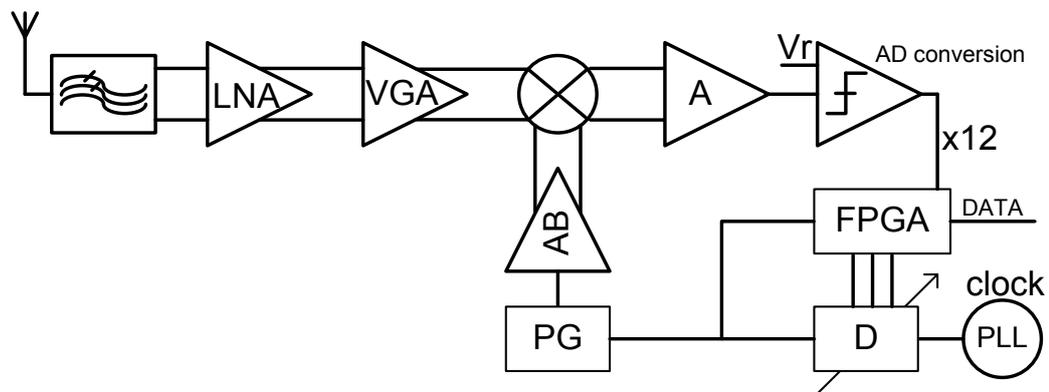
Figure 5.34. Template based coherent receiver.
