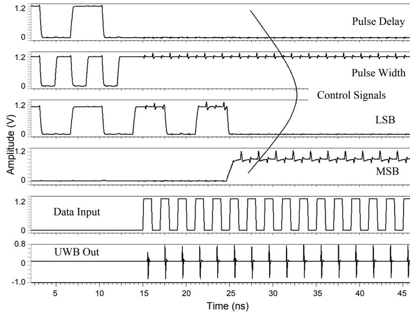
Figure 4.19. Simulation of configuration input signals and transmitter output.
