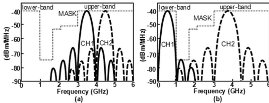
Figure 4.2. Dual-band spectrum (a) conventional method, (b) designed transmitter.
