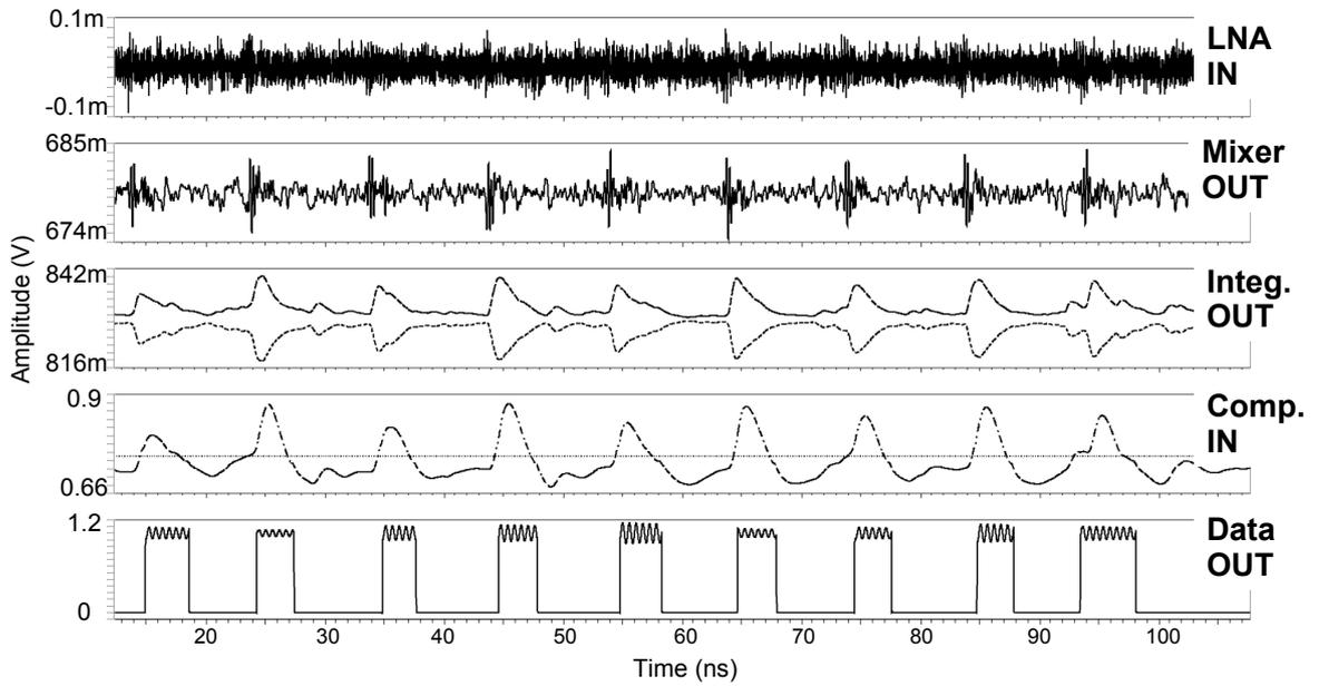
Figure 5.15. Receiver simulations.
