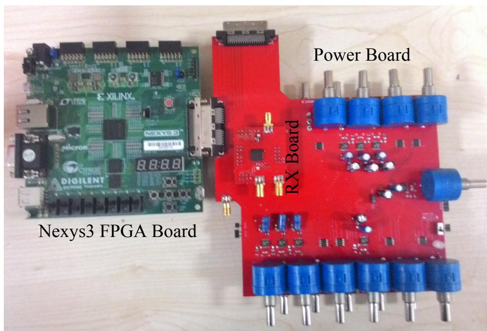
Figure 6.16. Coherent transceiver power and FPGA boards.
