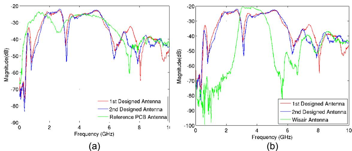
Figure 6.8. S21 comparisons for 10cm distance (a) designed antennas vs. reference antenna (b) designed antennas vs. commercial antenna.
