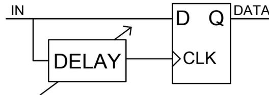
Figure 5.27. Self-correlator schematic.
