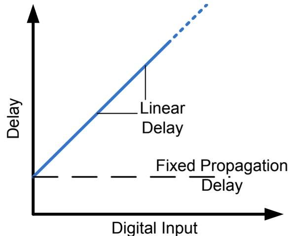
Figure 5.44. Propagation delay vs digital input.
