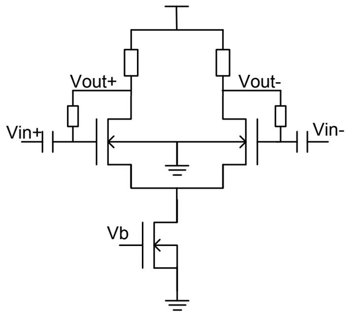
Figure 5.41. Schematic of single active balun stage.
