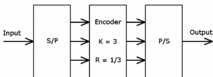
Figure 3.3. Convolutional encoder block diagram.
