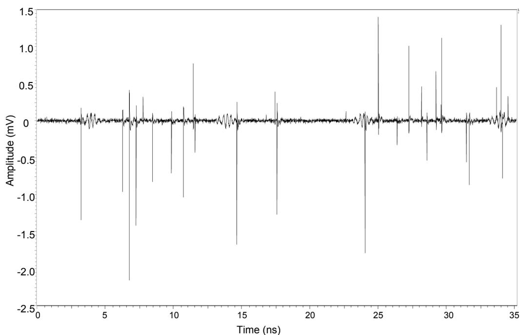
Figure 5.17. High intensity impulsive noise.
