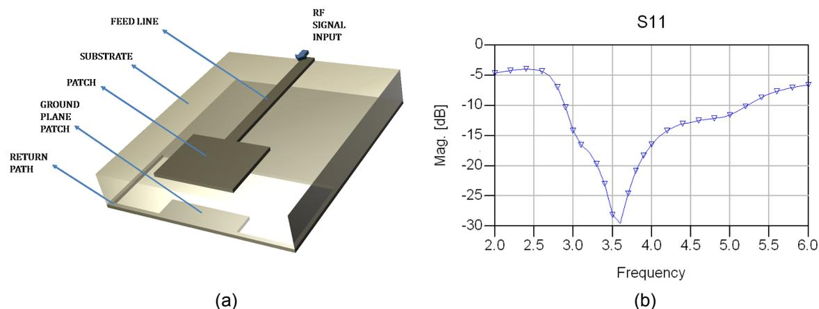
Figure 6.3. Proposed antenna; (a) Geometry (b) S11 simulation results.
