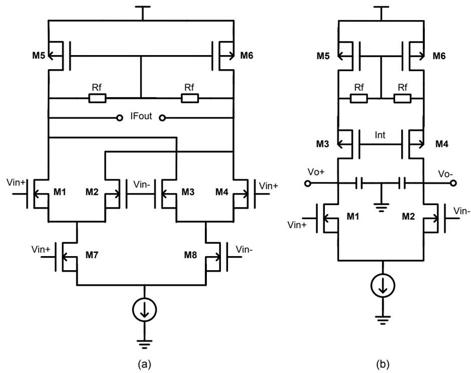
Figure 5.11. Energy detector; (a) Double balanced mixer, and (b) GmC integrator.
