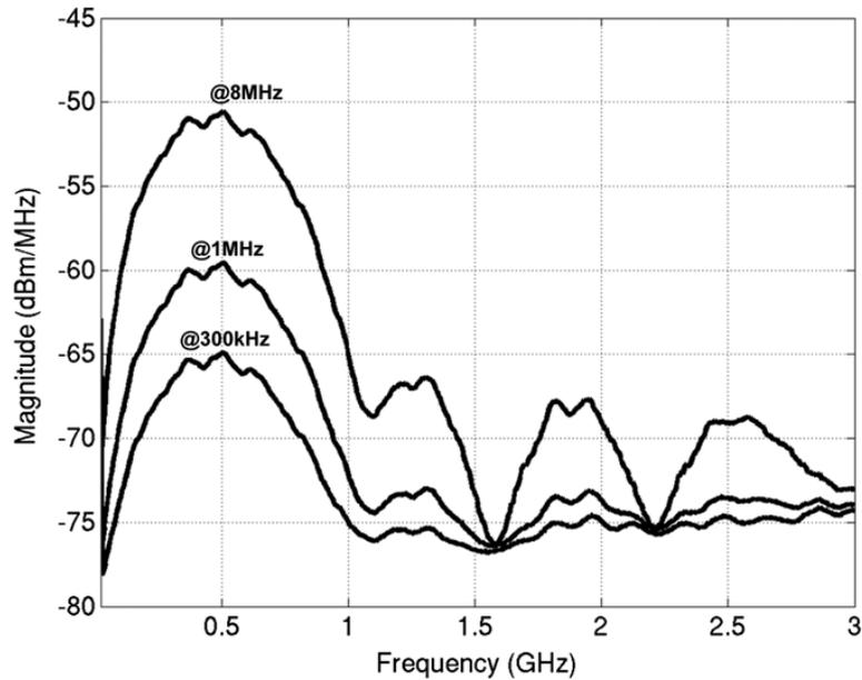
Figure 4.9. Spectrum measurement in the 0–960 MHz band with PRF at 300 kHz, 1 MHz, and 8 MHz.
