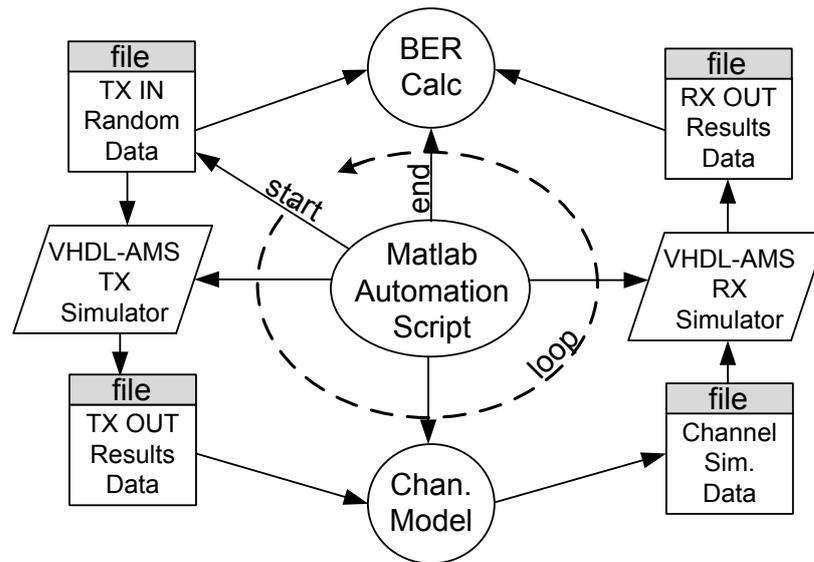
Figure 3.13. MATLAB and VHDL-AMS automated design flow.
