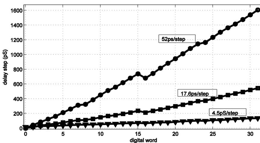
Figure 5.53. Delay vs digital word measurements.
