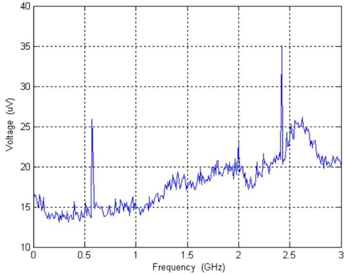
Figure 2.5. Indoor EMF measurement taken at a TV broadcast tower.
