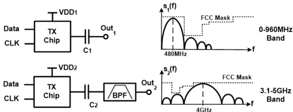
Figure 4.3. Transmitter reconfiguration for dual-band operation.
