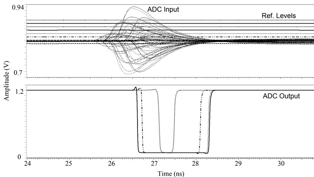
Figure 5.57. ADC inputs and outputs of the coherent receiver.
