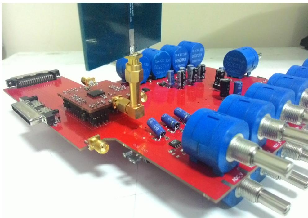
Figure 6.15. Coherent transceiver power board.
