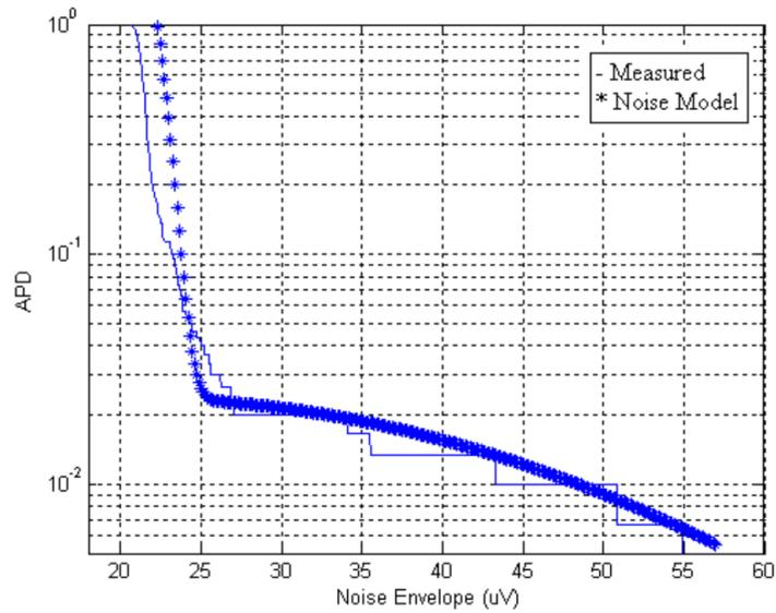
Figure 2.8. APD of Figure 2.4 and noise model fit.
