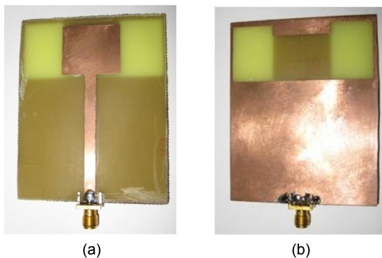
Figure 6.4. Proposed antenna; (a) top view (b) bottom view.
