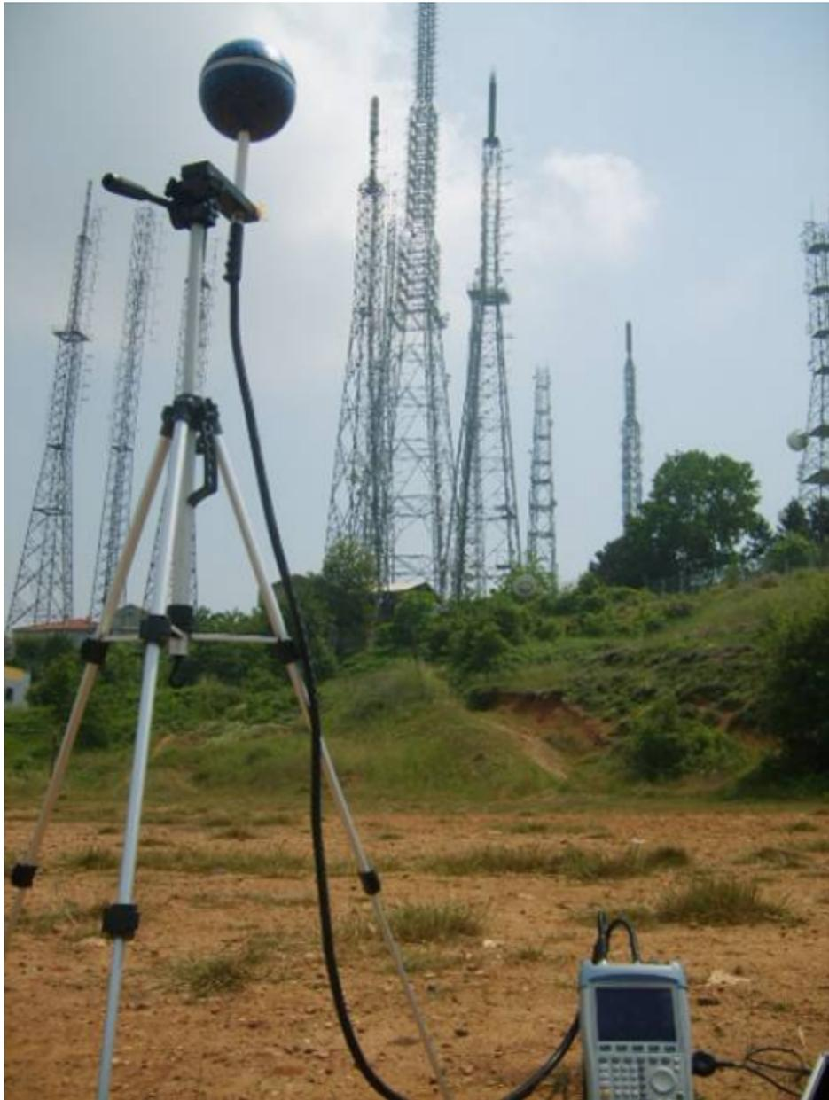
Figure 2.1. Rohde and Schwarz FSH-6 EMF measurement device.
