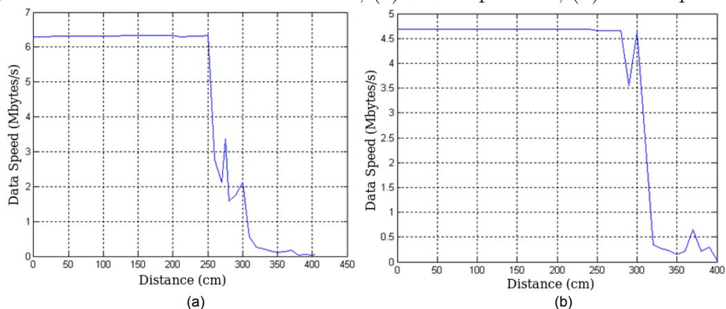
Figure 7.5. Performance of Wisair Board; (a) 160 Mbps mode, (b) 106.7 Mbps mode.
