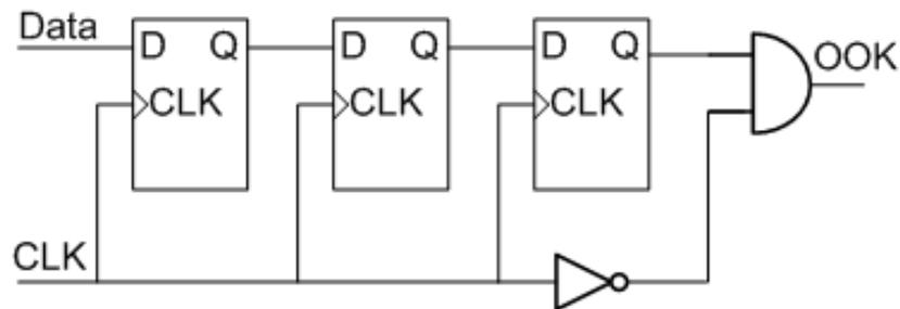
Figure 4.16. OOK modulator with synchronizer.
