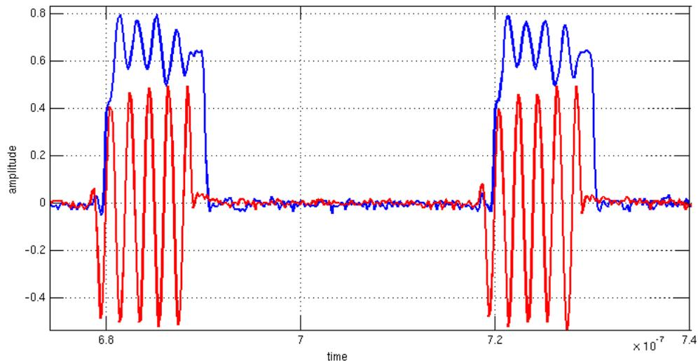
Figure 5.26. Digital envelope detector measurement results at 50 Mbps.
