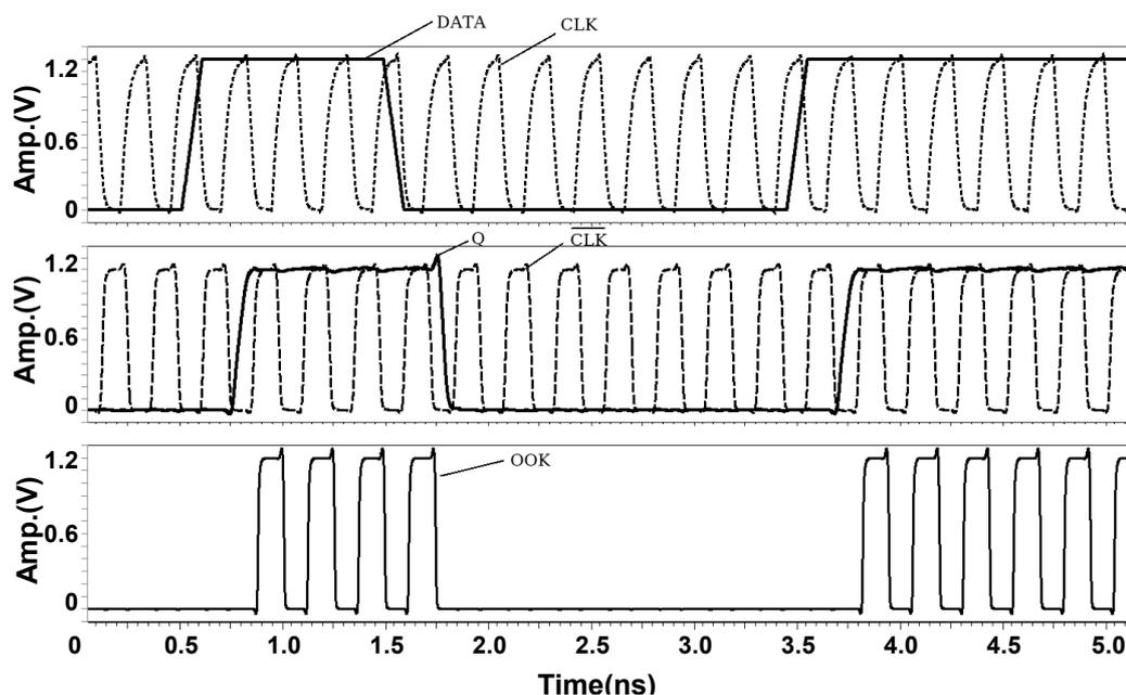
Figure 4.17. OOK modulator simulations.
