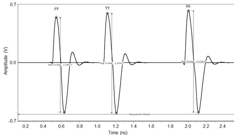
Figure 4.23. Time domain simulation of process variations.
