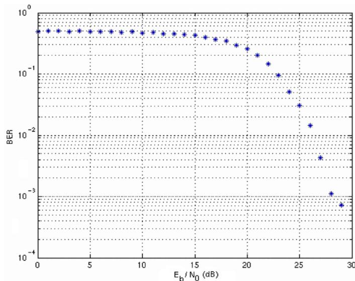
Figure 3.9. BER vs SNR of the overall UWB system.
