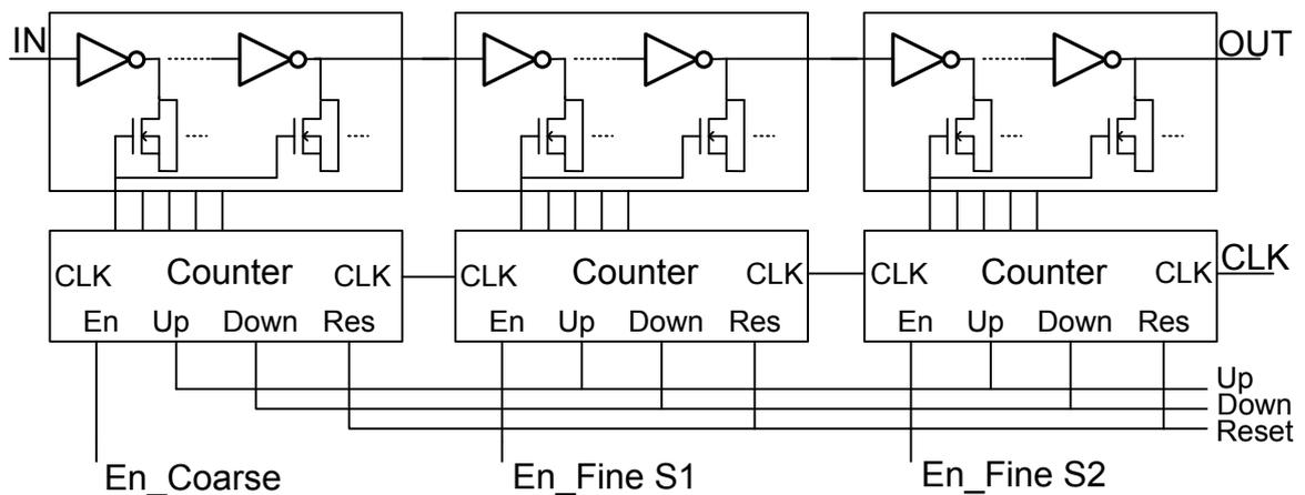
Figure 5.46. Configurable delay line architecture.
