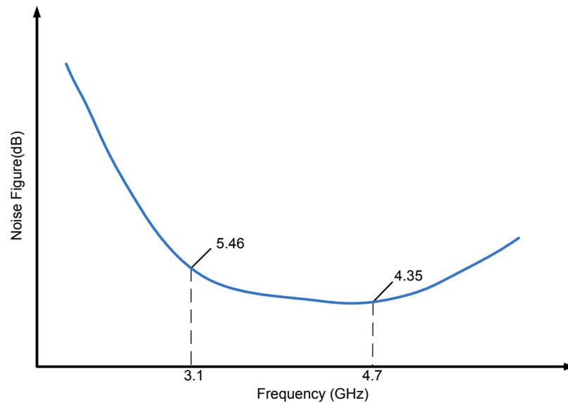
Figure 5.6. LNA noise figure layout simulation.
