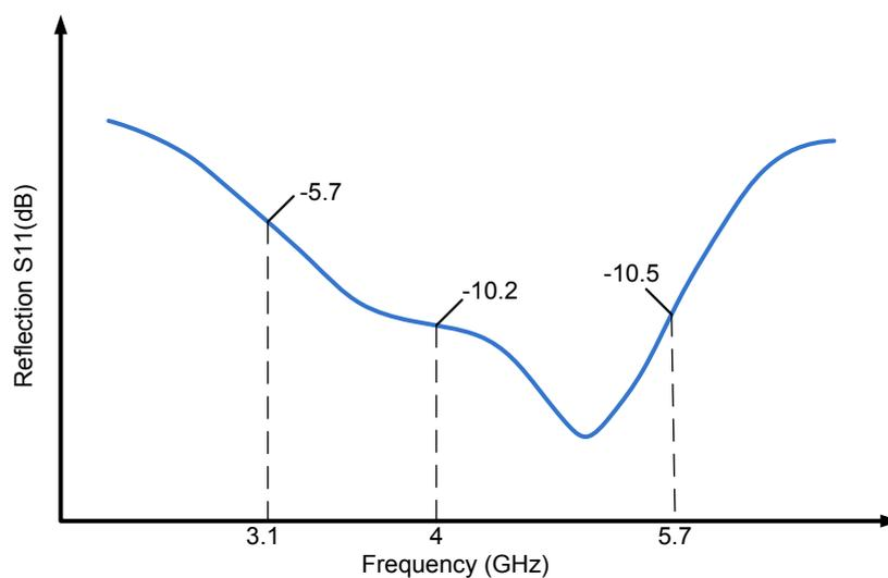
Figure 5.7. LNA input reflection schematic simulation.
