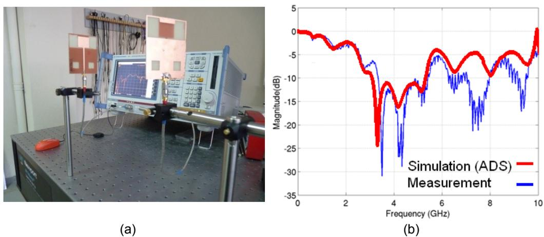
Figure 6.5. Proposed antenna; (a) Measurement setup (b) Simulation and measurement results.
