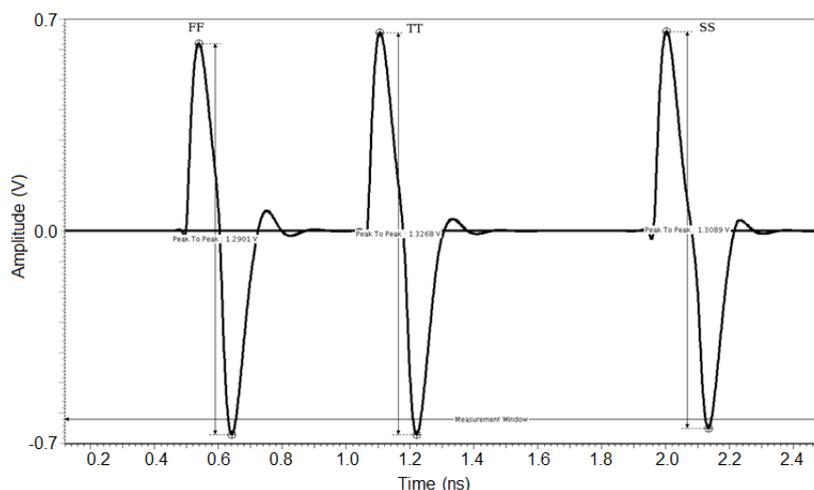
Figure 4.20. Time domain simulation of process variations.
