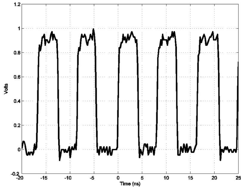
Figure 5.19. 120 MHz clock reception measurement result.
