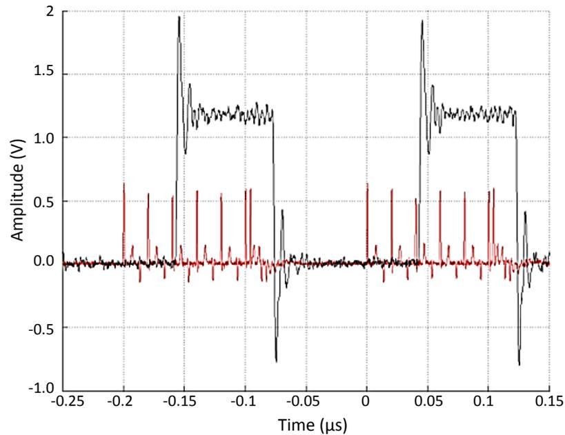
Figure 5.29. Self correlator measurements at 10 Mbps.
