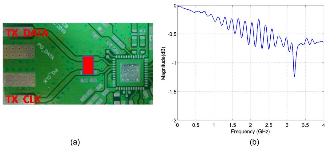
Figure 6.14. (a) Test setup of the short connected traces . (b) Total insertion loss of the short connected traces.
