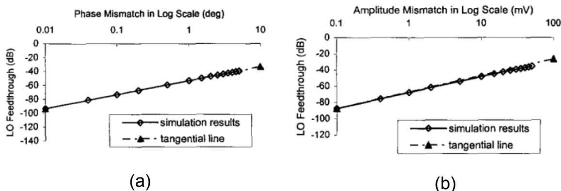
Figure 5.39. (a) Phase mismatch, (b) Amplitude mismatch in a mixer [1].
