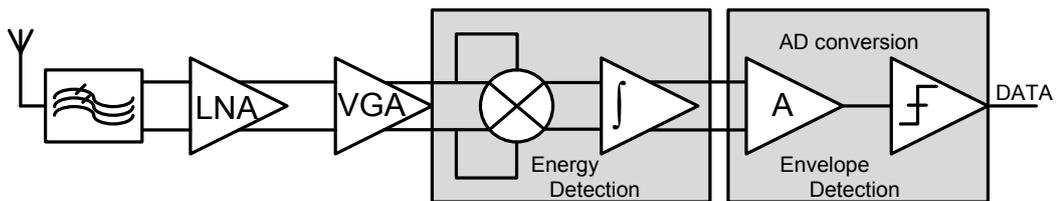
Figure 1.2. Energy Detection IR-UWB receiver.
