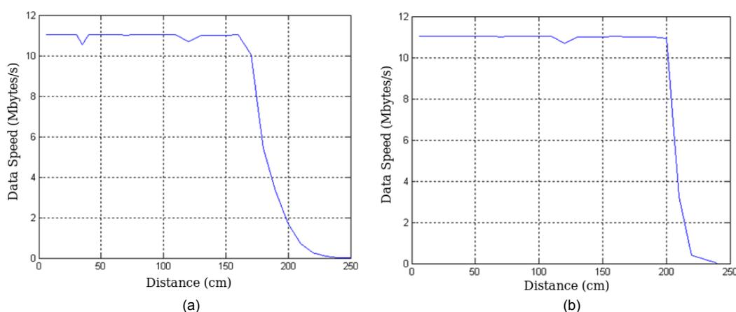
Figure 7.3. Performance of Wisair Board; (a) 480 Mbps mode, (b) 400 Mbps mode.
