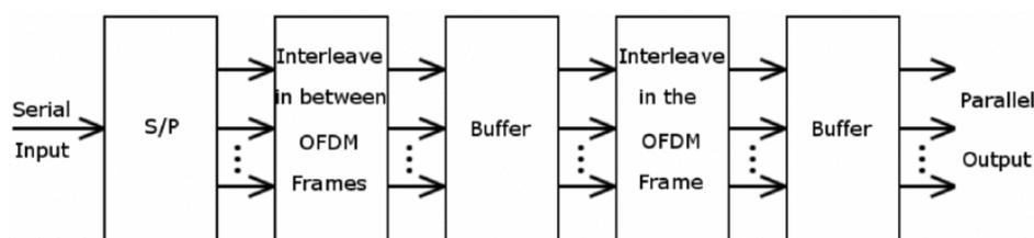
Figure 3.4. Interleaver block diagram.
