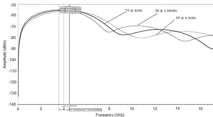
Figure 4.21. Frequency domain simulation of process variations.
