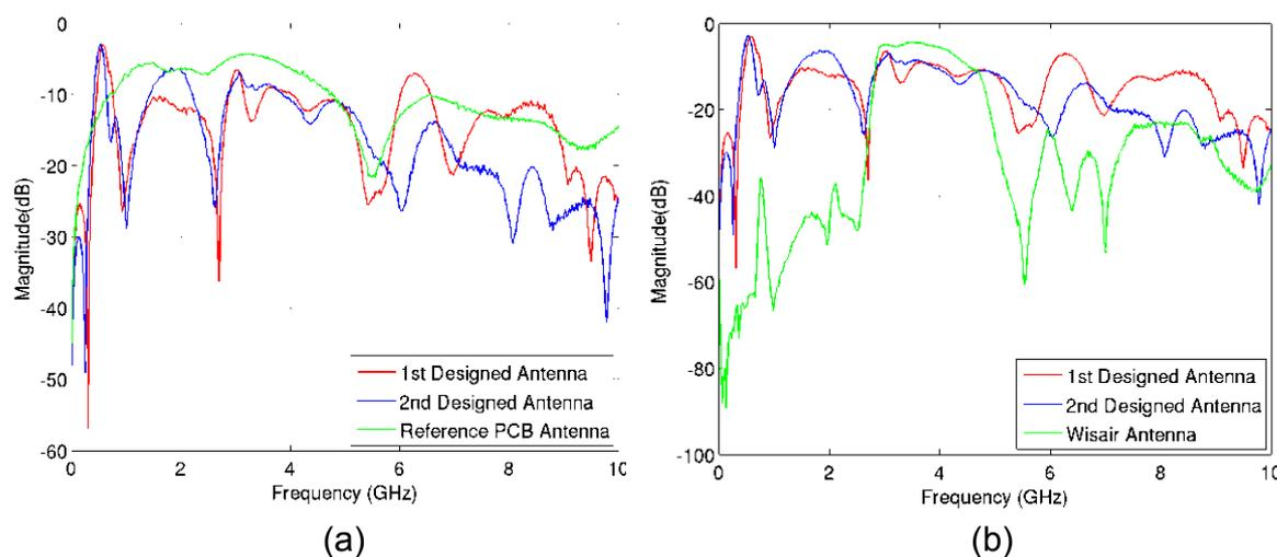
Figure 6.7. S21 comparisons for 1cm distance (a) designed antennas vs. reference antenna (b) designed antennas vs. commercial antenna.
