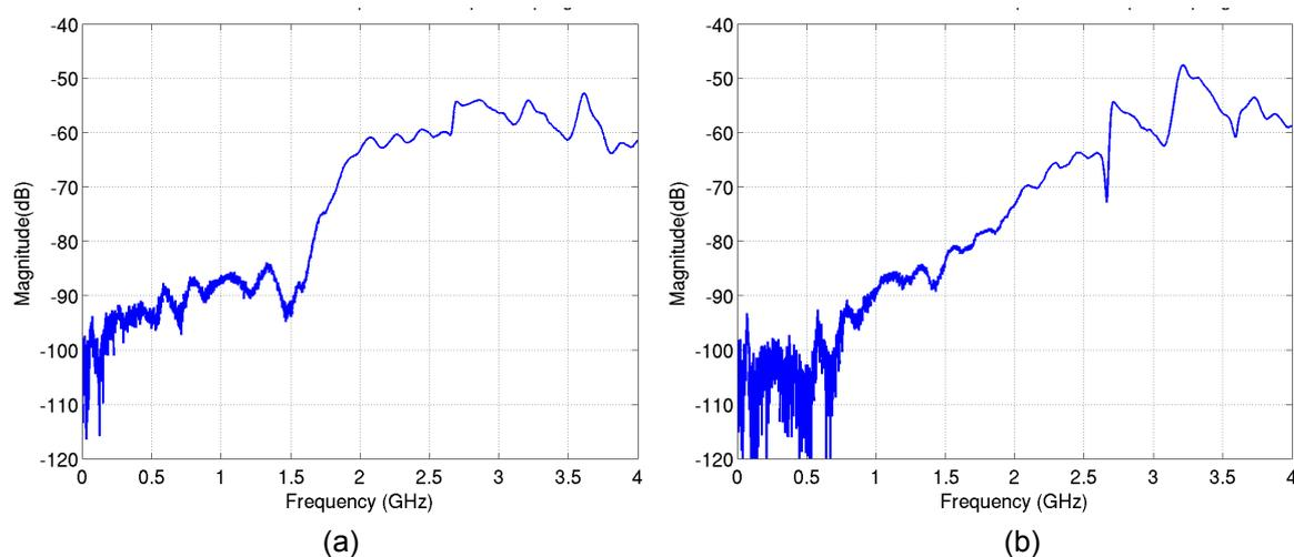
Figure 6.12. Measurements; (a) Coupling between TX DATA and LNA IN. (b) Coupling between TX CLK and LNA IN.
