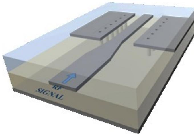
Figure 6.10. Coplanar waveguide.
