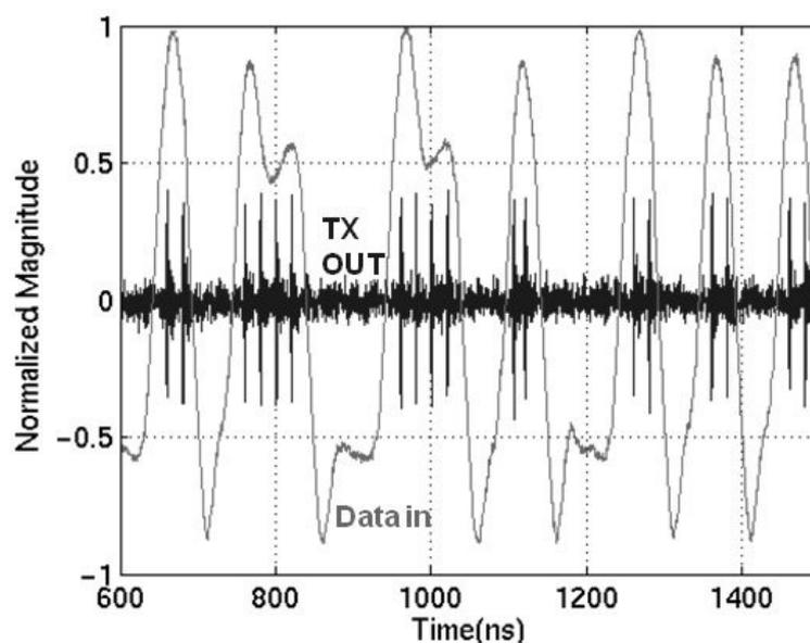
Figure 5.21. Ethernet signal and transmitter output.
