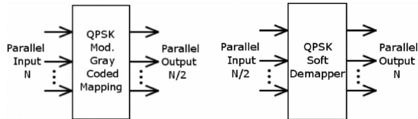
Figure 3.5. QPSK modulator/demodulator block definitions.
