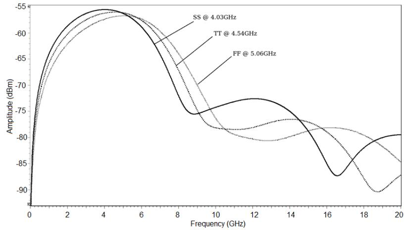
Figure 4.22. Frequency domain simulation of process variations.
