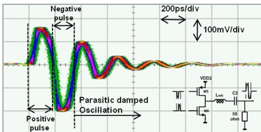
Figure 4.11. Transmitter output with pulse-shaping capacitor.
