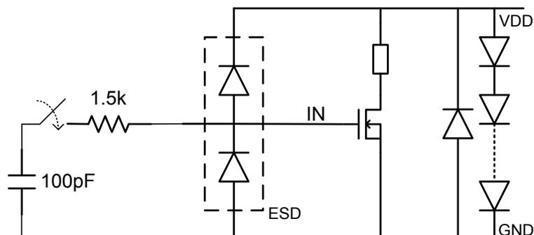
Figure 5.59. ESD test circuit.
