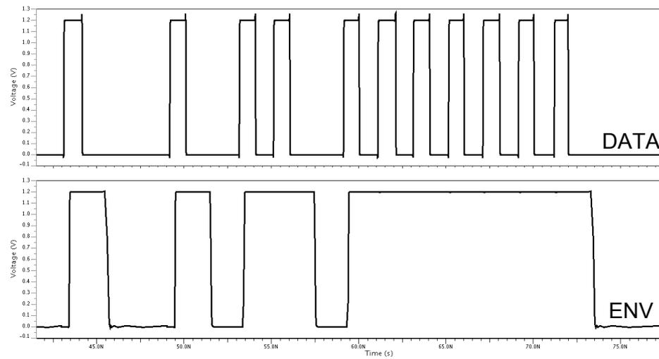
Figure 5.25. Envelope detector simulations.
