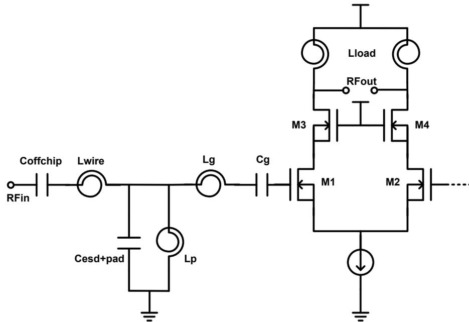
Figure 5.4. Cascode LNA schematic with matching network.
