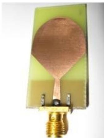
Figure 6.1. The fabricated reference antenna.
