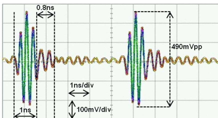
Figure 4.12. Transmitter output with BPF.
