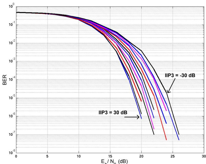
Figure 3.14. Effect of LNA linearity on BER performance.
