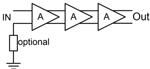
Figure 5.40. Active balun block diagram.
