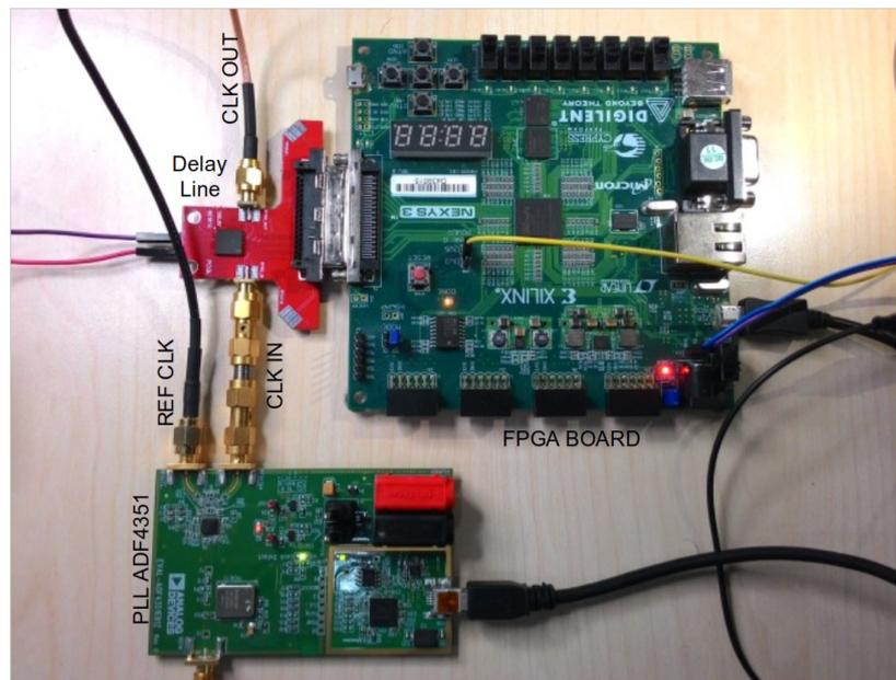
Figure 5.48. Measurement setup.
