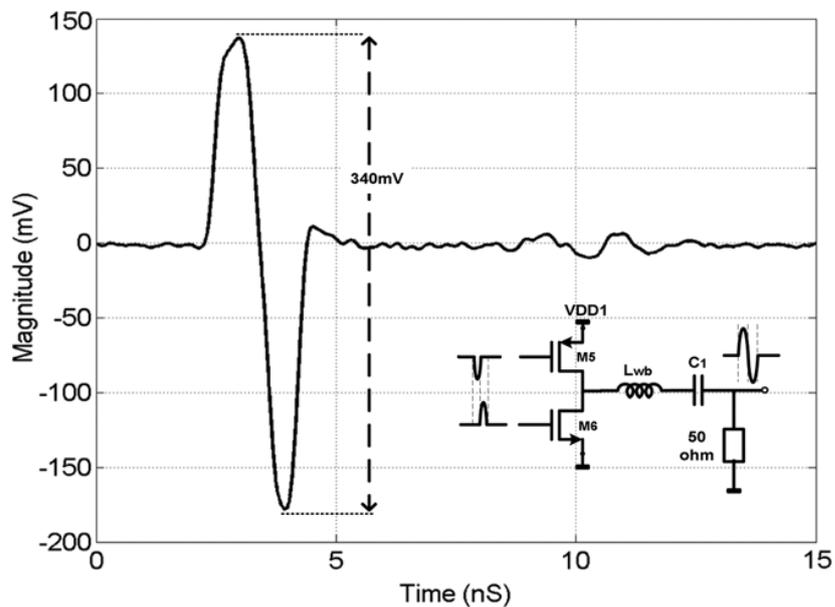
Figure 4.8. Transmitter output with a pulse-shaping capacitor.
