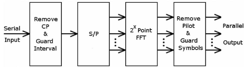
Figure 3.7. OFDM demodulator block diagram.
