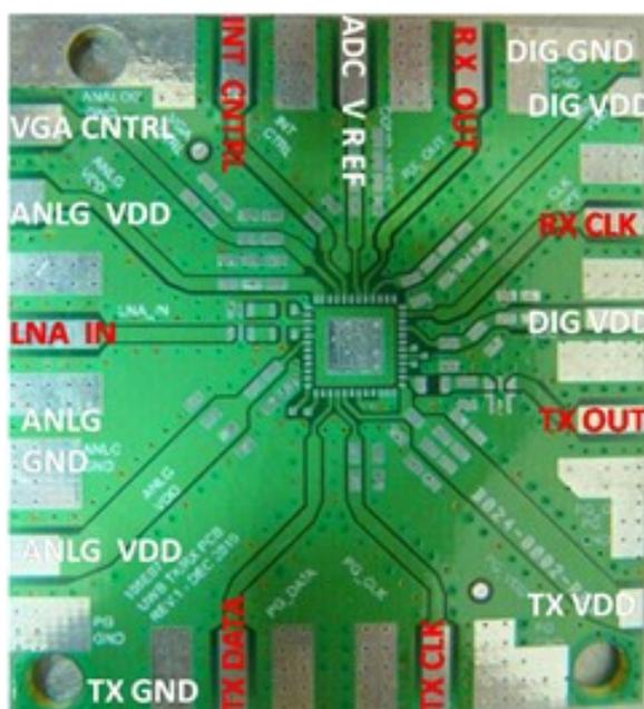
Figure 6.11. Non-coherent transceiver PCB design.
