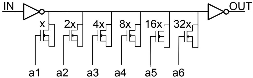
Figure 4.18. Configurable delay cell.
