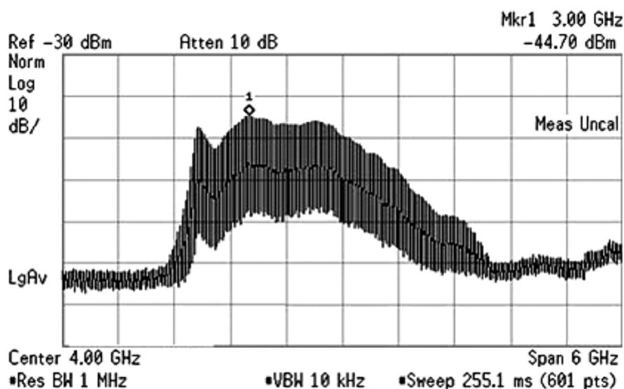
Figure 4.13. Output spectrum in the upper band at 10 MHz PRF.
