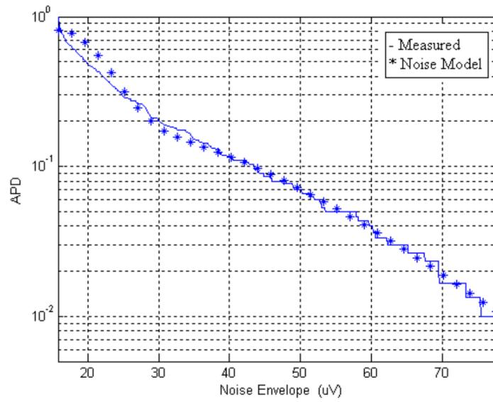
Figure 2.6. APD of Figure 2.2 and noise model fit.
