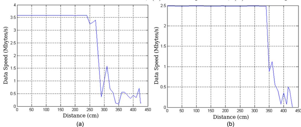
Figure 7.6. Performance of Wisair Board; (a) 160 Mbps mode, (b) 106.7 Mbps mode.
