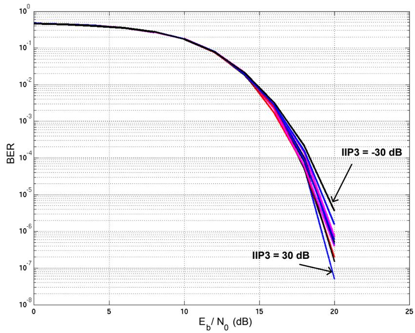
Figure 3.15. Effect of squarer linearity on BER performance.
