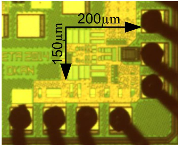
Figure 4.24. Transmitter micrograph.
