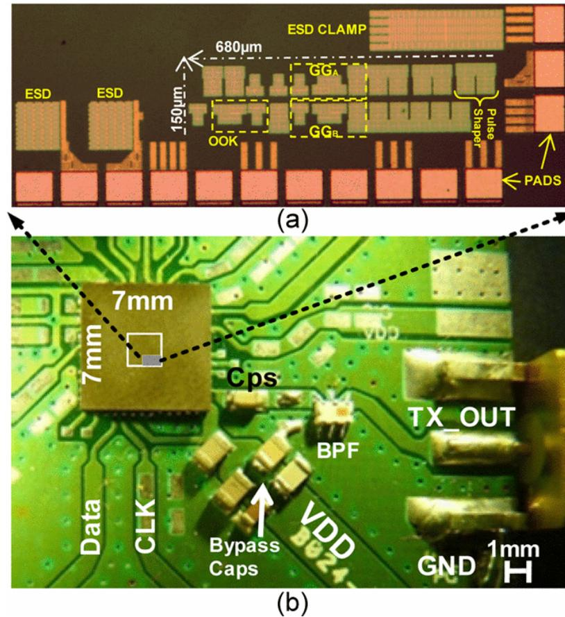
Figure 4.7. (a) Micrograph of the UWB transmitter in a UMC 130-nm process. (b) Picture of the RF FR-4 PCB and components used in the measurements.
