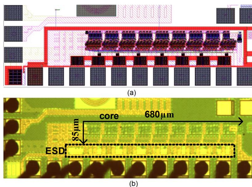
Figure 5.47. Delay line (a) layout design, and (b) micrograph.
