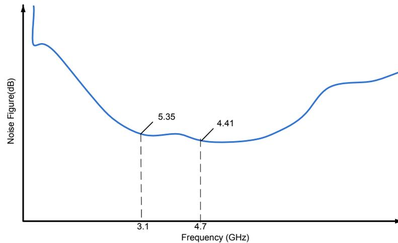
Figure 5.5. LNA noise figure circuit simulation.
