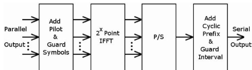
Figure 3.6. OFDM modulator block diagram.
