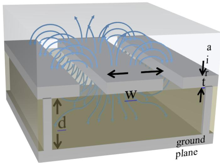
Figure 6.9. Coplanar waveguide.
