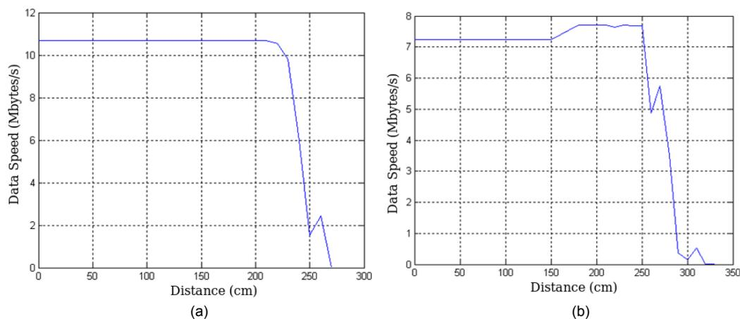
Figure 7.4. Performance of Wisair Board; (a) 320 Mbps mode, (b) 200 Mbps mode.
