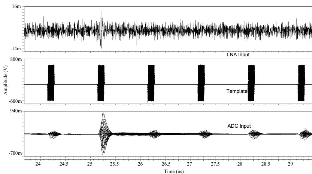
Figure 5.55. Template correlation simulations under noisy channel.
