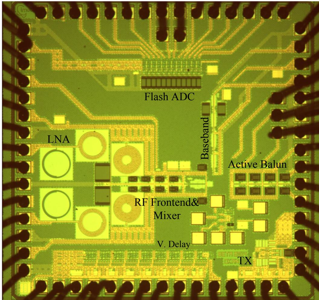
Figure 5.35. Coherent receiver micrograph.
