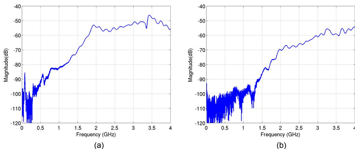
Figure 6.13. Measurements; (a) Coupling between RX OUT and LNA IN. (b) Coupling between TX OUT and LNA IN.
