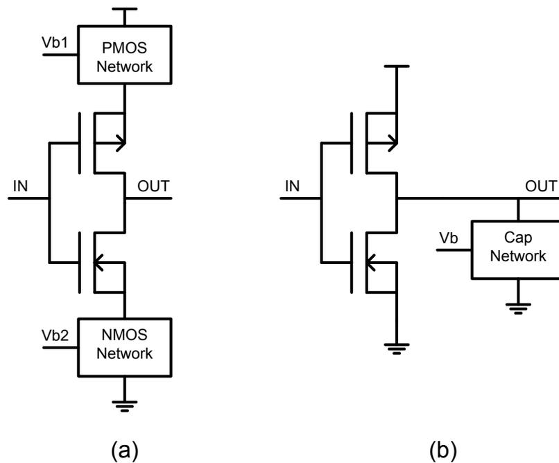
Figure 5.43. Delay cells (a) Current steering, and (b) Shunt capacitor methods.
