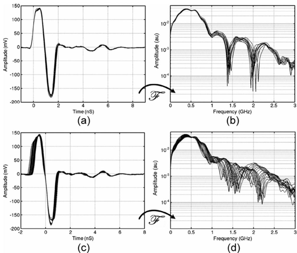
Figure 4.10. Output variation in time domain of (a) 11 chip samples (c) from  $-20\text{ }^{\circ}\text{C}$  to  $70\text{ }^{\circ}\text{C}$  at  $5\text{ }^{\circ}\text{C}$  steps. Output variation in the frequency domain of (b) 11 chip samples (d) from  $-20\text{ }^{\circ}\text{C}$  to  $70\text{ }^{\circ}\text{C}$  at  $5\text{ }^{\circ}\text{C}$  steps.
