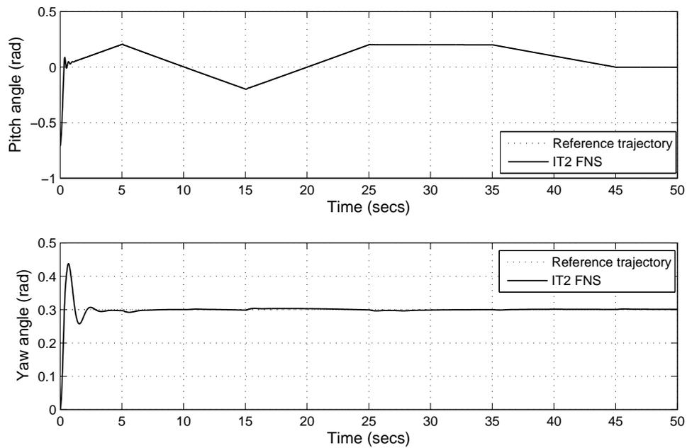
Figure 7.20. First simulation study, changing reference trajectory for the pitch axis and step reference trajectory for the yaw axis of a 2-DOF helicopter.
