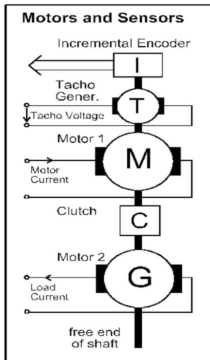
Figure 7.8. Block scheme of the plant.
