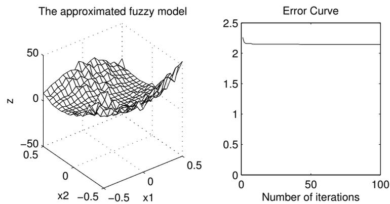
Figure 4.12. The result of Rosenbrock's Banana function approximation by using type-1 fuzzy algorithm (a) and the RMSE curve obtained by tuning the parameters of the parameterized conjunctive operators (b).
