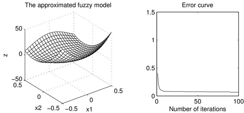
Figure 4.5. The result of Rosenbrock's Banana function approximation by using type-1 fuzzy algorithm (a) and the RMSE curve obtained by tuning the parameters of the parameterized conjunctive operators (b).
