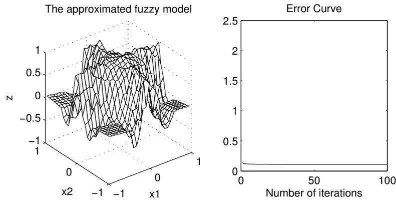
Figure 4.11. The result of Sinc function approximation by using type-1 fuzzy algorithm (a) and the RMSE curve obtained by tuning the parameters of the parameterized conjunctive operators (b).
