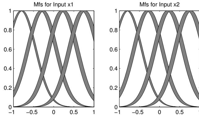
Figure 4.6. The input membership functions obtained by using IT2-FCM algorithm for Sinc function approximation without noise.
