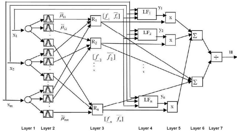
Figure 6.1. The structure of a Type-2 FNS.
