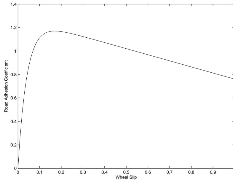
Figure 6.7. Road adhesion coefficient vs. wheel slip.
