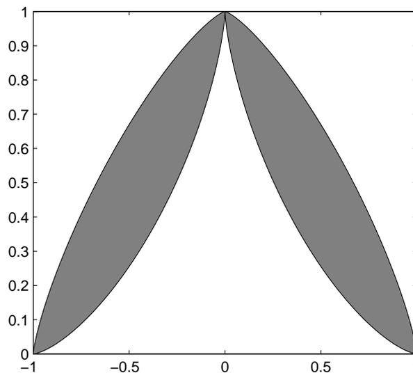
Figure 7.18. Interval type-2 elliptical membership function.
