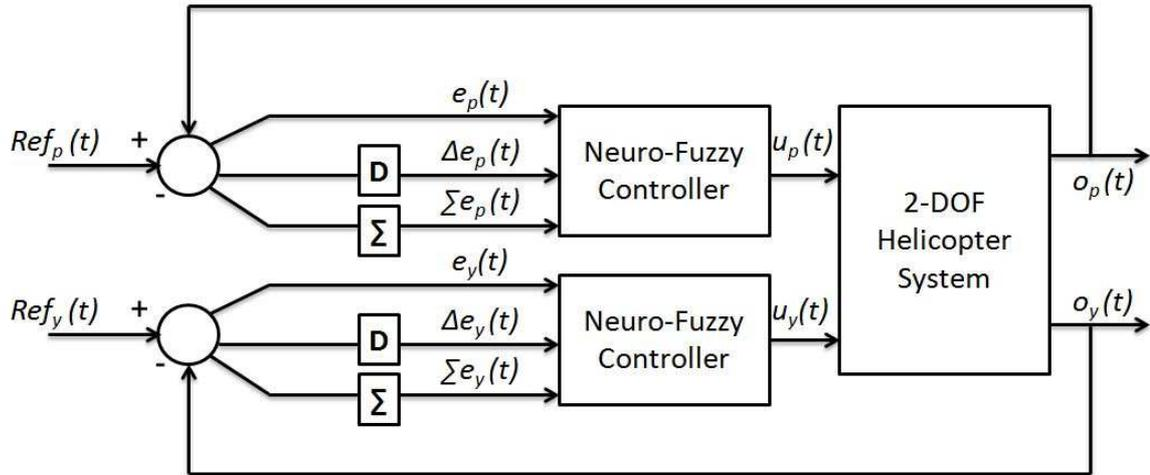
Figure 7.3. Block diagram of the neuro-fuzzy control system.
