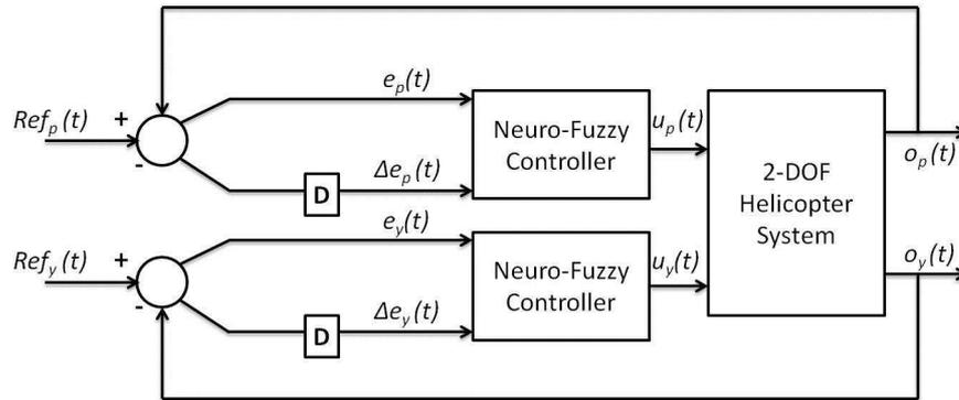
Figure 7.19. The block diagram of the system.
