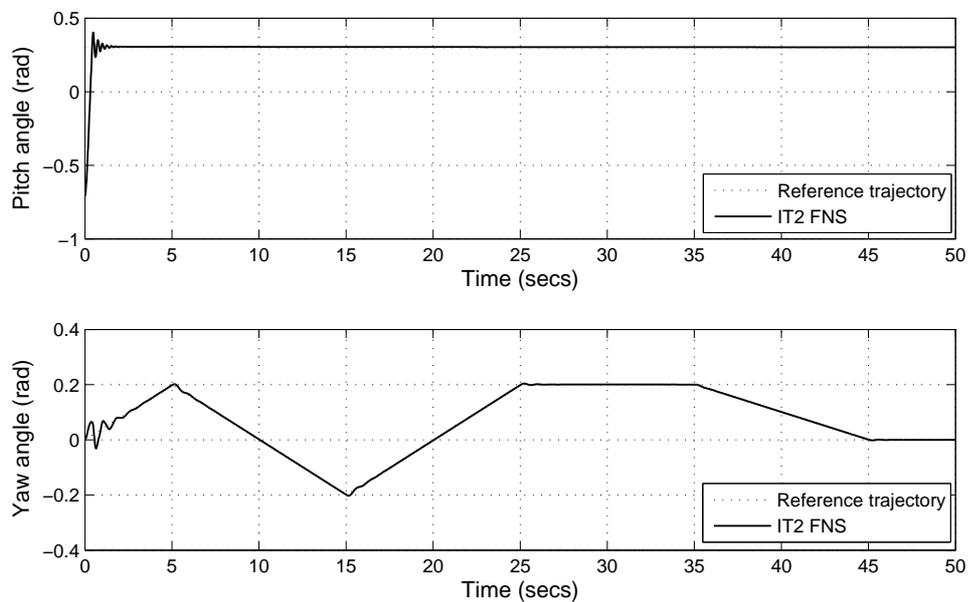
Figure 7.21. Second simulation study, step reference trajectory for the pitch axis and changing reference trajectory for the yaw axis of a 2-DOF helicopter.
