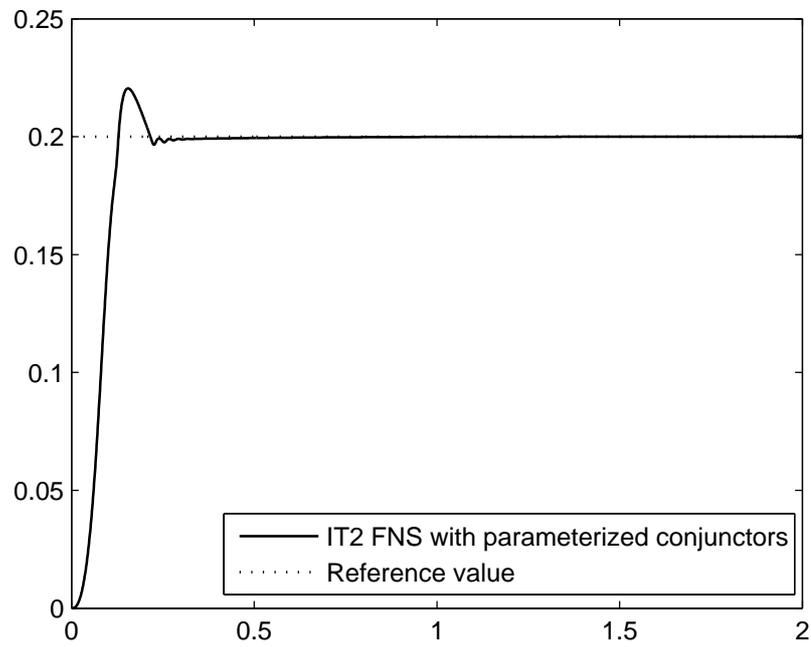
Figure 6.9. Wheel slip of type-2 FNS with parameterized conjunctors.
