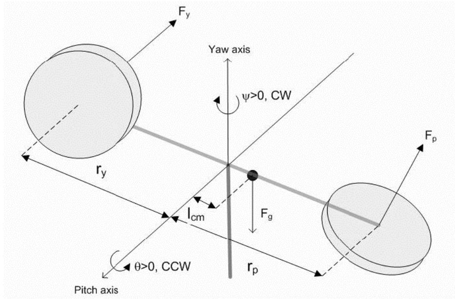
Figure 7.2. Simple free body diagram of 2-DOF helicopter [66].
