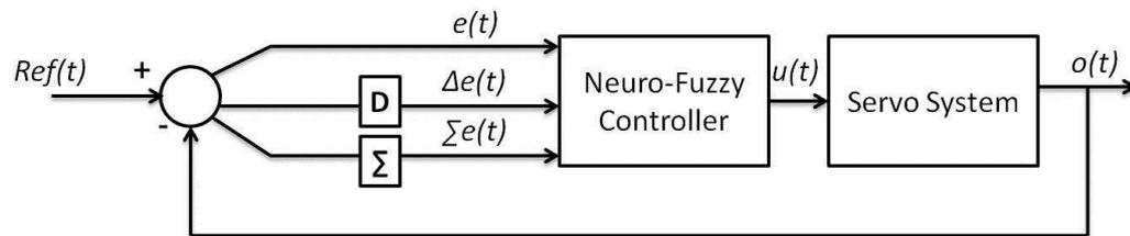
Figure 7.10. Block diagram of the neuro-fuzzy control system.
