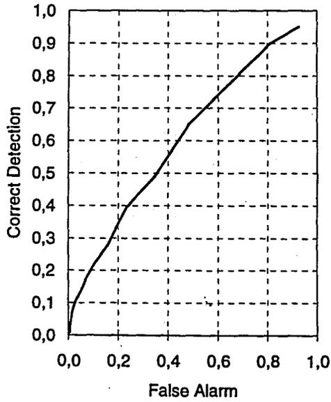
FIGURE 3.9. Average SOC curve for WPS based system.
