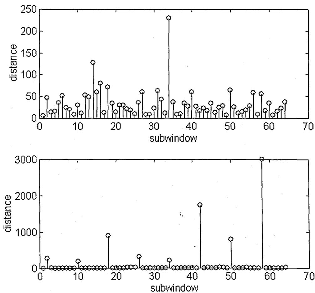
FIGURE 3.24. Distance ( $d_i$ ) values for the subwindows ( $i$ ) of defective textile fabric image 'dc17' obtained using SDCM (top) and SBCM methods (bottom).
