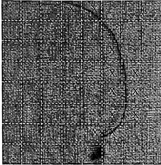
FIGURE 3.2. A defective textile fabric image and its partitioning. 'X' denotes defective subwindows as labeled by a quality inspector.
