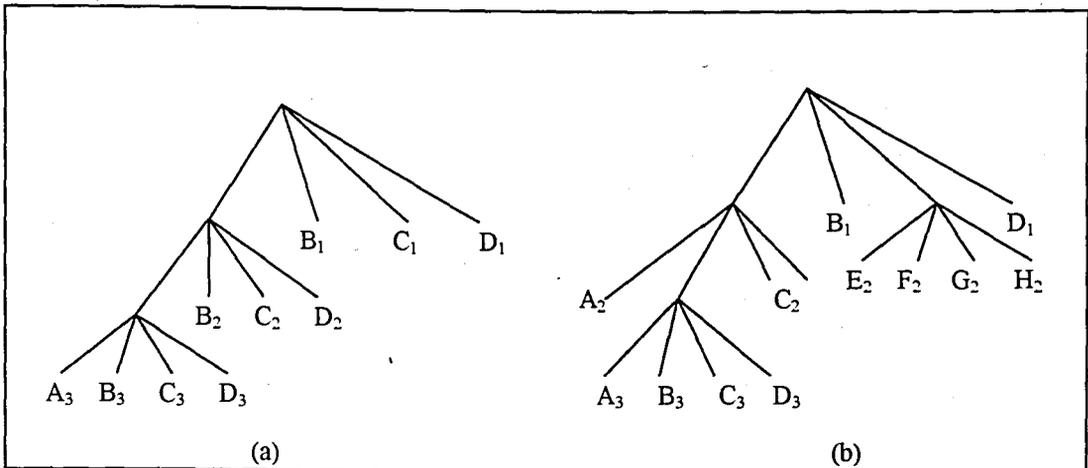
FIGURE 3.3. Pyramid-structured (a) and tree-structured (b) wavelet decomposition.
