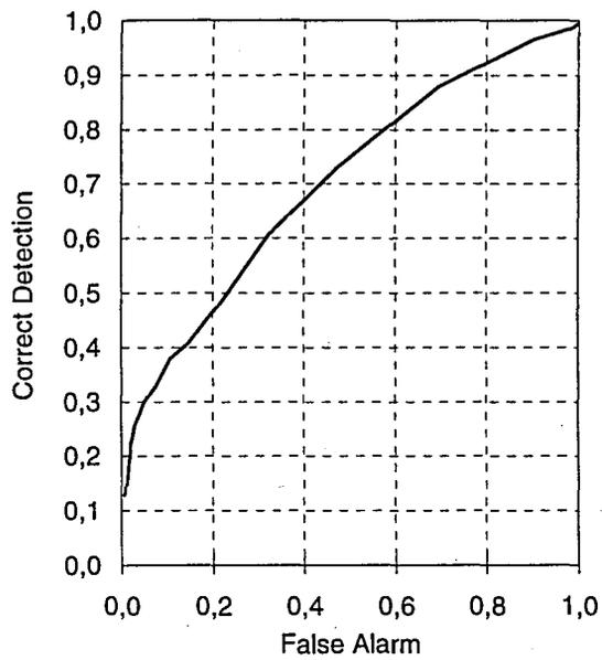
FIGURE 3.17. Average SOC curve for SDCM based system.
