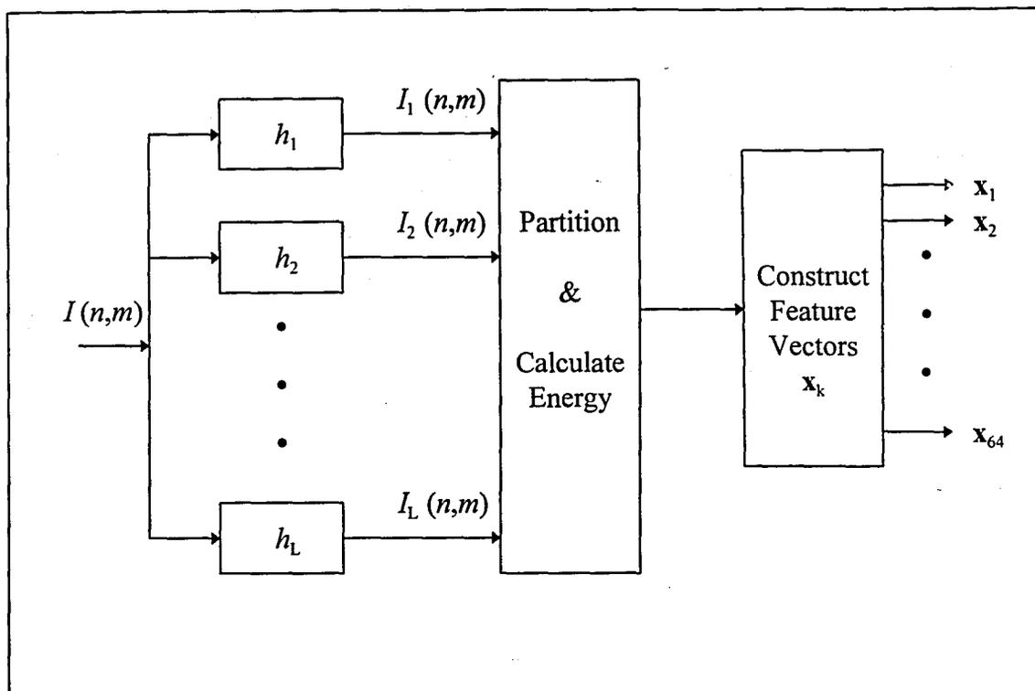
FIGURE 3.11. Multichannel feature extraction
