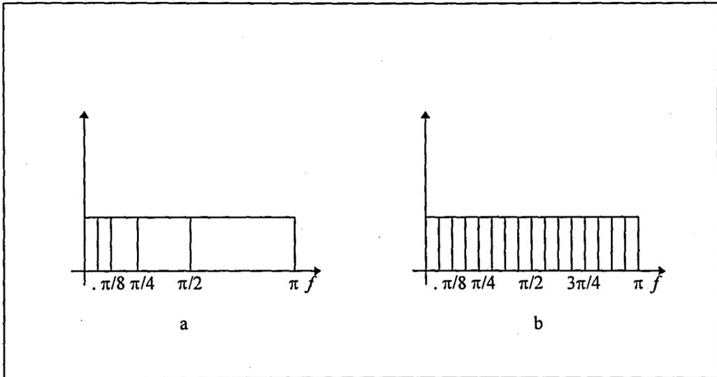
FIGURE 2.3. Split of frequency band for 4-level decomposition with (a) Pyramid structured wavelet transform and (b) wavelet packet bases.
