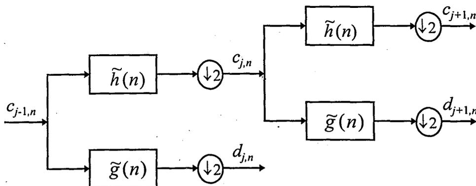
FIGURE 2.2. Two-level wavelet decomposition scheme
