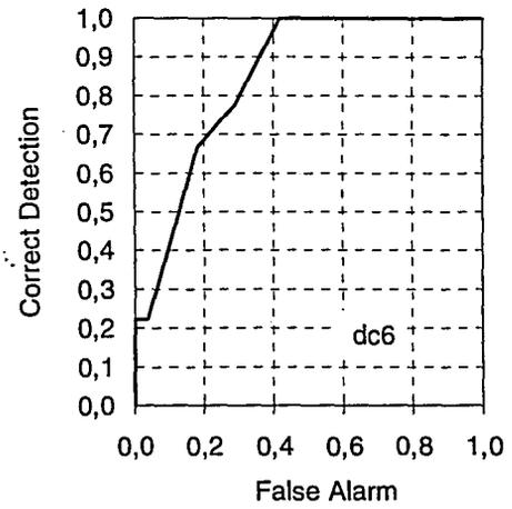
FIGURE 3.15. SOC curves for Gabor based system under each defect type.
