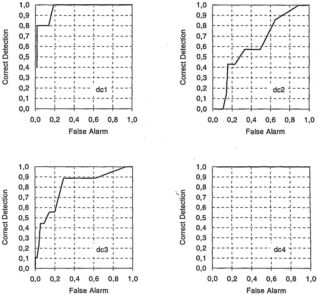
FIGURE 3.21. SOC curves for SBCM based system under each defect type.
