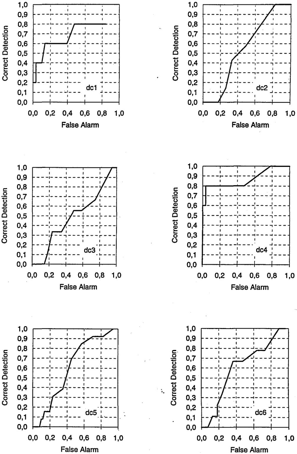
FIGURE 3.10. SOC curves for WPS based system under each defect type.
