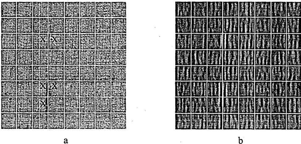
FIGURE 3.12. (a) Defective fabric image 'dc1' and (b) the feature image obtained by Gabor filtering with filter parameters  $(B, \Omega, F, \theta) = (1, \pi/4, 32, 0)$ . 'X' shows defective blocks.
