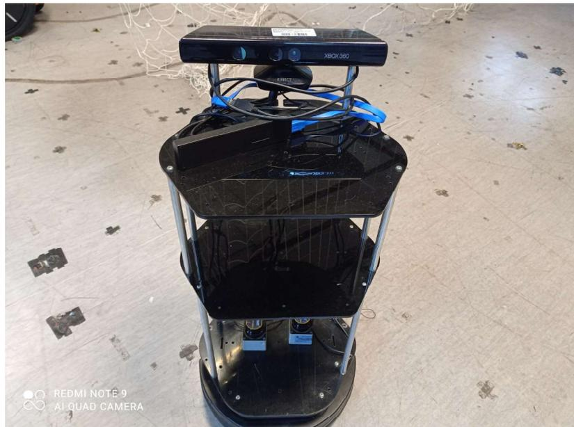
Figure A.1. Turtlebot Robot Used in the Experiments.
