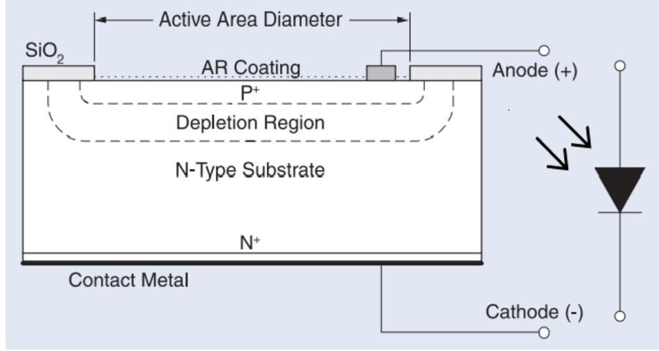
Figure 2.4. Planar diffused silicon photodiode [3].
