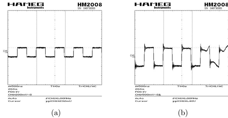
Figure 3.28. (a) Square wave input of the TIA at 1 MHz, (b) Output response of the TIA at 1 MHz.
