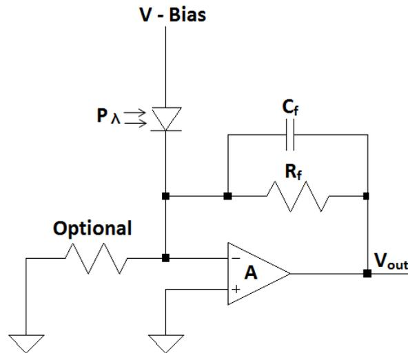
Figure 2.7. Circuit for photoconductive operation [4]
