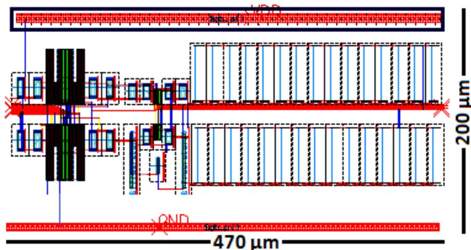
Figure 4.18. Layout of receiver circuit.
