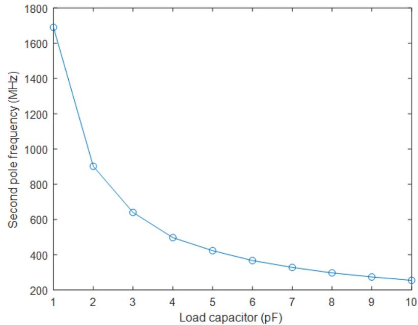
Figure 4.15. Load capacitance versus second pole frequency.
