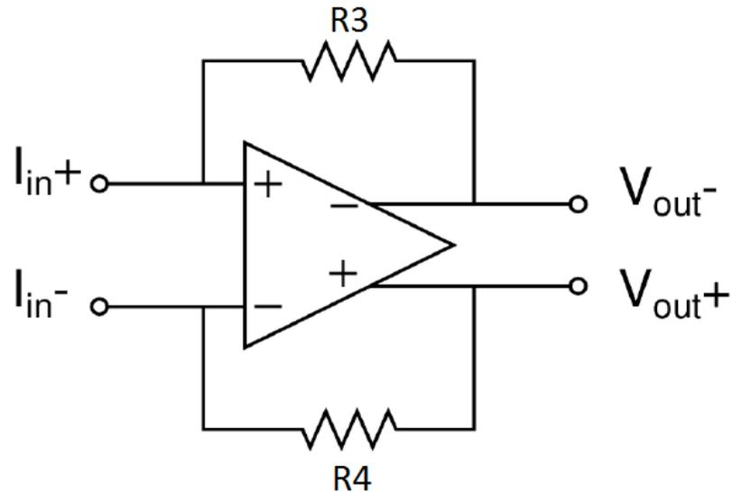
Figure 4.4. Schematic of CMOS TIA circuit (block diagram).
