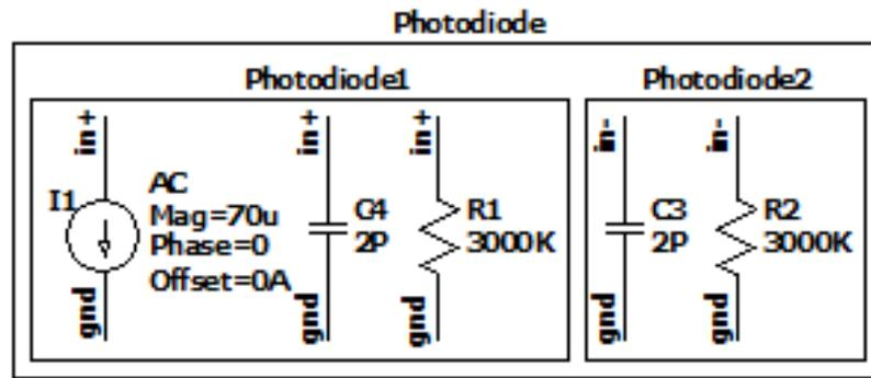
Figure 4.19. Photodiode Testbench.
