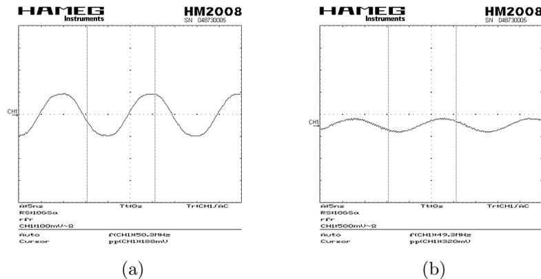
Figure 3.29. (a) Square wave input of the TIA at 50 MHz, (b) Output response of the TIA at 50 MHz.
