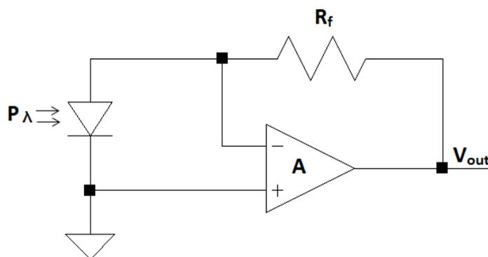
Figure 2.6. Circuit for zero bias operation [4]
