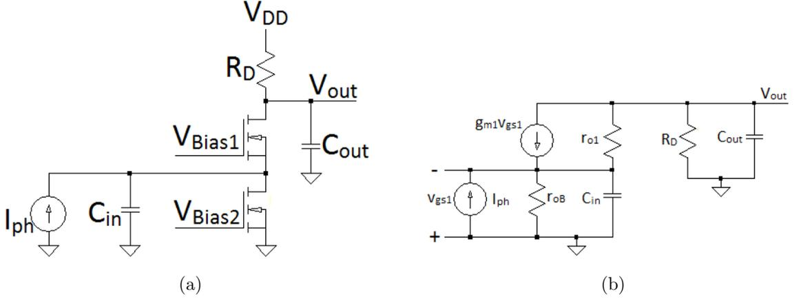
Figure 2.12. (a) CG-TIA circuitry, (b) Small-signal model of CG-TIA [5], [6].
