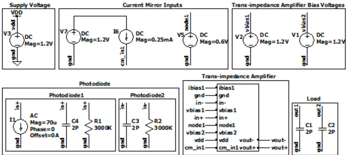
Figure 4.26. Test bench of the Equalizer for the AC simulation
