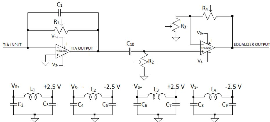
Figure 3.5. Circuit schematic of the Discrete Receiver System.
