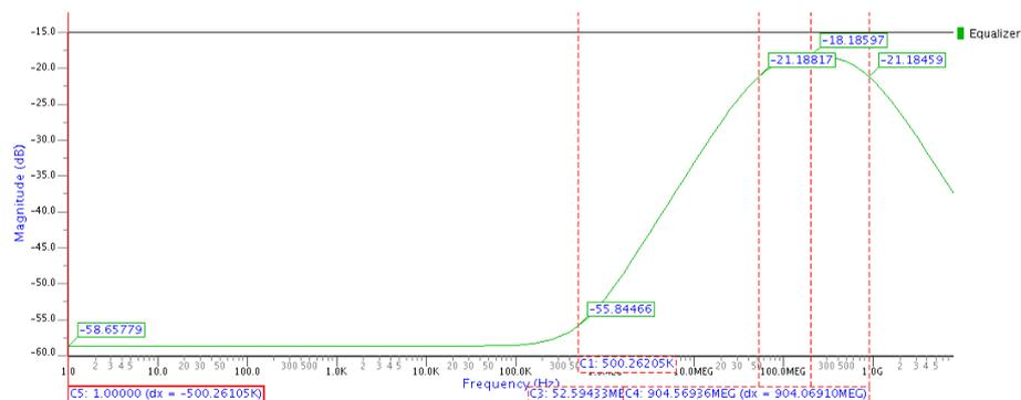
Figure 4.27. AC simulation result of the Equalizer.
