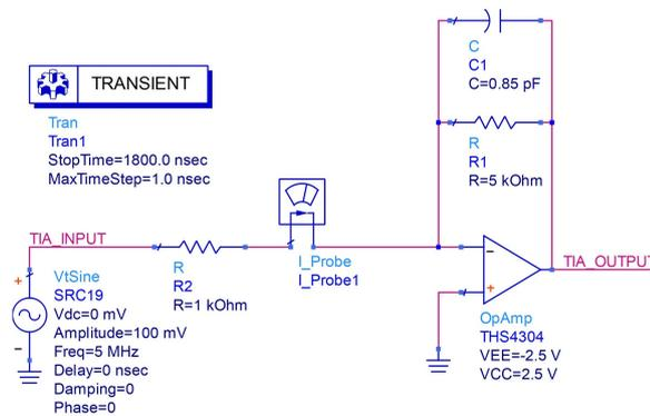
Figure 3.11. Circuit Schematic of the TIA for transient simulation.
