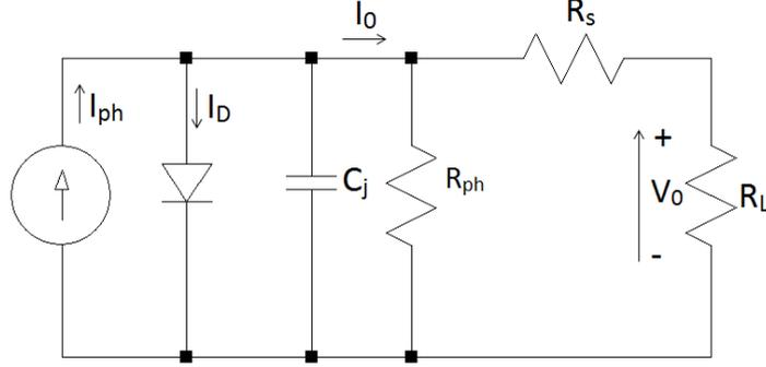
Figure 2.3. Equivalent circuit for a silicon photodiode [3].
