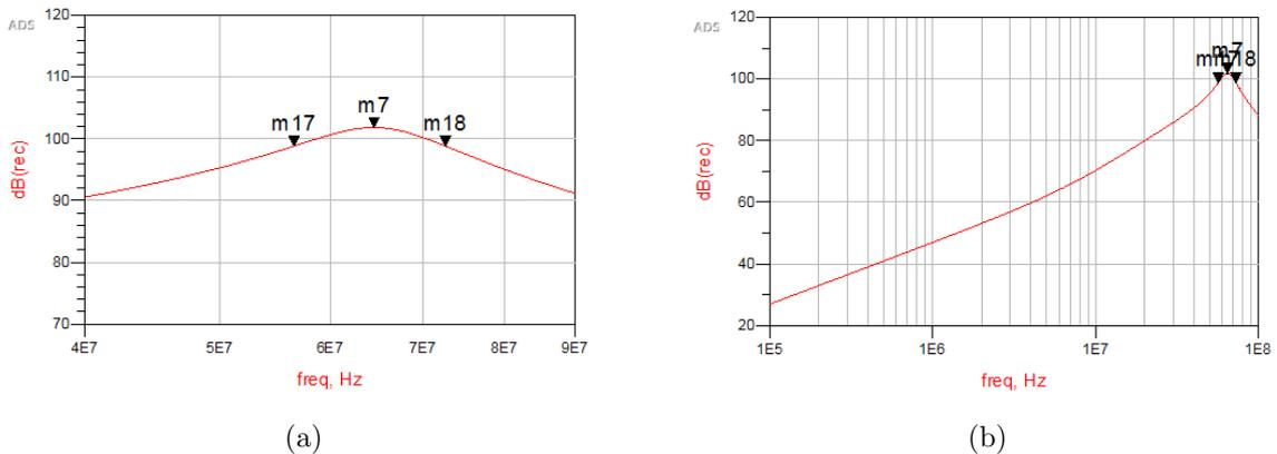
Figure 3.18. (a) Frequency response of the Discrete Receiver System (zoomed in), (b) Frequency response of the Discrete Receiver System (fully viewed).
