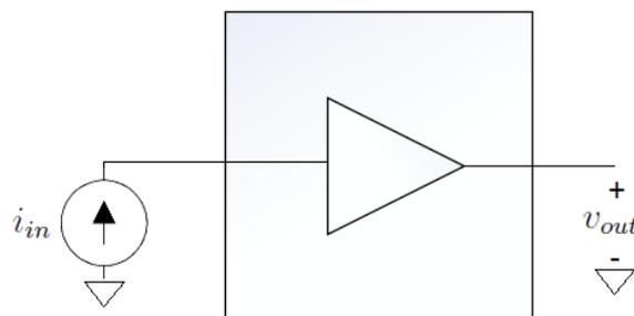
Figure 2.9. Trans-impedance amplifier.
