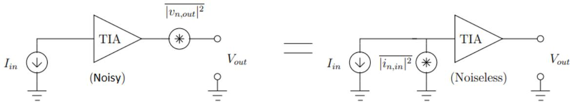
Figure 2.10. Input referred noise current.
