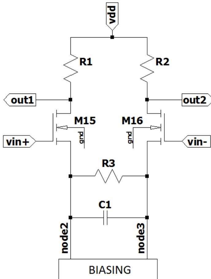
Figure 4.8. Schematic of Equalizer circuit.
