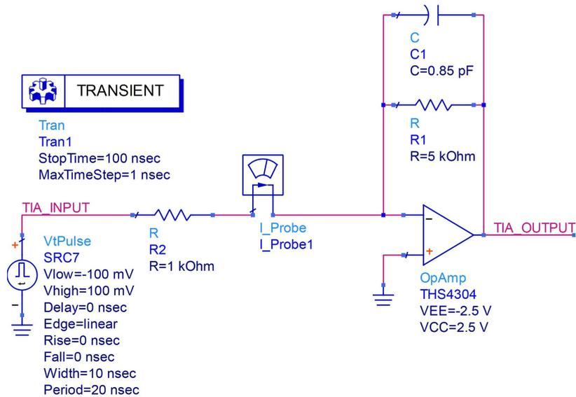
Figure 3.13. Circuit Schematic of the TIA for Transient simulation.
