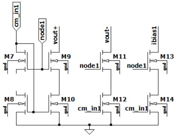
Figure 4.5. Schematic of low voltage current mirror.
