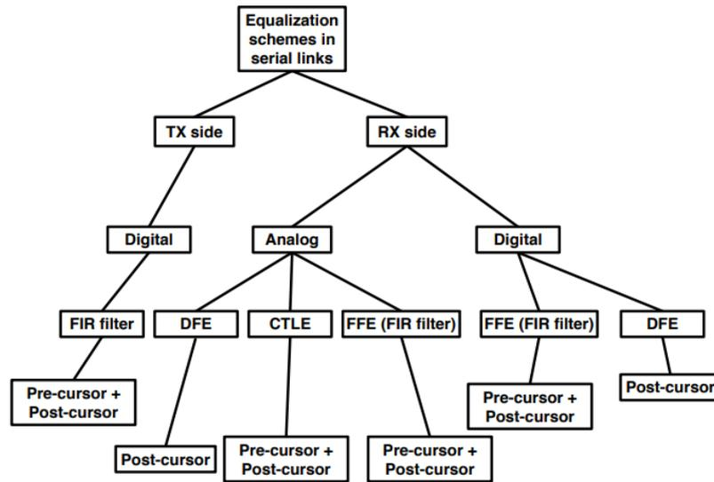
Figure 2.15. Equalizer methods utilized in high speed links [2]
