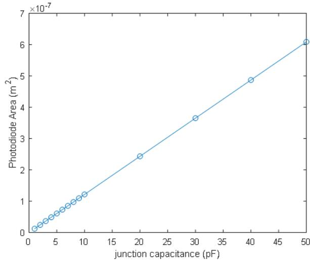
Figure 4.1. Photodiode junction capacitance versus photodiode area.
