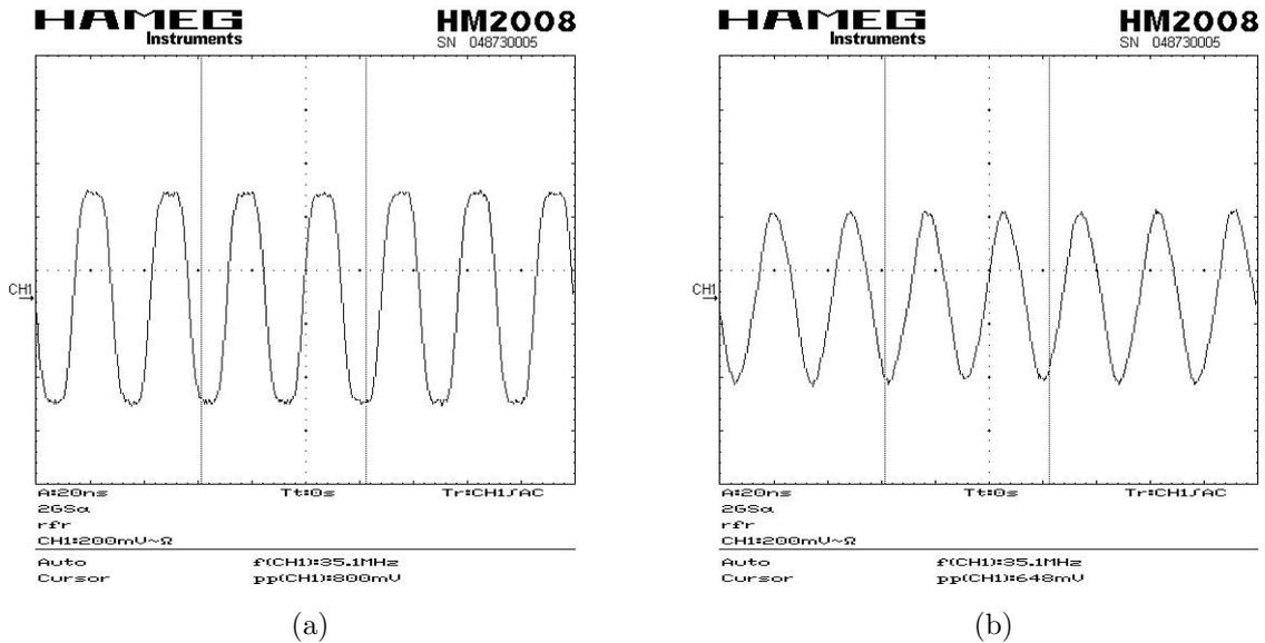
Figure 3.33. (a) Square wave input of the Discrete Receiver System at 35 MHz, (b) Output response of the Discrete Receiver System at 35 MHz.
