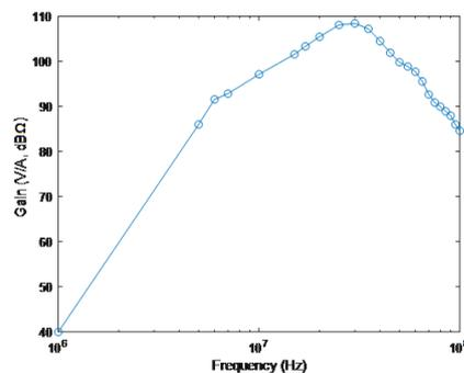
Figure 3.30. Frequency Response of the Discrete Receiver System.
