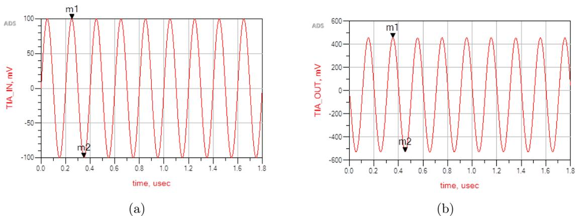
Figure 3.12. (a) Sinusoidal input at 5 MHz, (b) Sinusoidal output of the TIA at 5 MHz.
