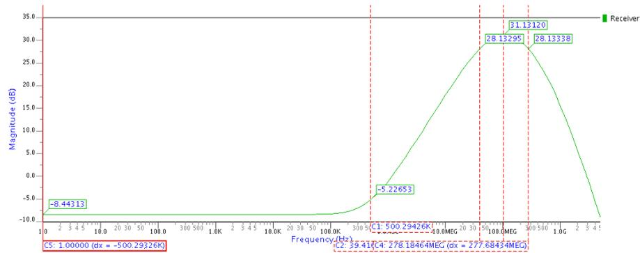
Figure 4.32. AC simulation result of the CMOS Receiver System using 2 pF photodiode capacitance.
