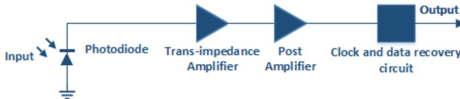
Figure 1.2. Architecture of a typical optical receiver [1].
