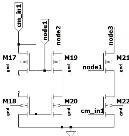
Figure 4.9. Schematic of low voltage current mirror.
