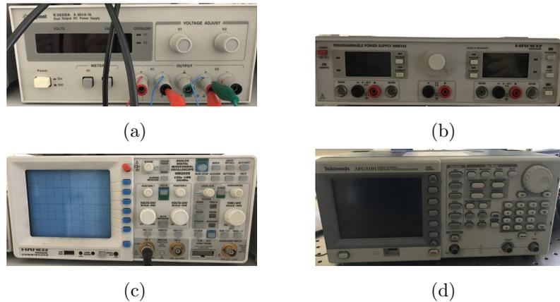
Figure 3.25. (a) DC Power Supply, (b) Programmable Power Supply, (c) HAMEG Oscilloscope, (d) Function Generator.
