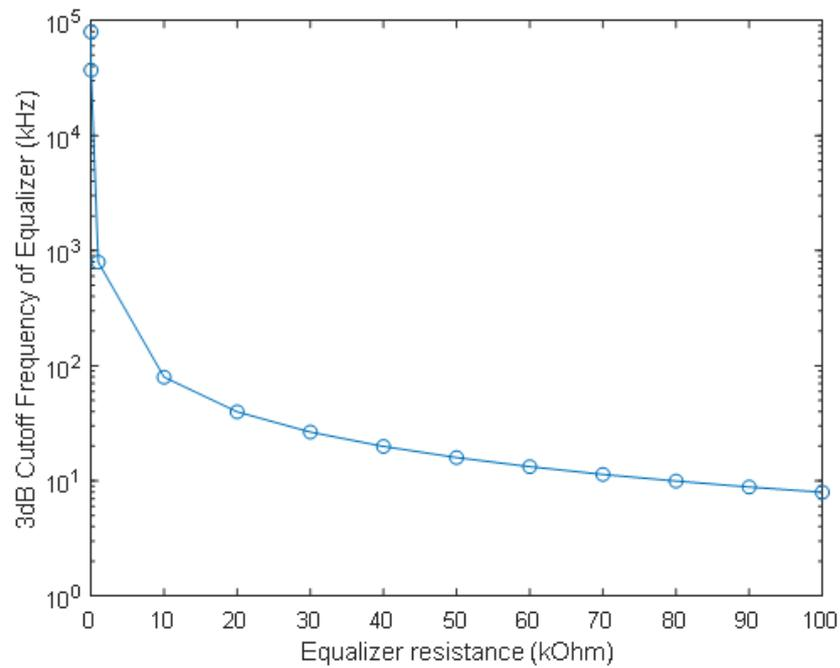
Figure 3.7. Equalizer resistance versus 3-dB Cutoff frequency.
