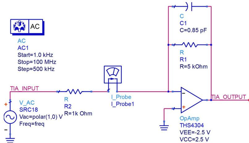
Figure 3.9. Circuit schematic of the TIA for AC simulation.
