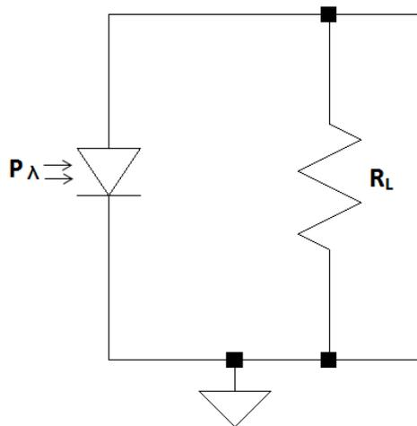
Figure 2.5. Circuit for photovoltaic operation [4].
