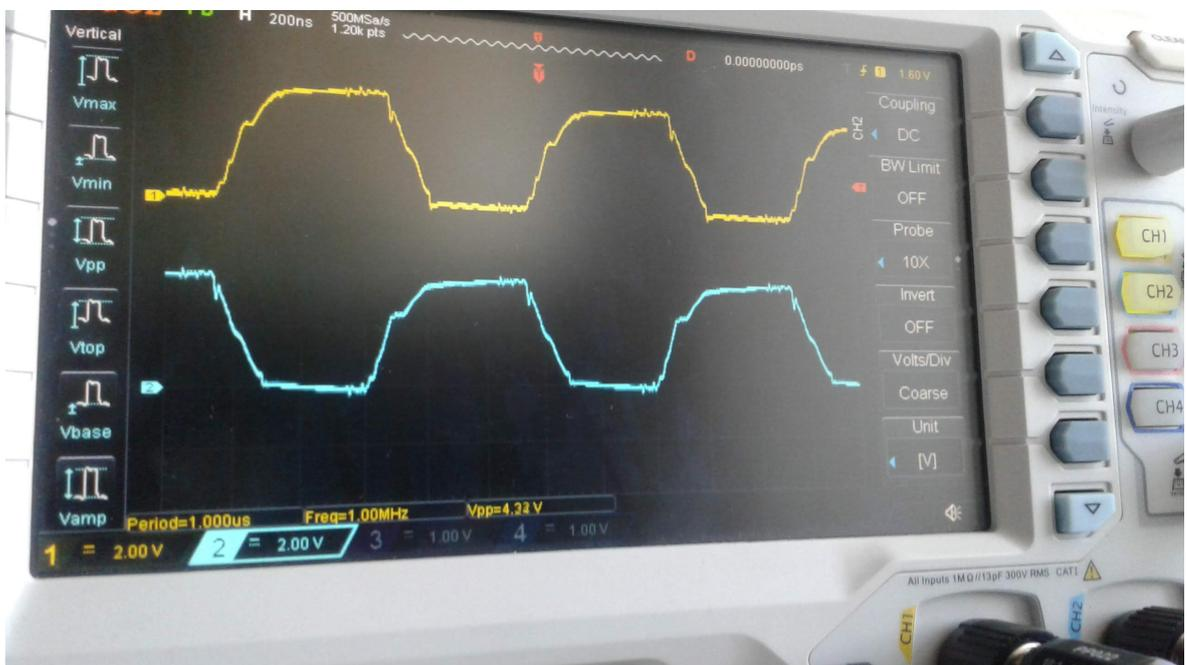
Figure 3.23. Transceiver PCB transmission switching gate driving signal
