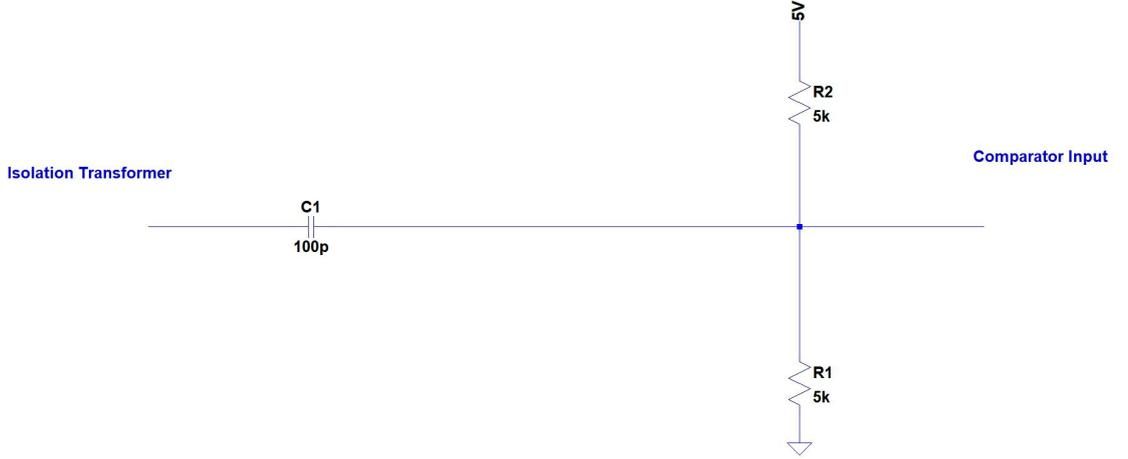
Figure 2.6. Receiver input filter and level shifter for PCB, LTSpice
