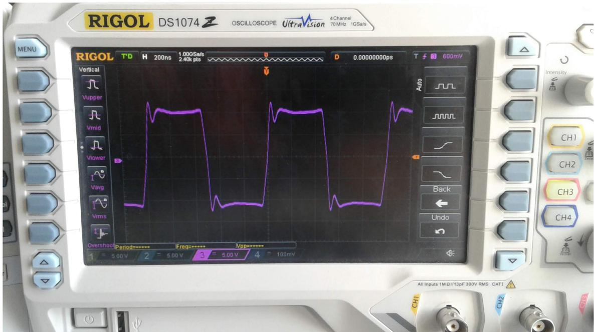
Figure 3.22. Transceiver PCB transmission signal on the terminal, with  $72\Omega$  cable load
