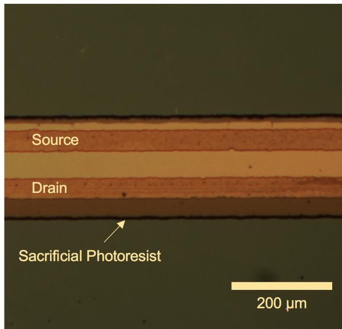
Figure 3.8. Micrograph of the device after patterning of 15  $\mu\text{m}$  thick sacrificial photoresist.
