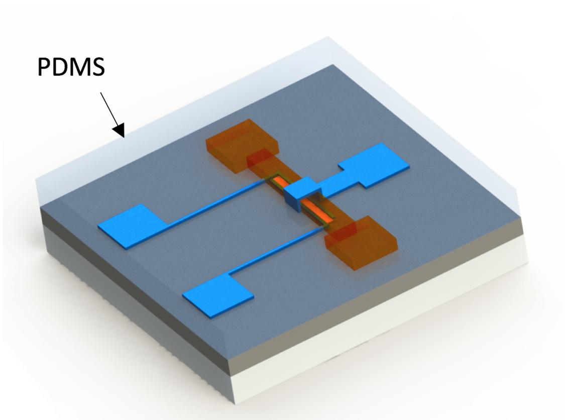
Figure 3.15. Device after 5 mm thick PDMS is casted.
