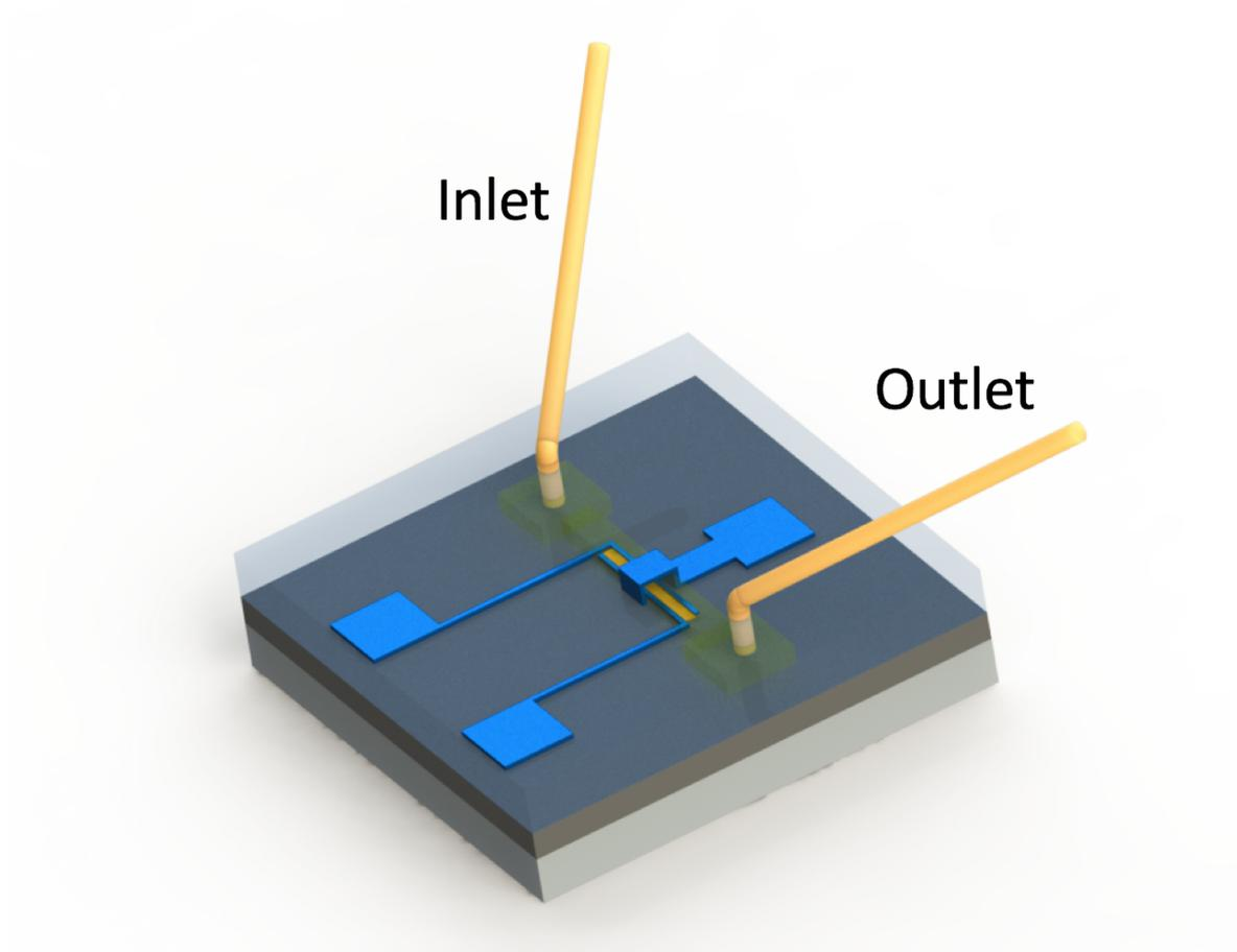
Figure 3.16. Device after reservoirs are opened and sacrificial photoresist is removed.
