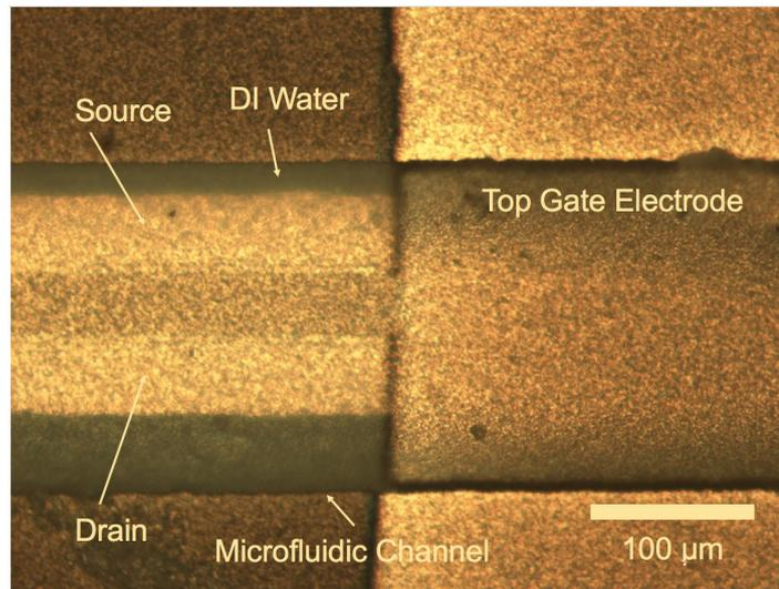
Figure 3.11. Micrograph of the device after 5  $\mu\text{m}$  parylene is deposited and microfluidic channel is released.
