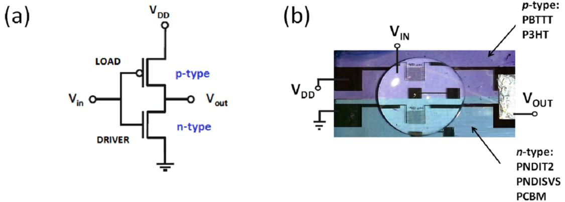
Figure 1.3. Integrated inverter with organic WG-FETs [17].
