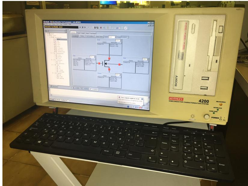
Figure 4.2. Keithley semiconductor characterization system.
