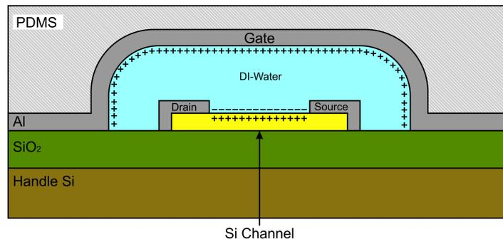
Figure 3.1. Cross-section sketch of the fabricated device.
