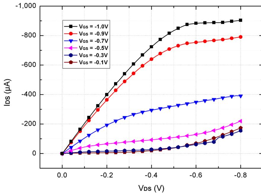
Figure 4.4.  $I_D$  vs  $V_{DS}$  characteristic of the device when gate width is  $1500 \mu m$ .
