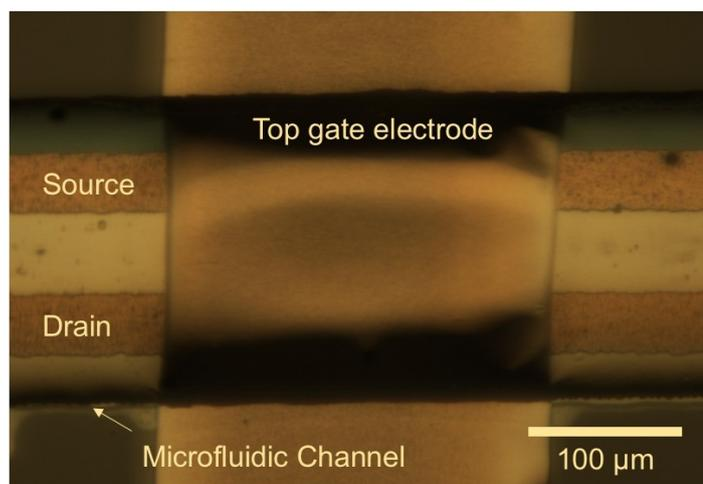
Figure 3.17. Micrograph of the device after PDMS microfluidic channel is released.
