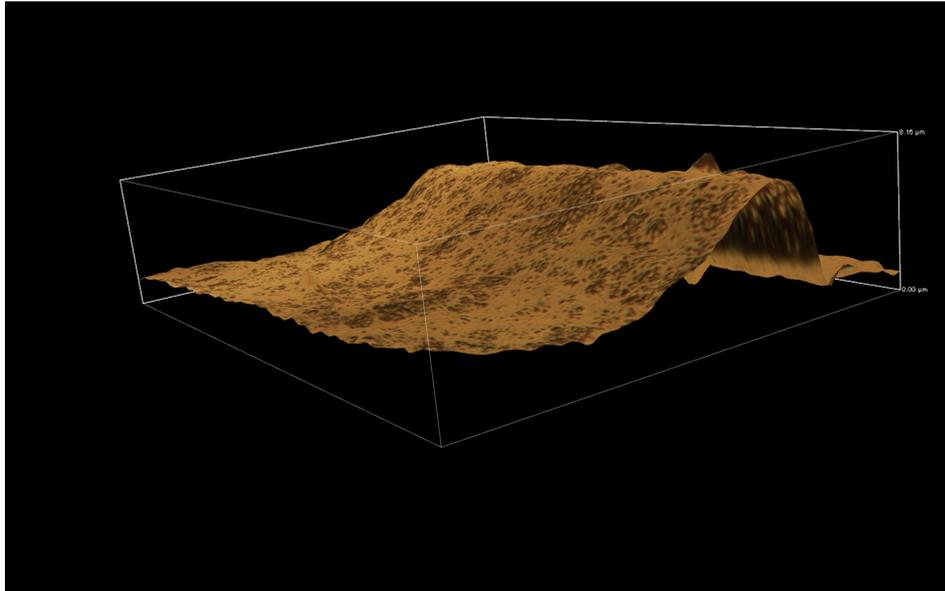
Figure 3.12. 3D micrograph of collapsed Al top gate.
