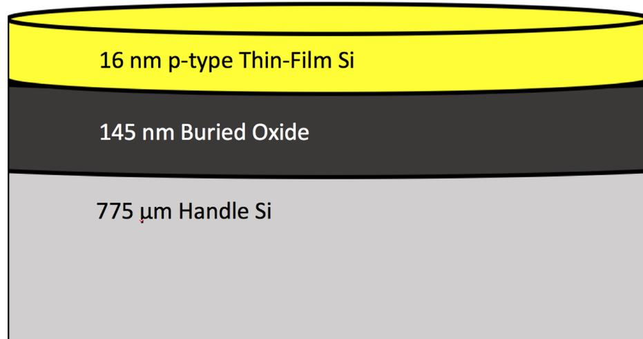
Figure 3.2. Sketch of SOI wafer.
