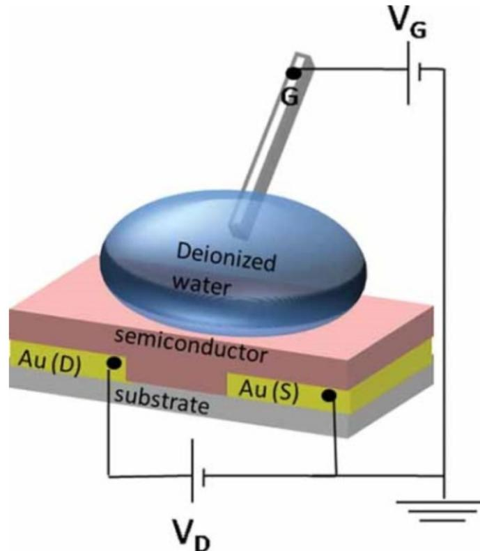
Figure 2.1. WG-FET with probe gate [15].
