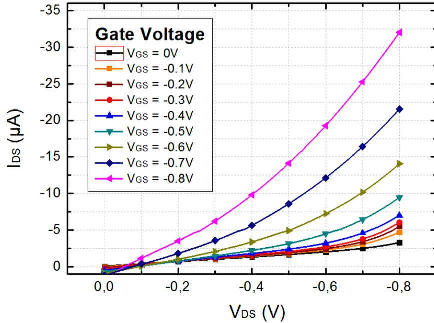
Figure 4.3.  $I_D$  vs  $V_{DS}$  characteristic of the device when gate width is  $300 \mu m$ .
