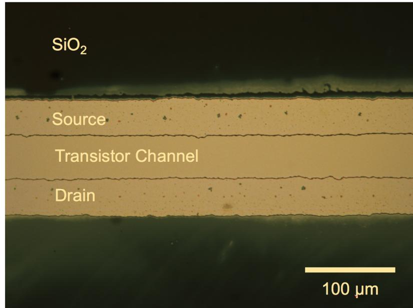
Figure 3.5. Micrograph of the device after Al patterning.
