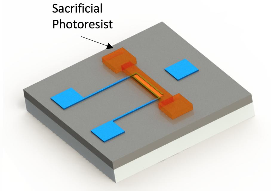
Figure 3.7. Device after patterning of  $15\ \mu\text{m}$  thick sacrificial photoresist.
