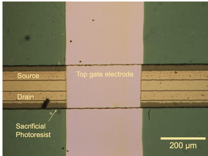
Figure 3.10. Micrograph of the device after 200 nm top gate Al is evaporated by shadow mask technique.
