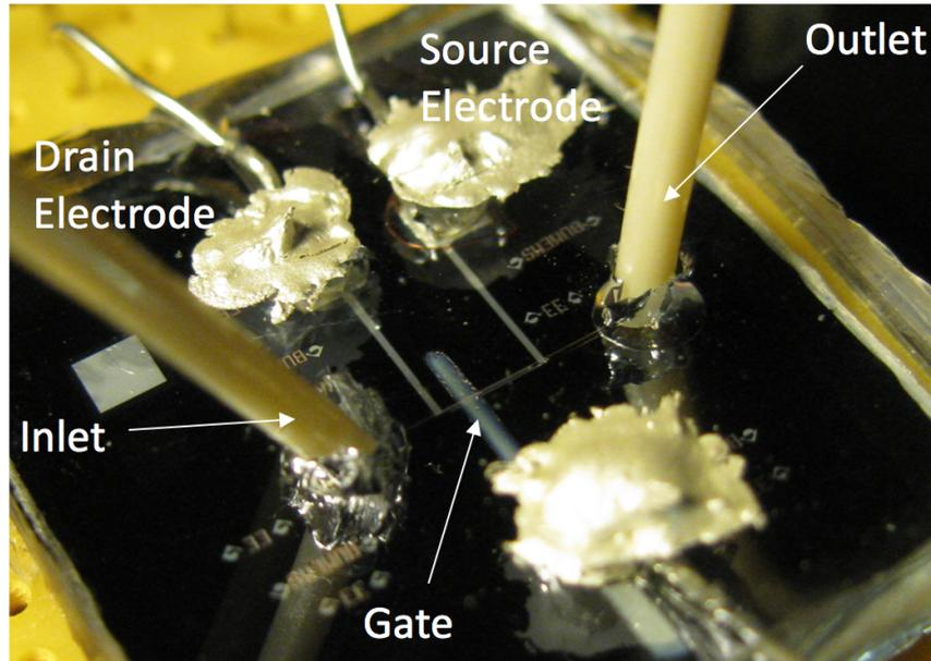
Figure 4.1. Test setup of the fabricated WG-FET device with external fluidic and electrical connections.
