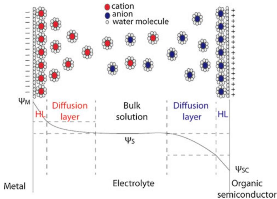
Figure 2.2. Representation of electrical double layer at the interfaces of semiconductor and gate electrode. [2]
