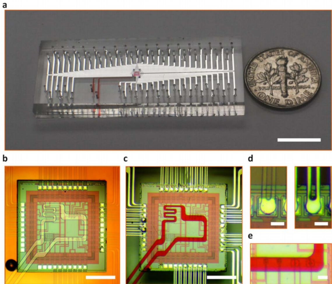
Figure 1.2. Microfluidic integrated CMOS hybrid chip with liquid interconnects. [11]
