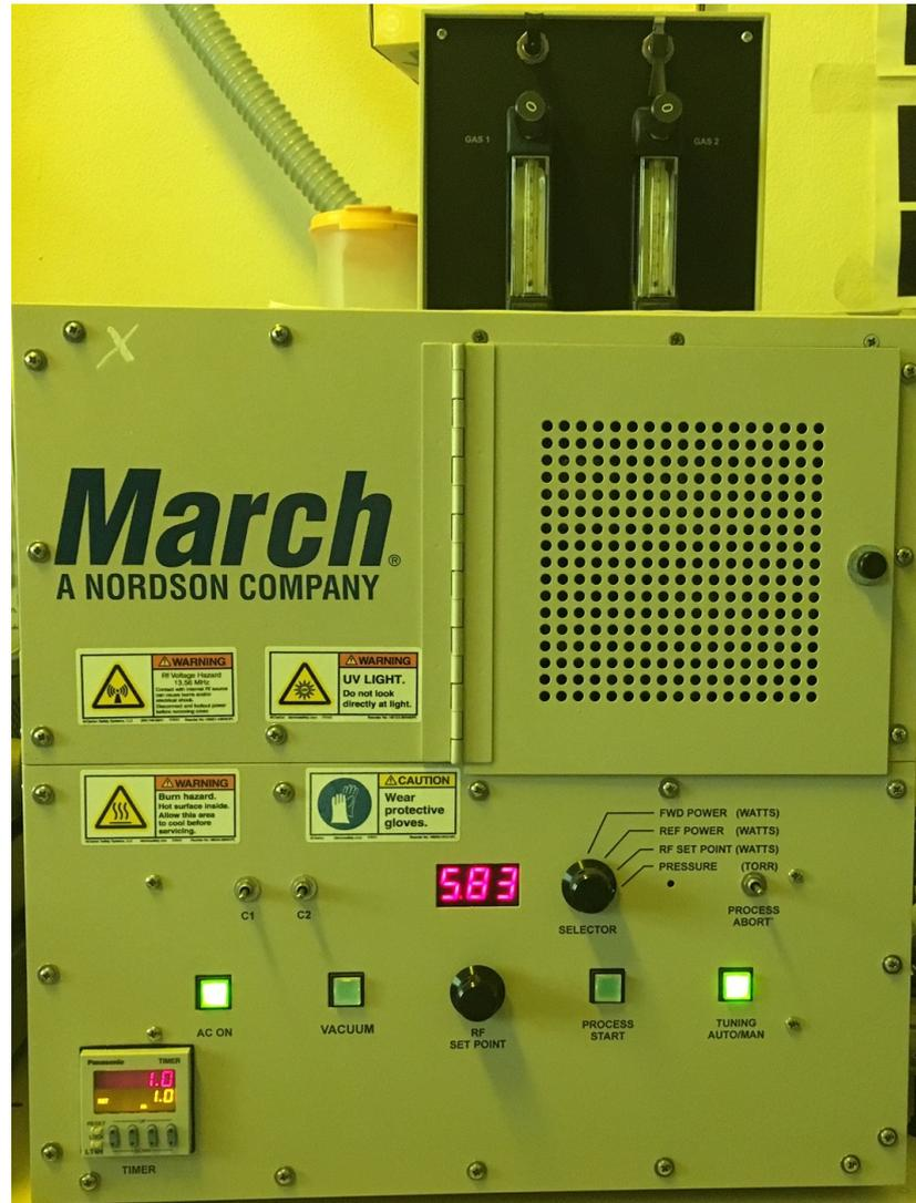
Figure 3.14. Oxygen plasma equipment.
