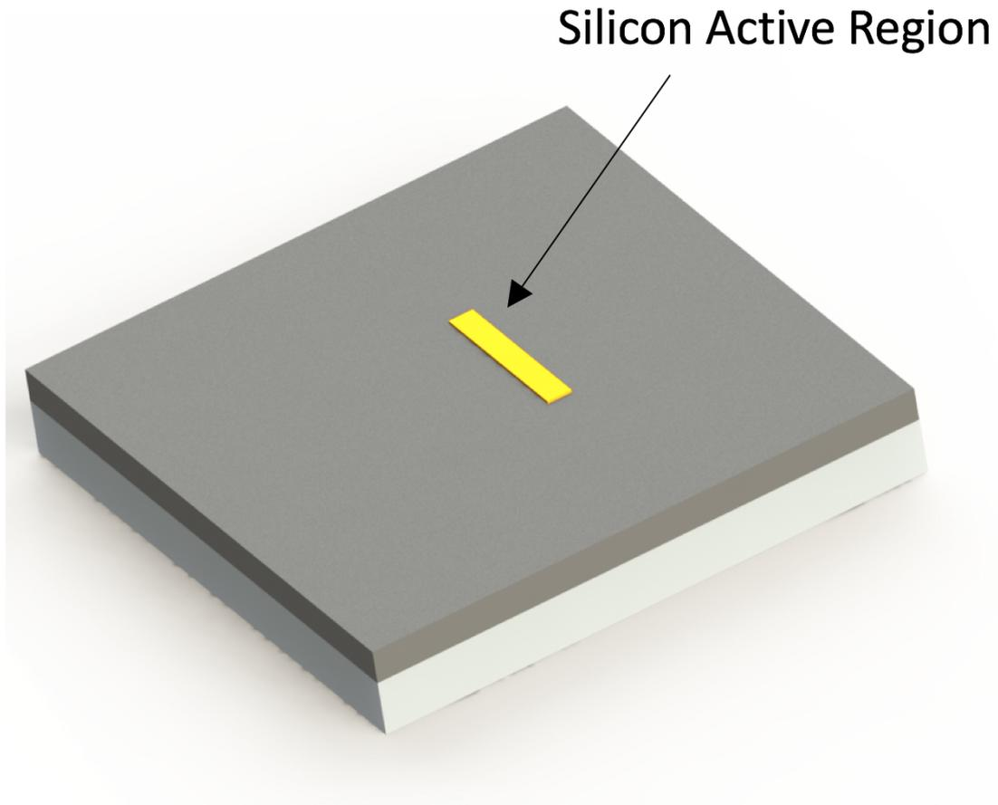
Figure 3.3. Device after patterning of 16 nm thick Si.
