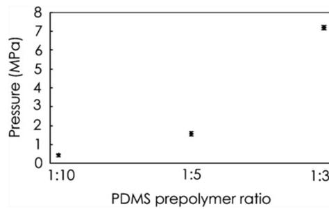
Figure 3.13. Comparison of bonding strengths of PDMS with respect to mixing ratios [27].
