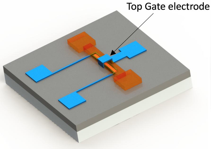
Figure 3.9. Device after 200 nm top gate Al is evaporated by shadow mask technique.
