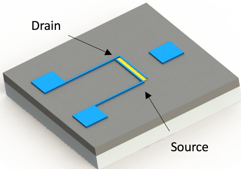
Figure 3.4. Device after patterning of 200 nm thick Al.
