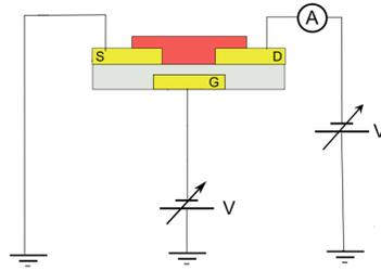
Figure 2.9. Measurement arrangement for DC characterization.
