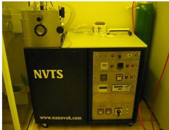
Figure 3.1. High vacuum thermal evaporator system.
