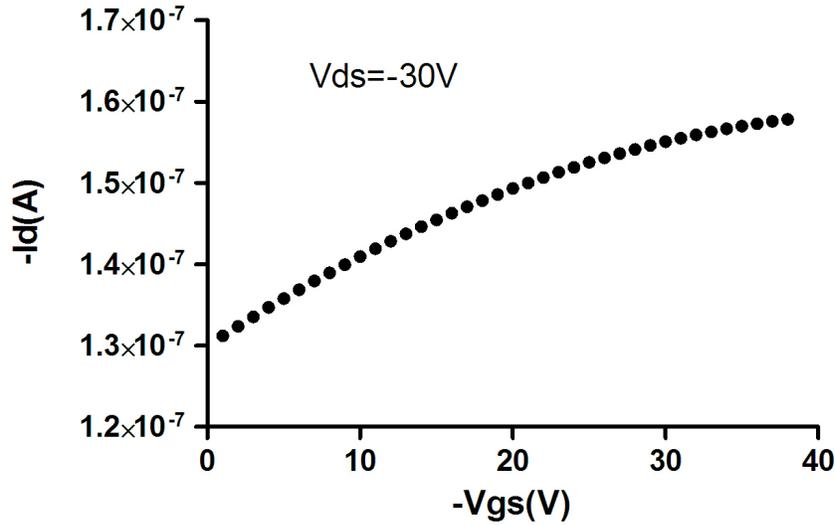
Figure 3.27. Transfer characteristic(interdigitated,  $L=50 \mu\text{m}$   $W=1000 \mu\text{m}$ ).
