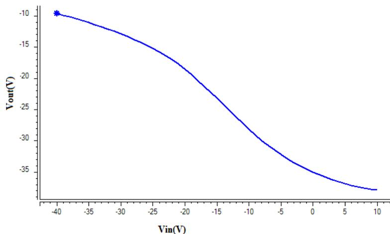
Figure 2.13. Transfer characteristic of zero- $V_{gs}$  load inverter.
