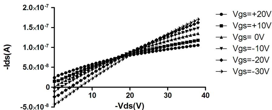
Figure 3.26. Output characteristic(interdigitated,  $L = 50 \mu\text{m}$   $W = 1000 \mu\text{m}$ ).
