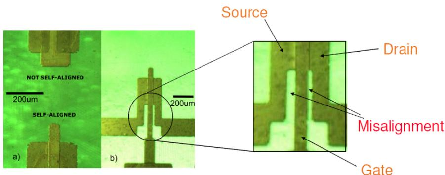
Figure 3.9. a) Picture of self-aligned and not self-aligned PTFTs b) Picture of a self-aligned PTFT alone.
