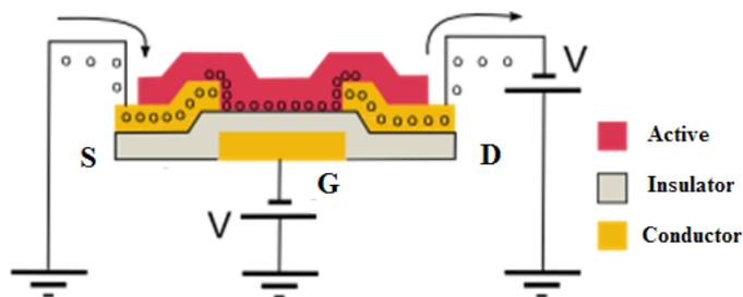
Figure 2.5. Representation of charge transport in a PTFT employing a p-type organic semiconductor.
