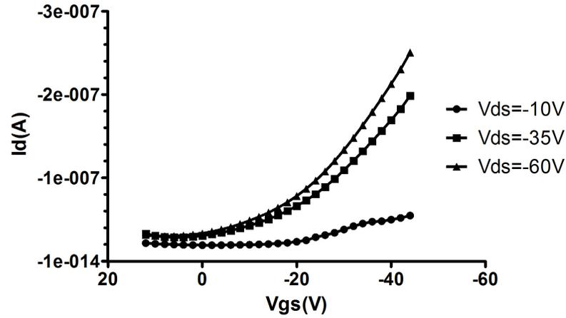
Figure 3.43. Transfer characteristics of PTFT with Ag drain/source ( $L = 200 \mu\text{m}$ ,  $W = 800 \mu\text{m}$ ).
