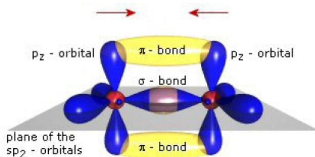
Figure 2.3. Bond structure between two carbon atoms( $sp^2$  hybridization).
