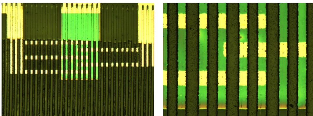
(a) Interdigitated transistor ( $L = 50 \mu\text{m}$ , $W = 1000 \mu\text{m}$ )
