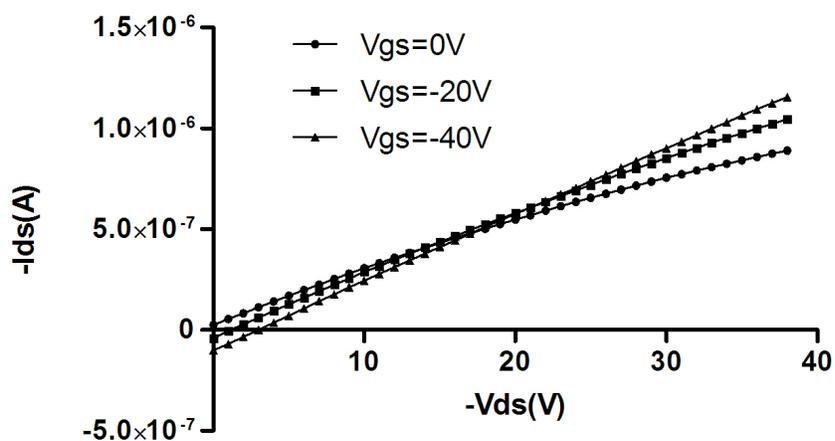
Figure 3.24. Output characteristic (interdigitated,  $L = 30 \mu\text{m}$   $W = 1000 \mu\text{m}$ ).
