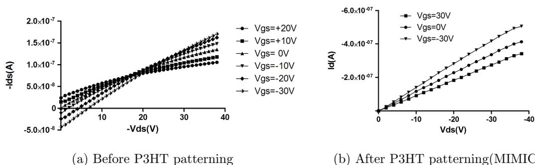
Figure 3.38. Output characteristics of an interdigitated PTFT before and after active layer patterning ( $L=50 \mu\text{m}$   $W=1000 \mu\text{m}$ ).
