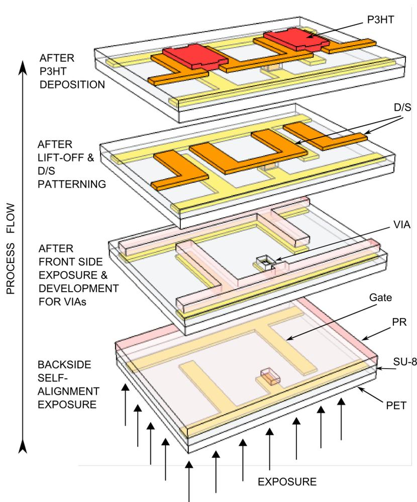
Figure 3.10. Process flow of a self-aligned PTFT
