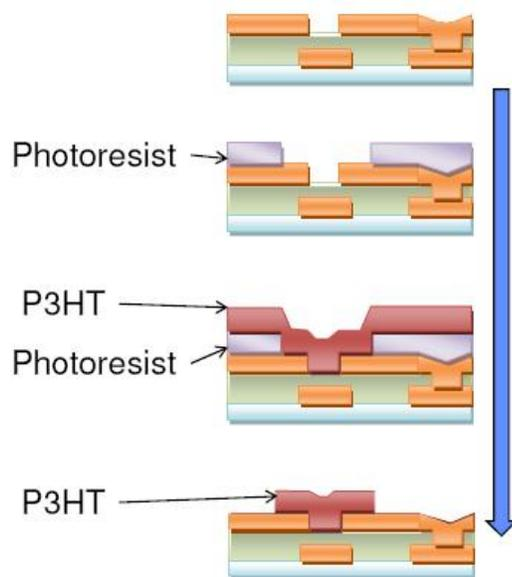
Figure 3.34. P3HT lift-off process flow.
