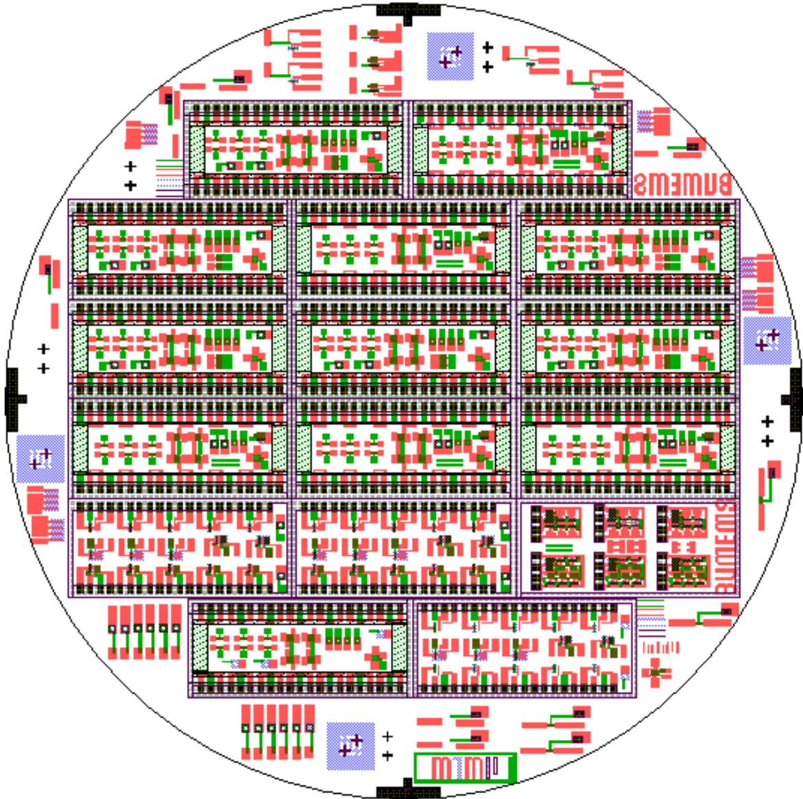
Figure A.1. Test layout containing various transistors, contact chains, Kelvin bridges, capacitors, invertors and ring-oscillators.
