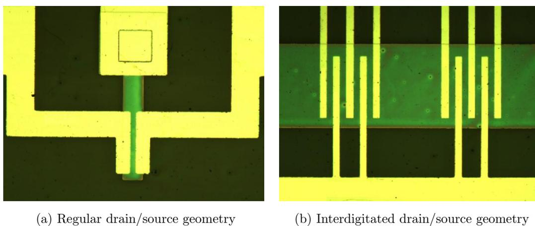
Figure 3.21. Transistors prior to the P3HT deposition.
