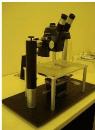
Figure 3.3. Custom made optical alignment setup.
