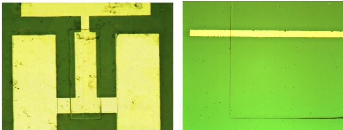
(a) Fully patterned transistor ( $L=50 \mu\text{m}$
