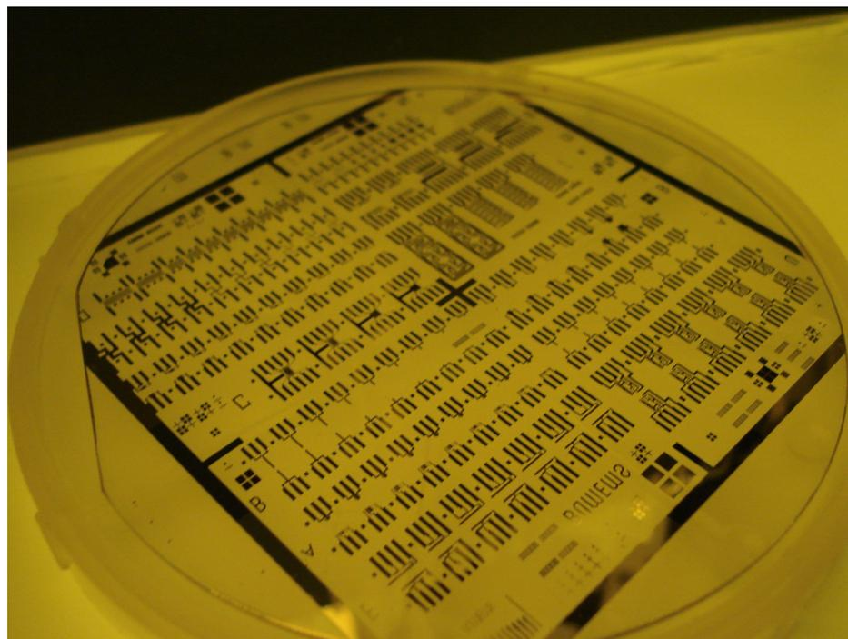
Figure 3.22. Completed four inch wafer prior to active layer deposition with patterned gate electrode, gate insulator and drain/source electrodes.
