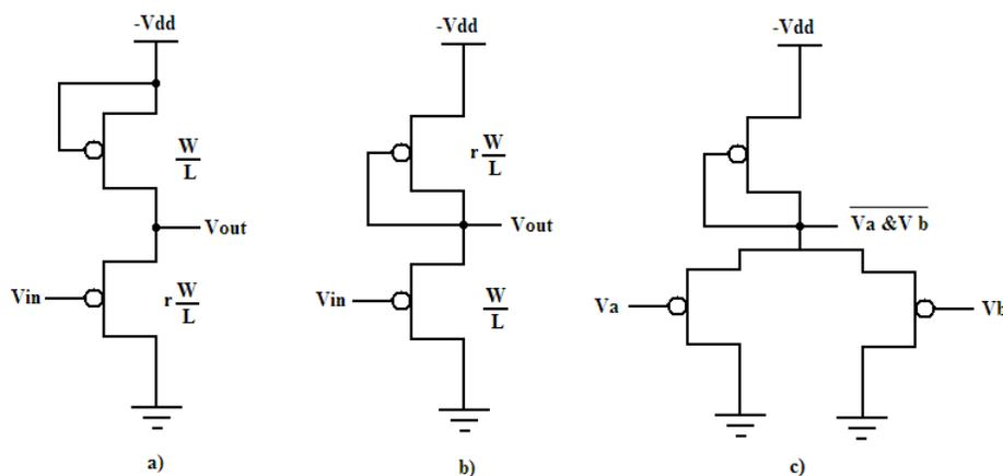
Figure 2.12. Inverters and NAND gate usually employed in digital PTFT circuits
