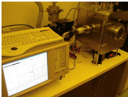
(b) Vacuum chamber and Keithley SCS 4200 semiconductor parameter analyzer
