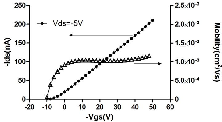
Figure 2.11. Simulated transfer characteristic in linear region and extracted mobility variation ( $C_i = 11 \text{ nF/cm}^2$ ,  $W = 2 \text{ mm}$ ,  $L = 30 \text{ }\mu\text{m}$ ).
