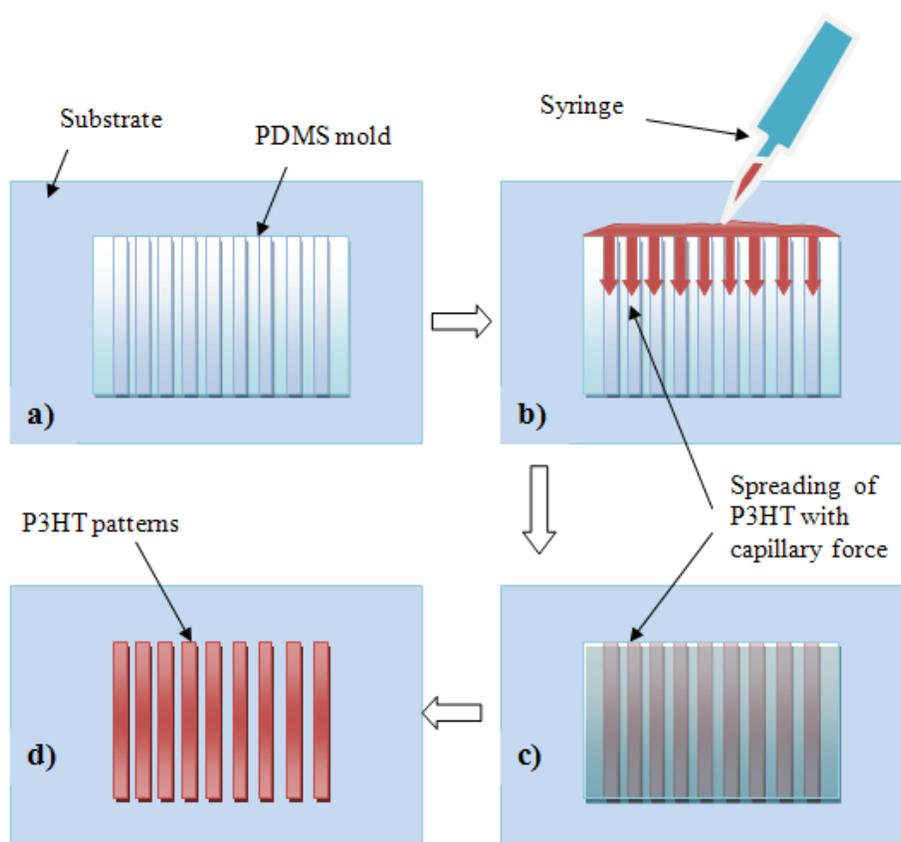
Figure 3.31. MIMIC process flow a)PDMS mold brought in contact with the substrate b)rr-P3HT in chlorobenzene is dispensed with a syringe c)capillary force drives the solution into the channels d)removal of the mold
