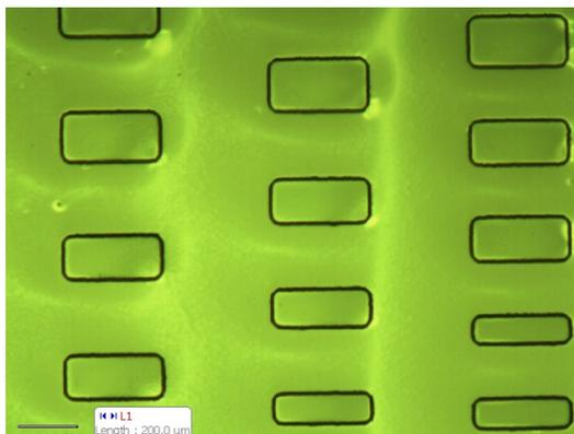
Figure 3.35. Spin-coated rr-P3HT from chlorobenzene solution (1 mg/ml).
