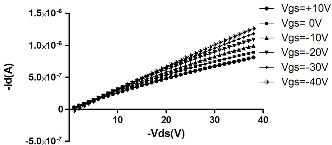
Figure 3.29. Output characteristic(Corbino,  $r_1=15 \mu\text{m}$   $r_2=18 \mu\text{m}$ ).
