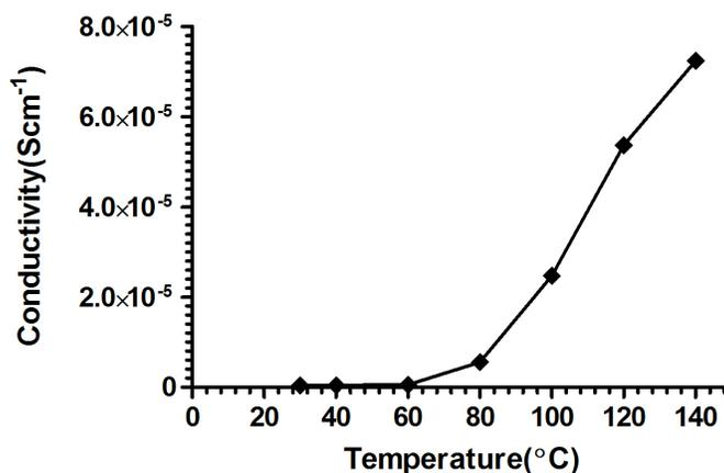
Figure 4.2. Variation of the conductivity with temperature.
