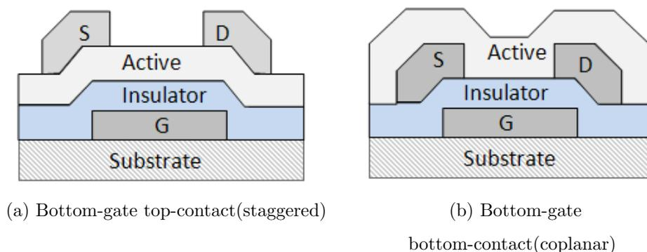
Figure 2.2. Bottom-gate(inverted) TFT topologies
