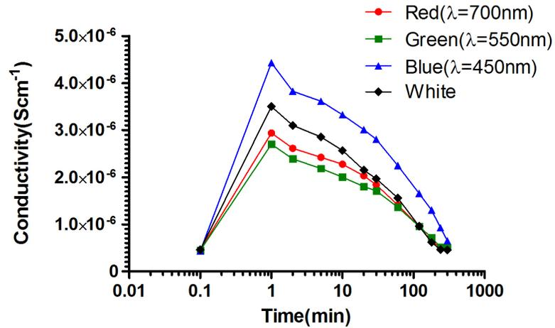
Figure 4.3. Variation of the conductivity with light exposure.
