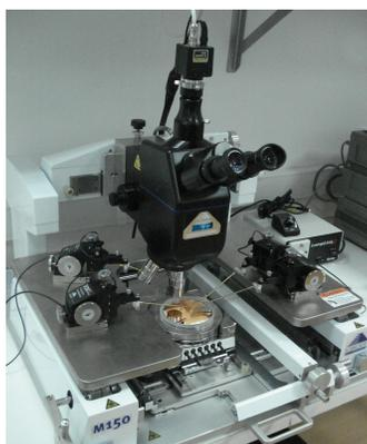
(a) Probe Station(Cascade Microtech M150)
