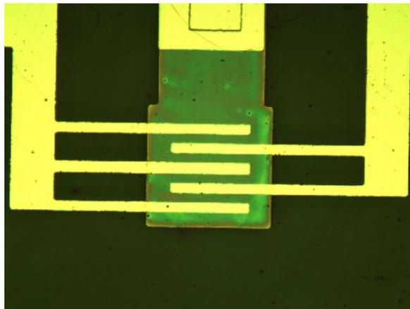
Figure 3.23. Interdigitated transistor ( $L = 50 \mu\text{m}$   $W = 1000 \mu\text{m}$ ).
