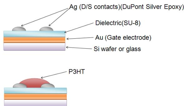
Figure 3.40. Cross-section of the PTFTs with Silver Epoxy Drain/Source Electrodes.
