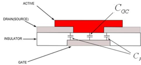
Figure 3.5. Cross-section of a TFT together with parasitic capacitors.
