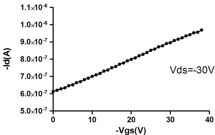
Figure 3.25. Transfer characteristic(interdigitated,  $L = 30 \mu\text{m}$   $W = 1000 \mu\text{m}$ ).
