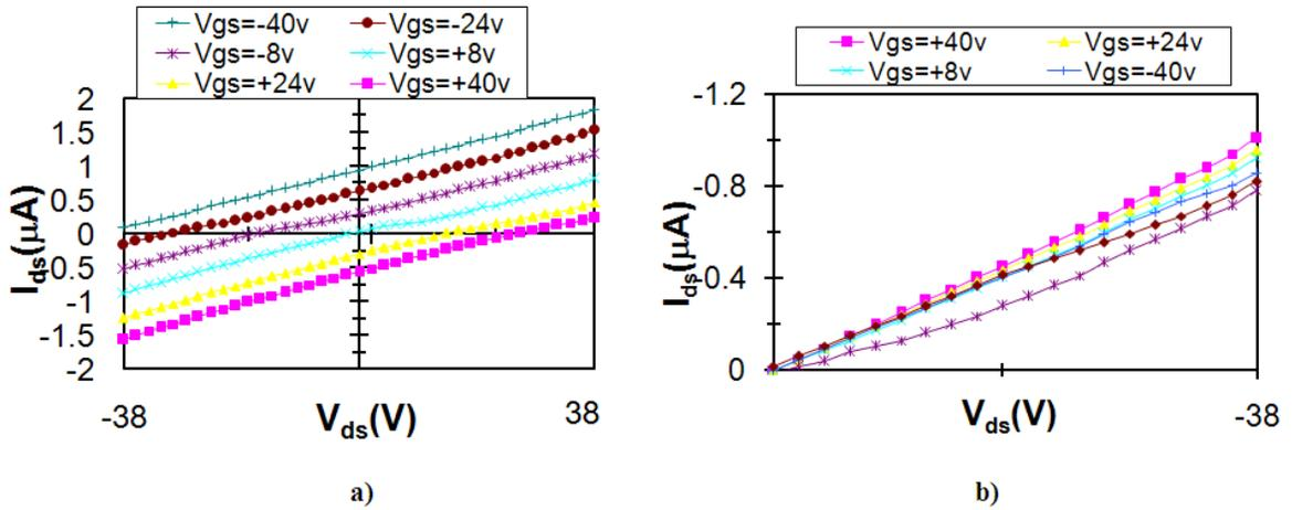
Figure 3.14. Measured output characteristics of a self-aligned transistor with defective gate insulator ( $L=50 \mu\text{m}$  and  $W=1000 \mu\text{m}$ ).
