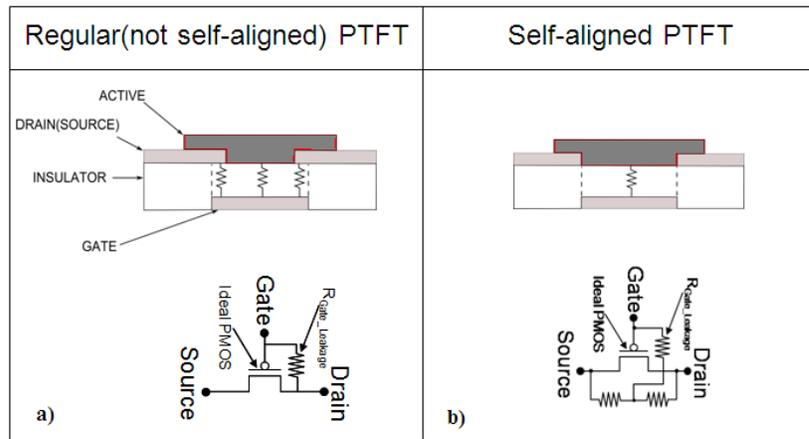
Figure 3.15. Device structures due to fabrication nonidealities.
