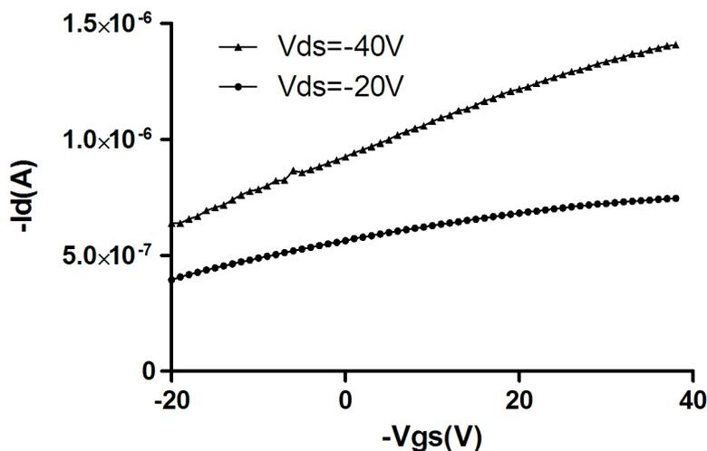
Figure 3.30. Transfer characteristic(Corbino,  $r_1=15 \mu\text{m}$   $r_2=18 \mu\text{m}$ ).
