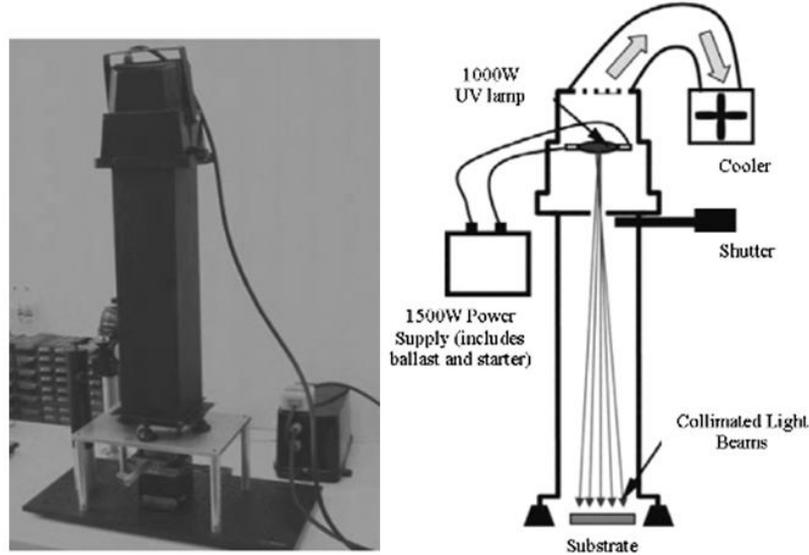
Figure 3.2. Custom made UV exposure system.
