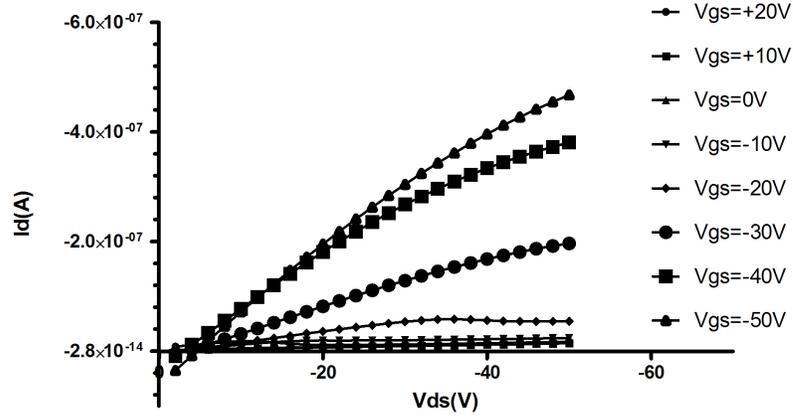
Figure 3.42. Output characteristics of PTFT with Ag drain/source ( $L = 200 \mu\text{m}$ ,  $W = 800 \mu\text{m}$ ).
