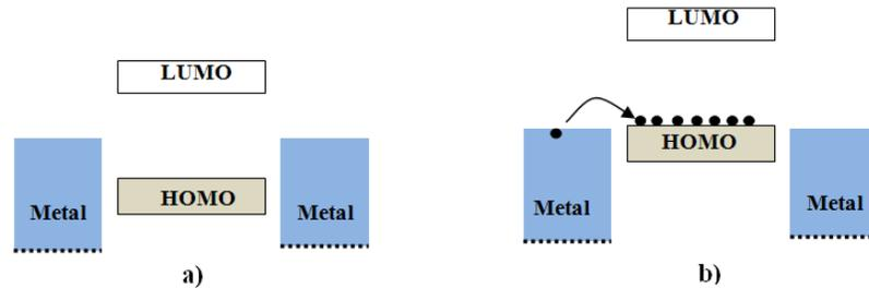
Figure 2.6. Representation of a working principle of a p-type OTFT a)no charges are accumulated when  $V_{GS} = 0V$  b)when a negative voltage applied to the gate.
