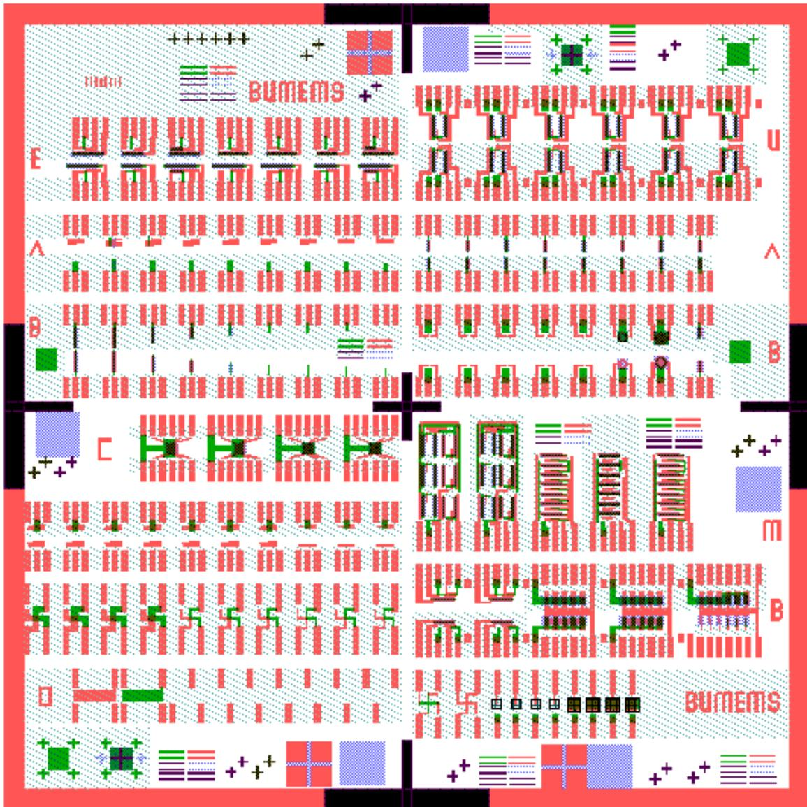
Figure 3.6. Layout of the test structures fabricated with self-aligned process.
