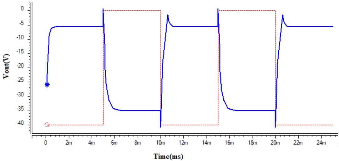
Figure 2.14. Transient output voltage waveform of a zero- $V_{gs}$  load inverter with square-wave input voltage.
