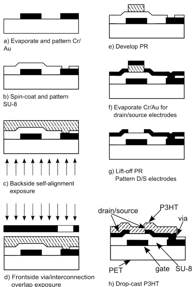
Figure 3.7. Process flow of a self-aligned PTFT
