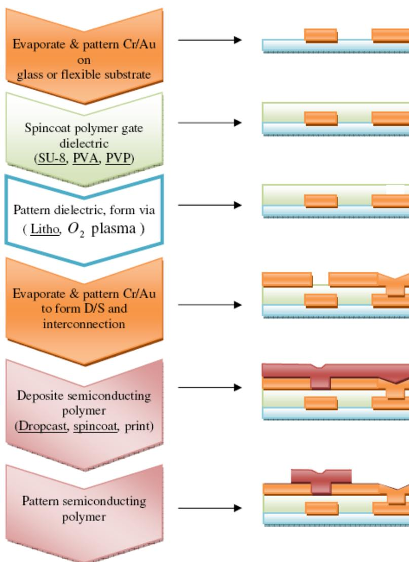
Figure 3.16. Process flow of the bottom-gate bottom contact transistors.
