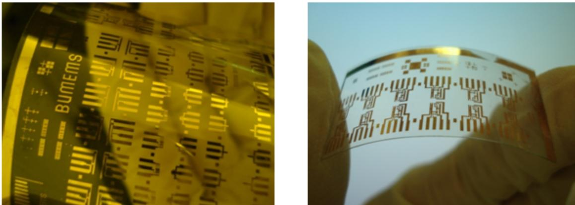
Figure 3.11. a) Picture of self-aligned and not self-aligned PTFTs on flexible substrate. b) PTFT circuits on flexible substrate.
