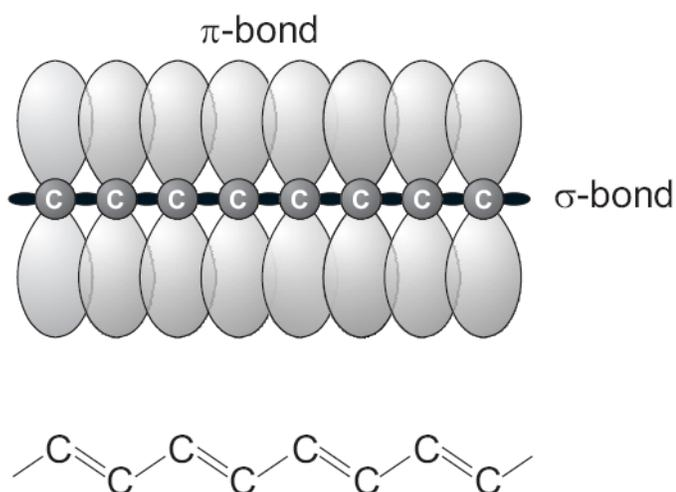
Figure 2.4. Representation of the sigma( $\sigma$ ) and pi( $\pi$ ) bonds between carbon atoms (above) in polyacetylene (below).
