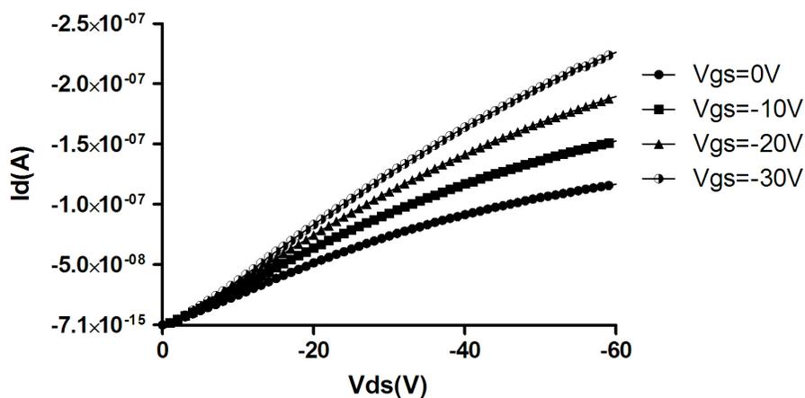
Figure 3.39. Output curves of the fully patterned transistor (Lift-off,  $L=50 \mu\text{m}$   $W=1000 \mu\text{m}$ ).
