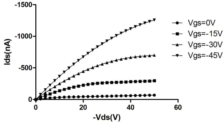
Figure 2.10. Simulated output characteristics ( $C_i = 11 \text{ nF/cm}^2$ ,  $W = 2 \text{ mm}$ ,  $L = 30 \text{ }\mu\text{m}$ ).
