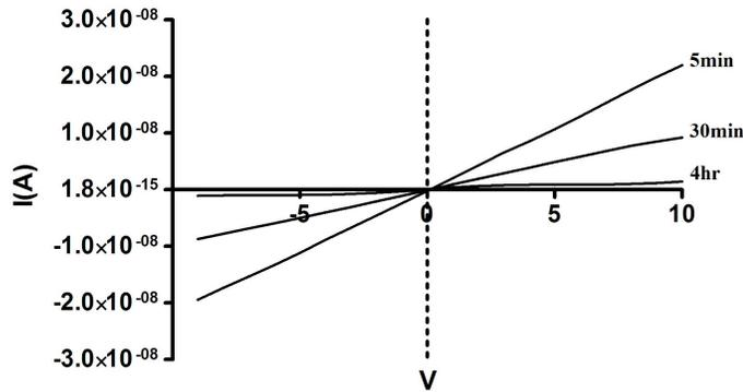
Figure 3.41. I-V sweeps of rr-P3HT film between lateral Ag electrodes as time progresses in vacuum.
