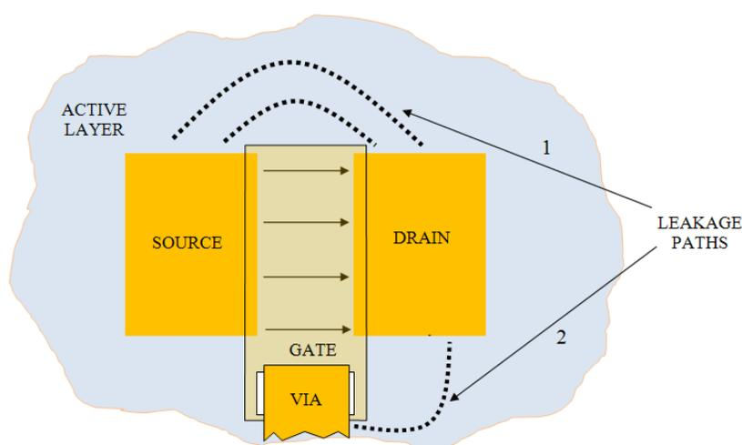
Figure 3.37. Leakage paths due to un-patterned active layer.
