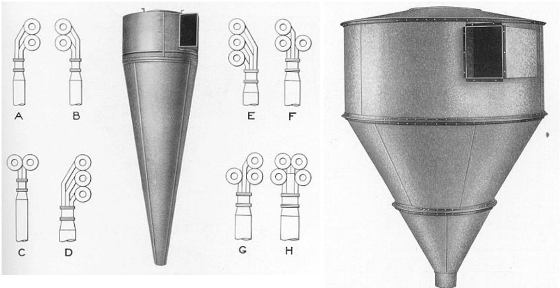
Figure 1.3. Flour mill multi-cyclones manufactured in 1922 by Wolf company [1].
