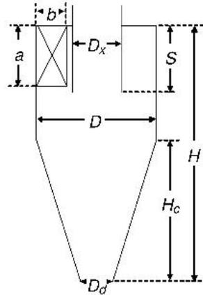
Figure 1.9. The geometrical sizes of cyclone separator.
