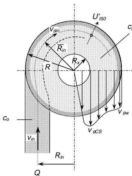
Figure 2.2. Upper section of conventional cone type cyclone with further more information about velocities and dimensions [1].
