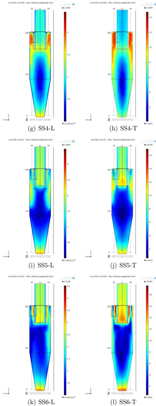
Figure 3.27. Double slot inputs-SS MODELS-Velocity profile in laminar(L) & turbulent(T) solvers (g-l).
