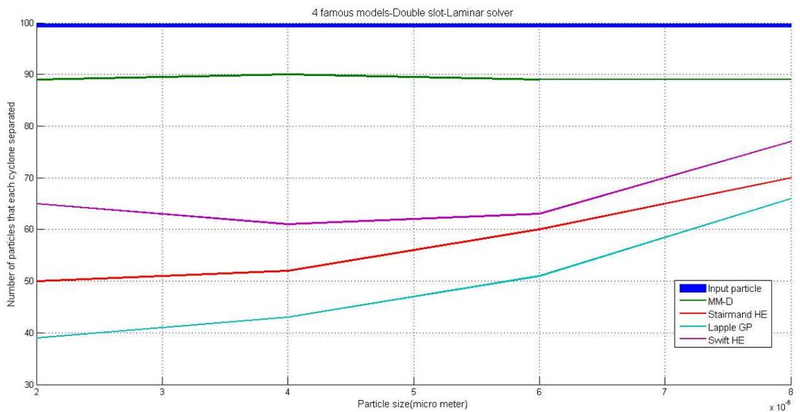
Figure 3.8. Famous models-Double slot-with low input velocity.
