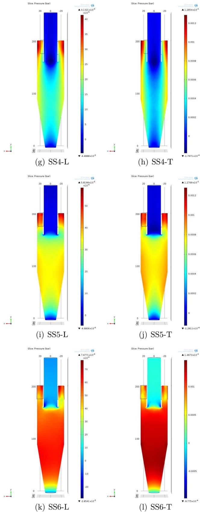
Figure 3.21. Double slot inputs-SS MODELS-Pressure profile in laminar(L) & turbulent(T) solvers (g-l).
