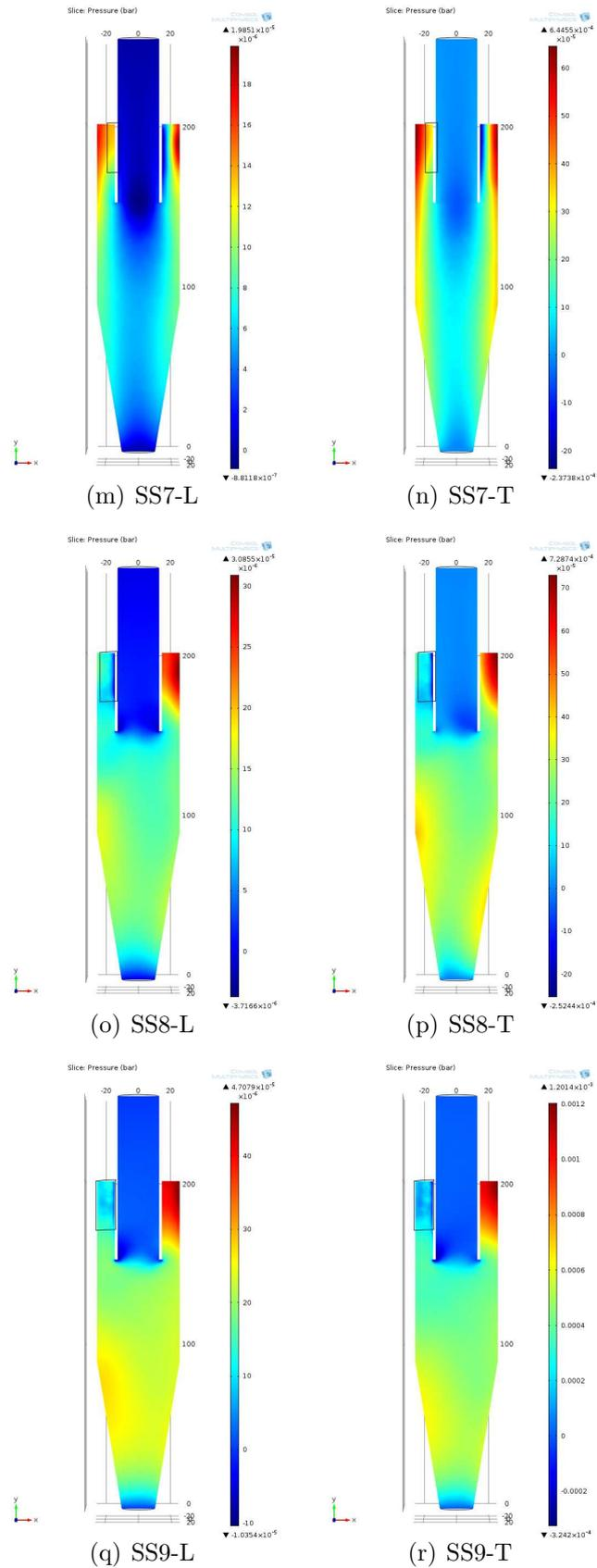
Figure 3.19. Single slot input-SS MODELS-Pressure profile in laminar(L) & turbulent(T) solvers (m-r).
