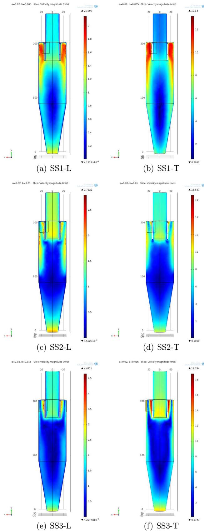
Figure 3.26. Double slot inputs-SS MODELS-Velocity profile in laminar(L) & turbulent(T) solvers (a-f).
