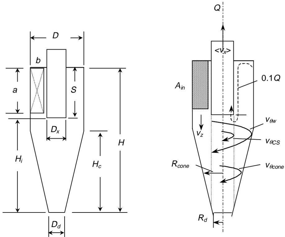
Figure 2.1. Dimensional notation and placements of velocities inside the ordinary cyclone with cone type [1].
