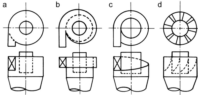
Figure 1.10. Side and top views of the four well-known inlet configurations. a 'slot' (also called 'tangential') inlet, b 'wrap-around' inlet, c 'helical roof' inlet and d axial inlet with swirl vanes [1].
