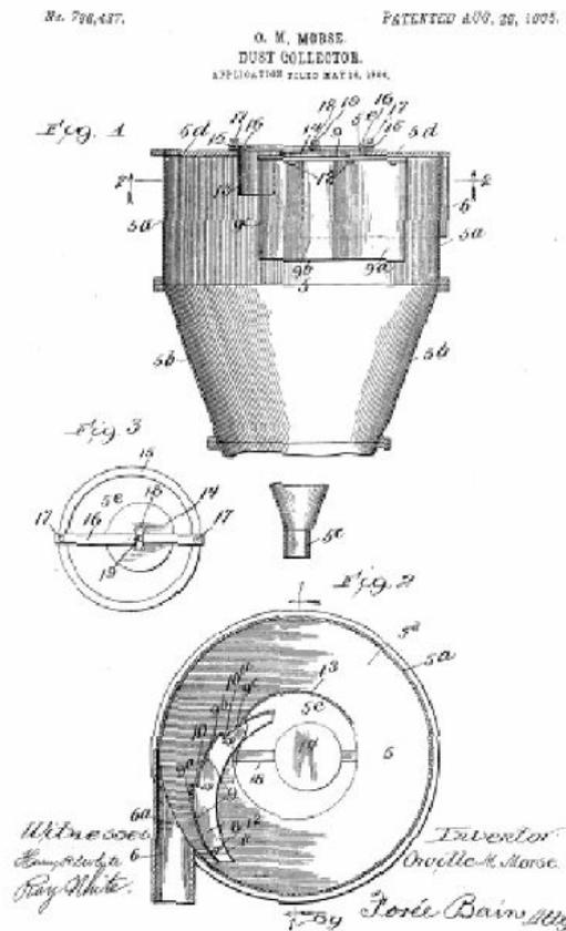
Figure 1.2. A basic patent of cyclone with conical section in bottom apex [1].
