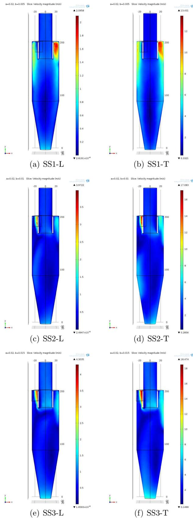
Figure 3.23. Single slot input-SS MODELS-Velocity profile in laminar(L) & turbulent(T) solvers (a-f).
