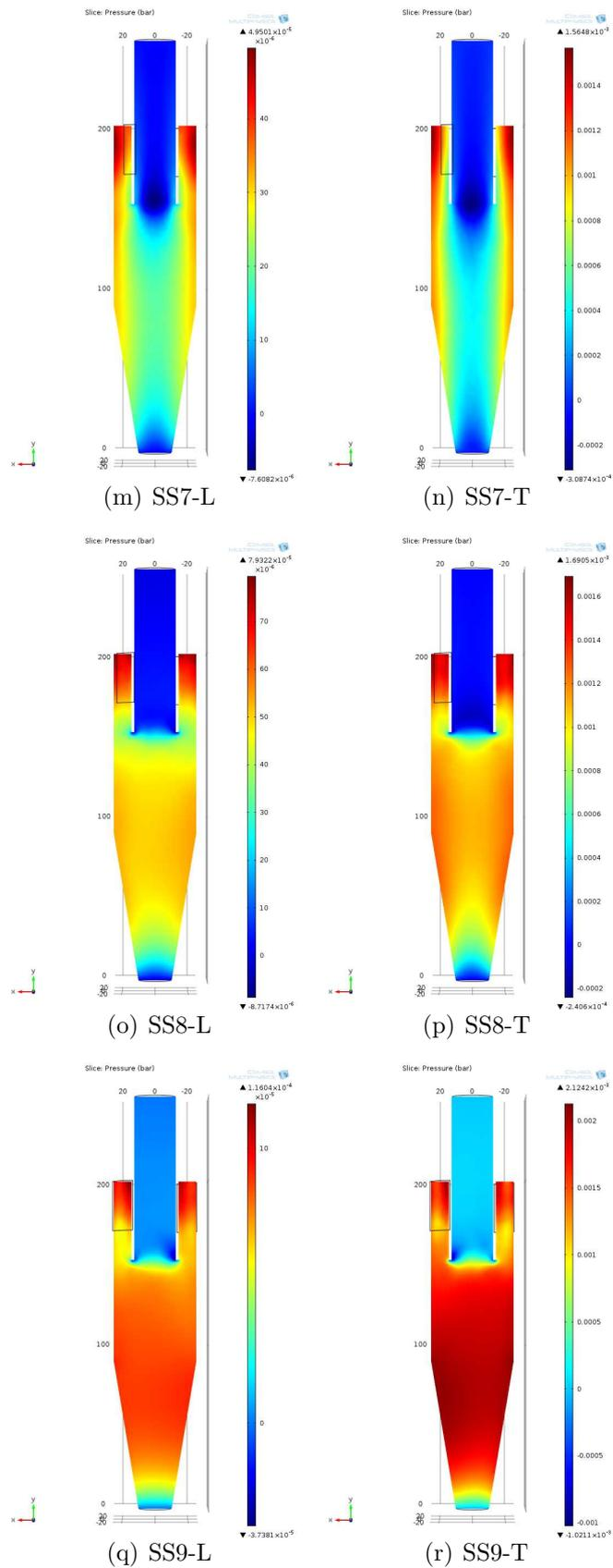
Figure 3.22. Double slot inputs-SS MODELS-Pressure profile in laminar(L) & turbulent(T) solvers (m-r).
