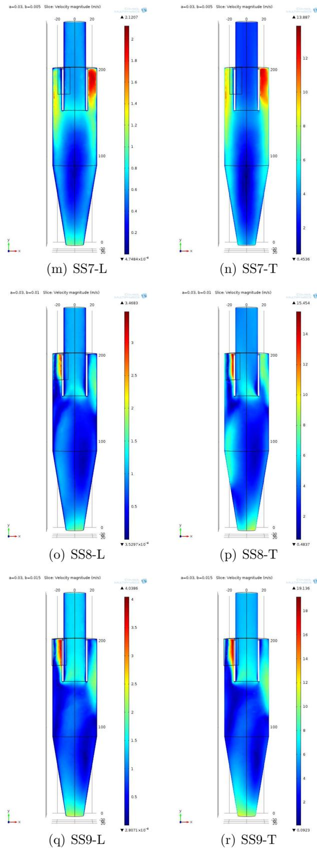
Figure 3.25. Single slot input-SS MODELS-Velocity profile in laminar(L) & turbulent(T) solvers (m-r).
