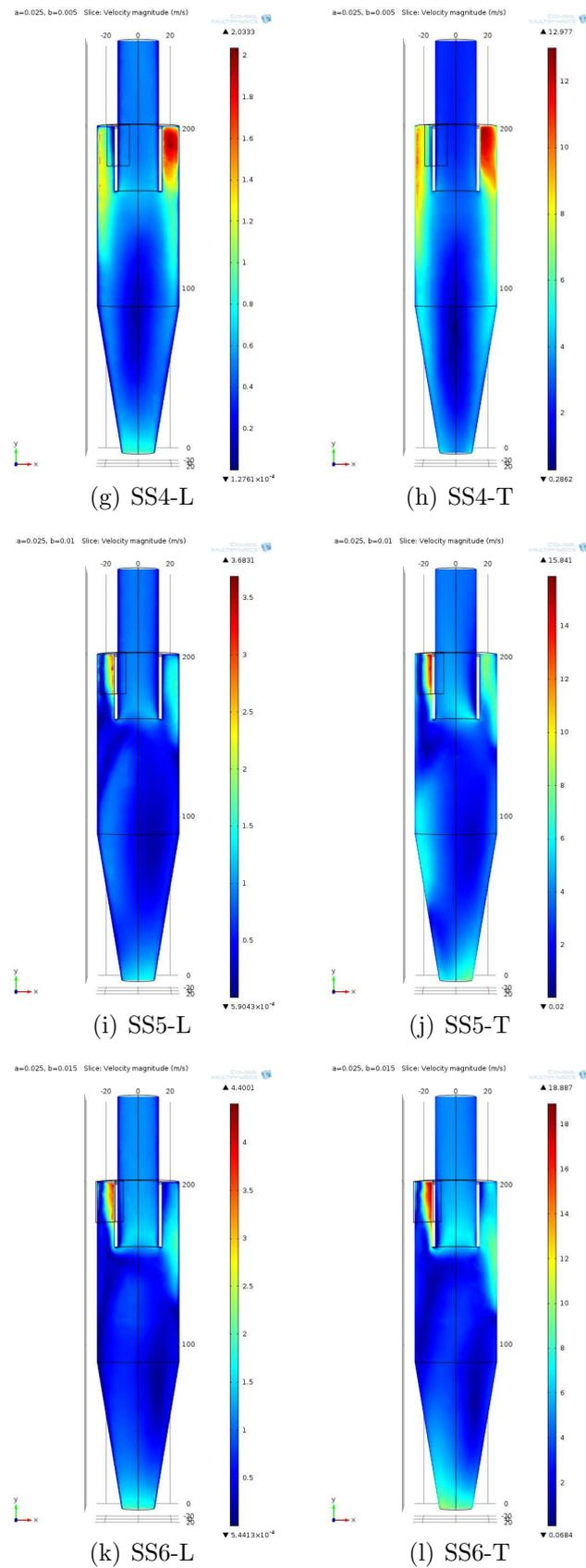
Figure 3.24. Single slot input-SS MODELS-Velocity profile in laminar(L) & turbulent(T) solvers (g-l).
