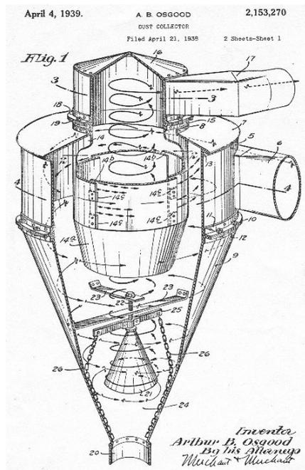
Figure 1.4. Another patent of a cyclone that designed by Osgood in 1939 [1].
