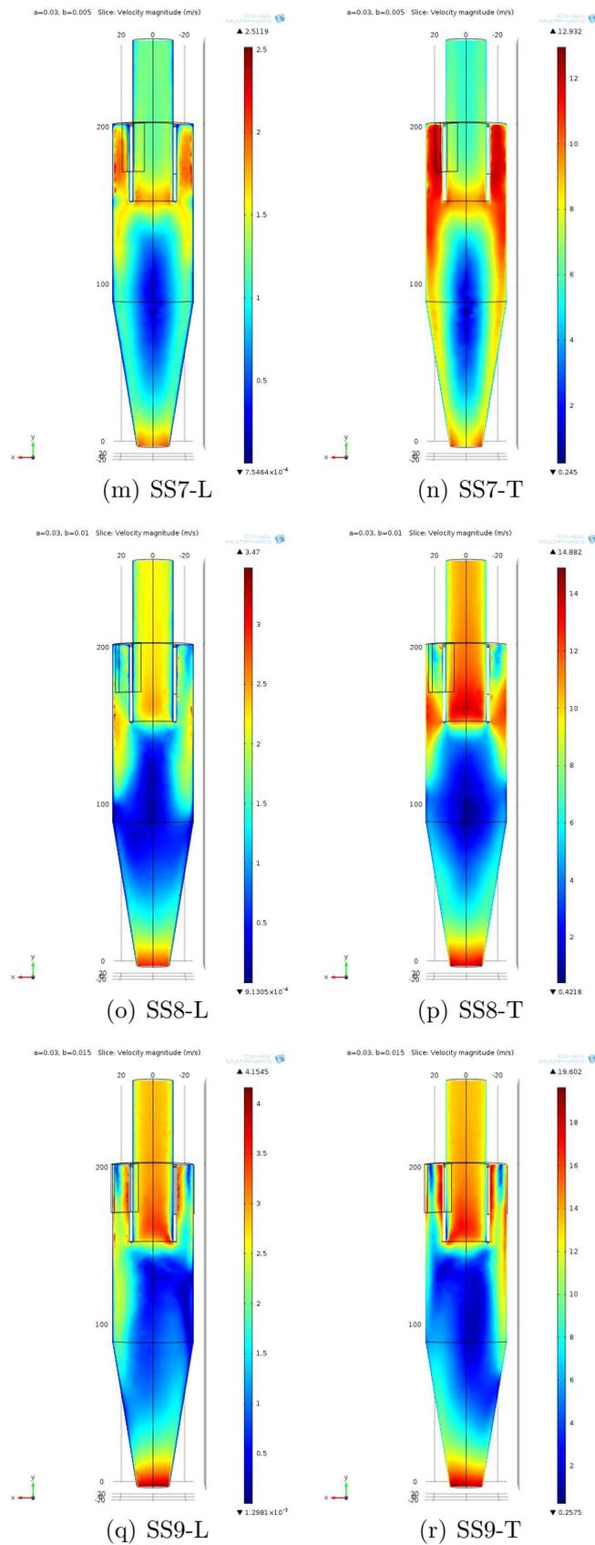
Figure 3.28. Double slot inputs-SS MODELS-Velocity profile in laminar(L) & turbulent(T) solvers (m-r).
