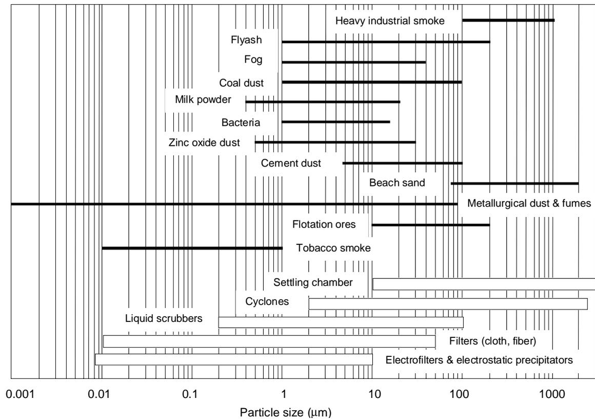
Figure 1.7. Particle size of some materials and recommended methods for removing them from a gas stream [1].
