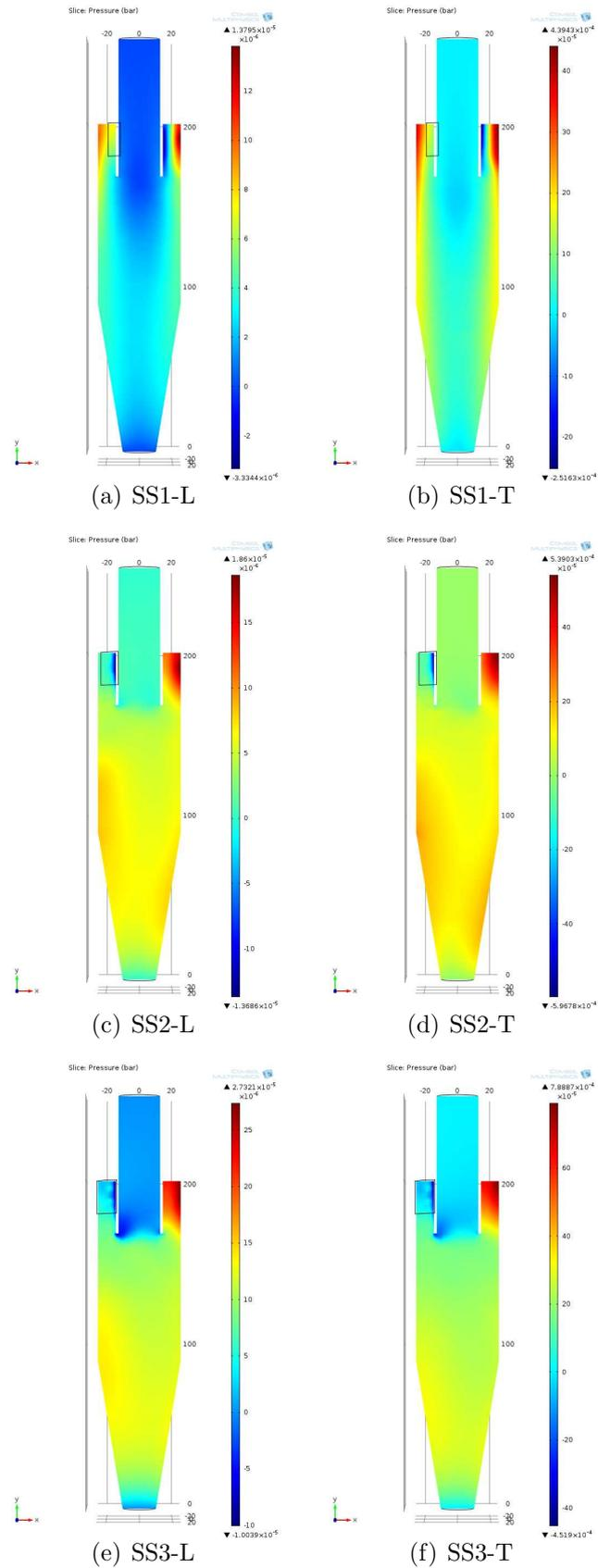
Figure 3.17. Single slot input-SS MODELS-Pressure profile in laminar(L) & turbulent(T) solvers (a-f).
