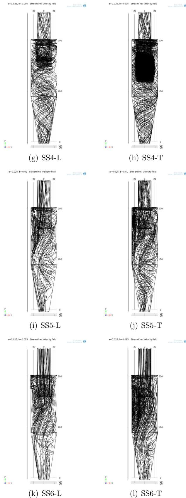
Figure 3.12. Single slot input-SS MODELS-Streamlines in laminar(L) & turbulent(T) solvers (g-l).
