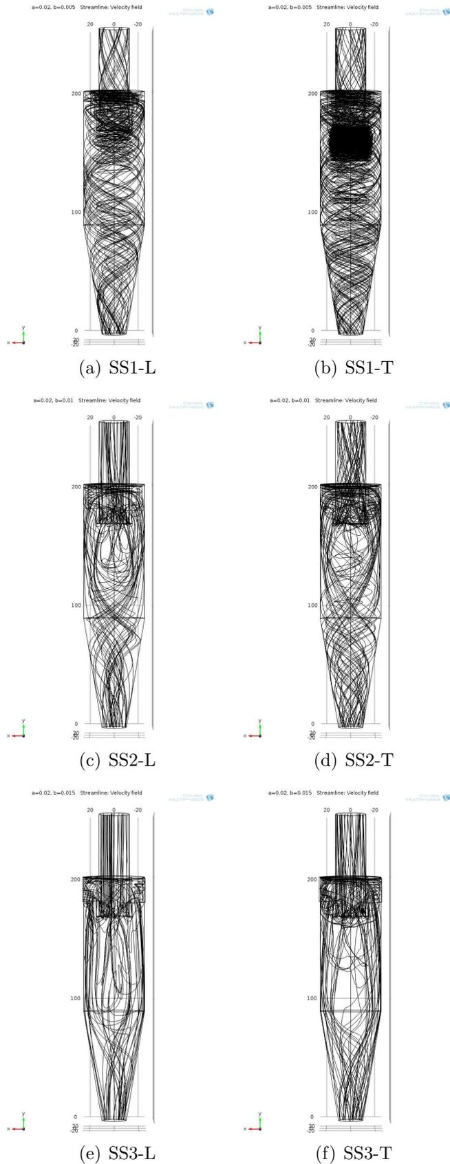
Figure 3.14. Double slot inputs-SS MODELS-Streamlines in laminar(L) & turbulent(T) solvers (a-f).
