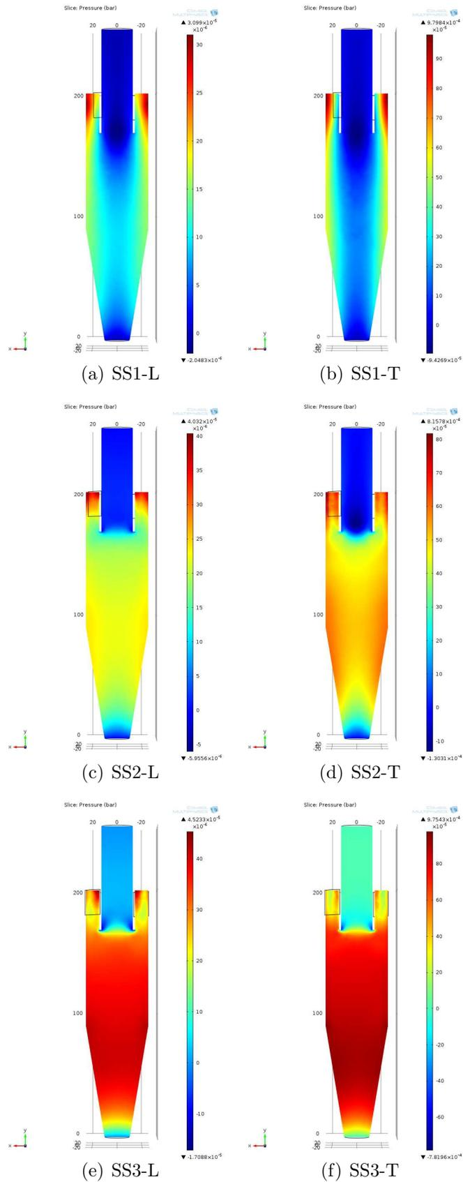
Figure 3.20. Double slot inputs-SS MODELS-Pressure profile in laminar(L) & turbulent(T) solvers (a-f).
