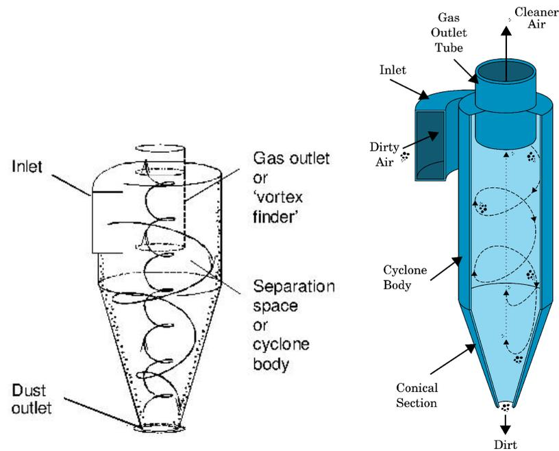
Figure 1.8. Sketch of a reverse flow and conical type cyclone with a tangential slot type inlet [1].
