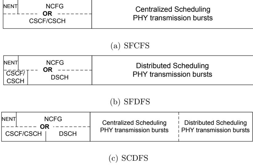
Figure 2.8. Mesh frame structure types according to the scheduling methods
