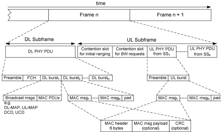
Figure 2.3. PMP mode OFDM frame structure using TDD [3]
