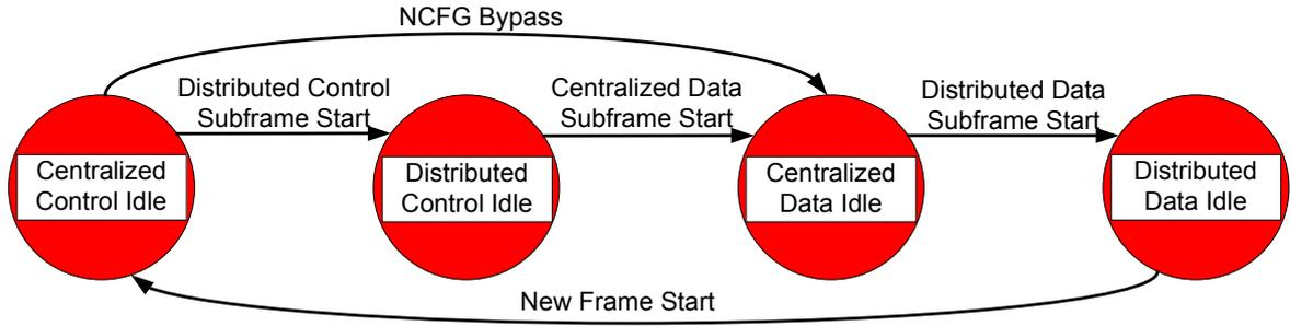
Figure 5.3. NEMMS frame cycle state diagram
