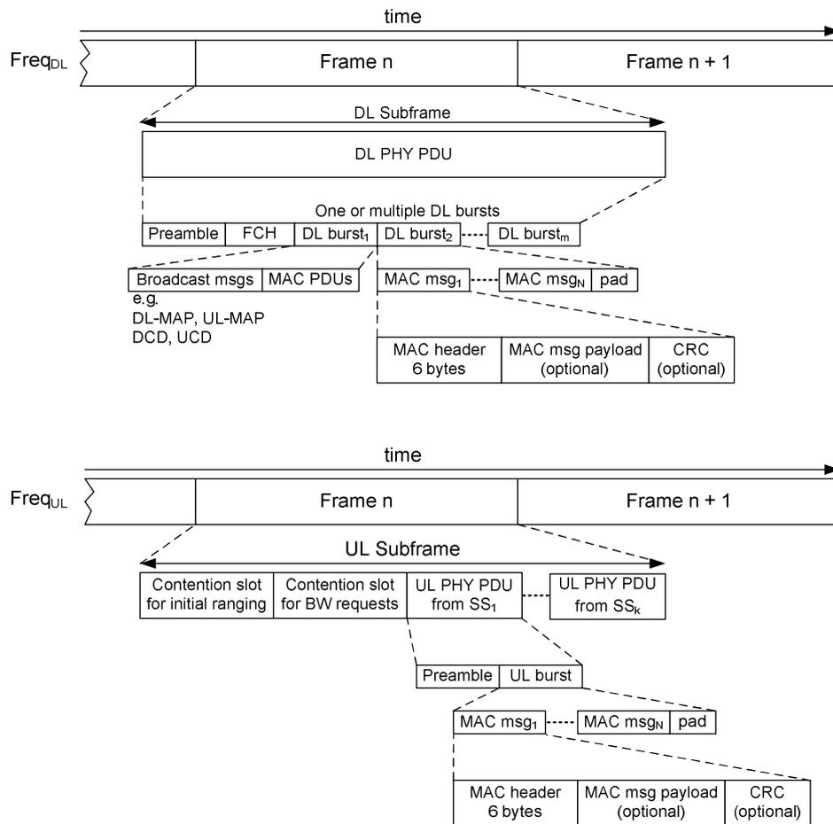
Figure 2.4. PMP mode OFDM frame structure using FDD [3]
