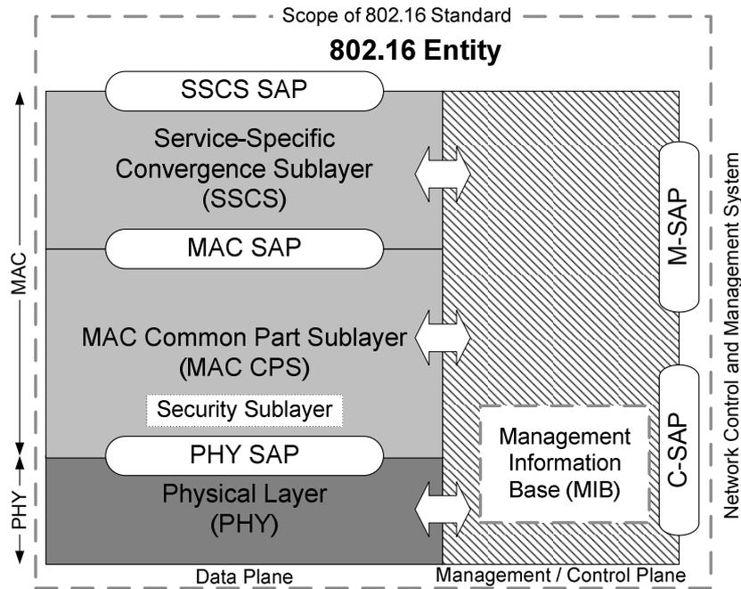
Figure 2.1. Reference model and scope of WiMAX standard [7]
