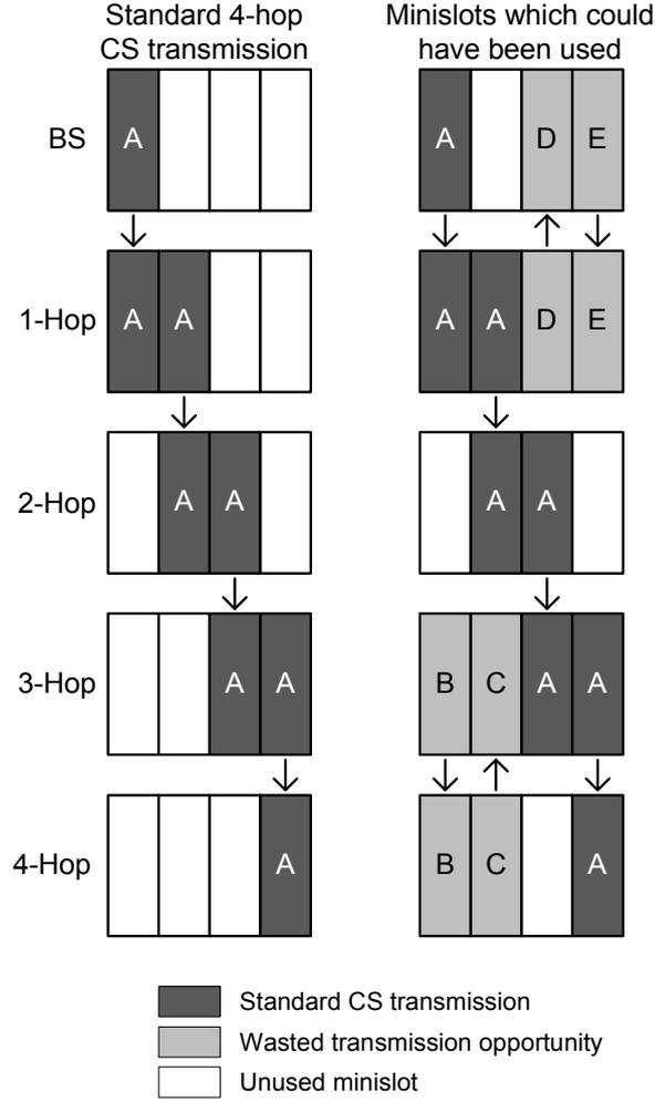
Figure 4.1. Wasted minislots during a standard CS transmission
