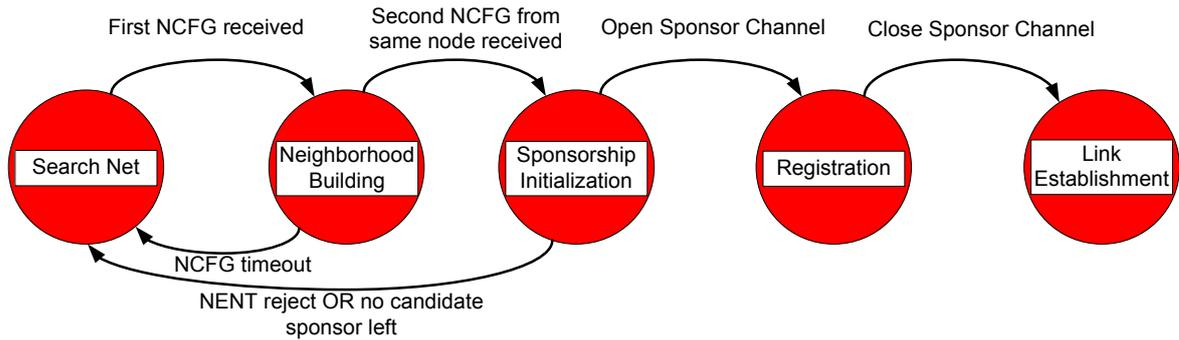
Figure 5.1. Initialization procedure simplified state diagram
